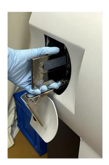
**Fig. S6.**The present chip inserted in to MALDI-TOFMS mounted on an adapter (P/N 8235380, Bruker Japan K.K.).
