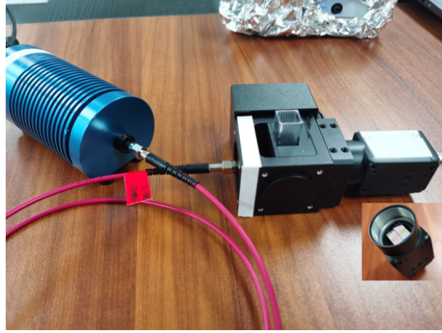
Figure S2 The four-channel spectral sensor acquisition system for detecting wine adulteration.
