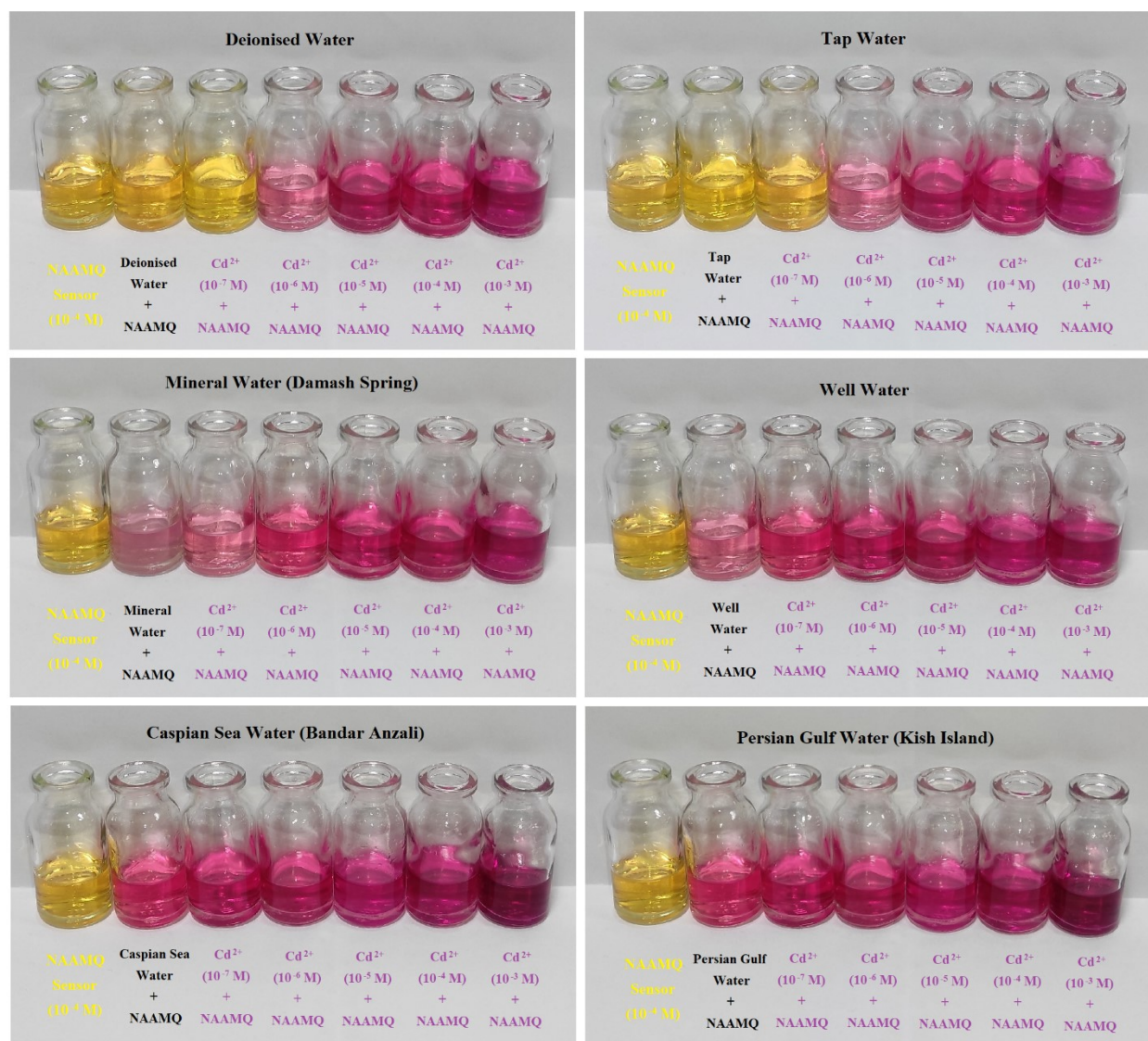
Figure S4. The color changes of the NAAMQ in acetonitrile/H 2 O (60:40, v/v) upon the addition of water samples and different concentrations of Cd 2+ ions at pH of 7.0.
