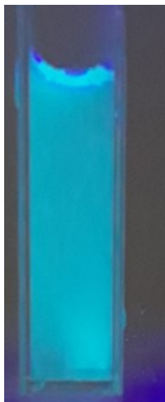
Fig. S1. Visible observation of the fluorescence of the synthesized 2D Ni nanosheets under UV light.
