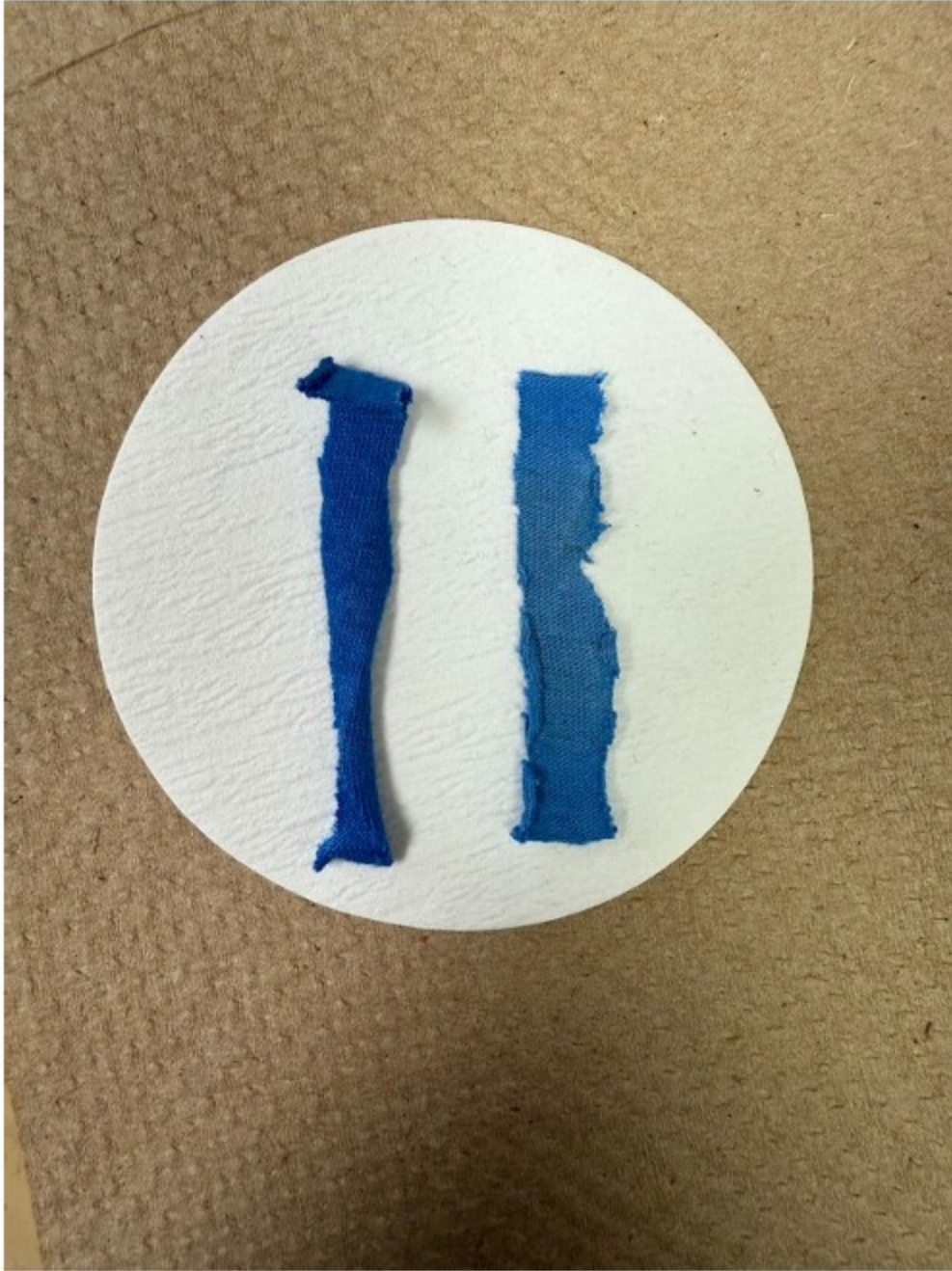
Figure S9. Blue-colored fabric at week 0 (left) and week 14 (right) after exposure to lake water.
