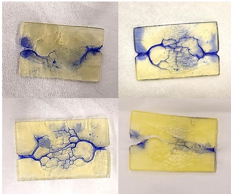
**ESI Figure 2.** Resulting perfusability tests for CAD designs containing hollow microchannels embedded within the part. As shown, most of the channels were blocked and the dyed solution was not able to perfuse due to the many overcured or blocked channels. Despite this, the fact that some dye was able to make it through suggests that a proper combination of optimized design and curing conditions could make this a possible method to explore in future studies.
