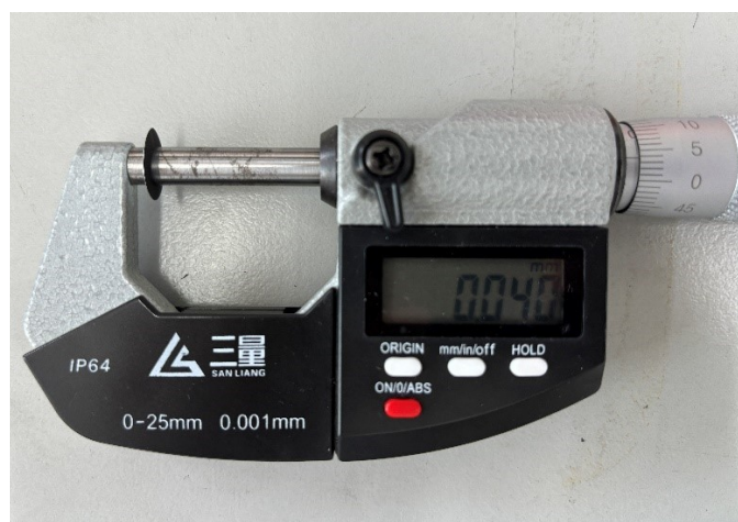
Fig. S15. Optical photograph of the thickness of the LFP positive electrode.
