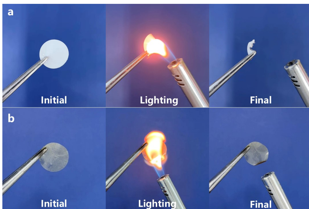
Fig. S4. Combustion experiments of (a) the PP separator and (b) the SICPE membrane.
