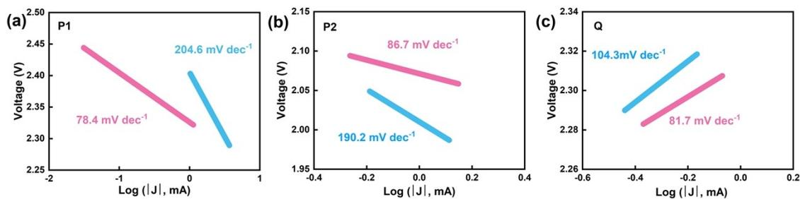
Fig.S10 Tafel plots for the redox peaks in the CV curves in Fig.2f
