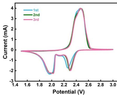
Fig.S9 CV curves of the DPIC@Li<sub>2</sub>S<sub>6</sub>/Li cell which employed a catholyte simultaneously containing Li<sub>2</sub>S<sub>6</sub> and DPIC at a scan rate of 0.1 mV s<sup>-1</sup>
