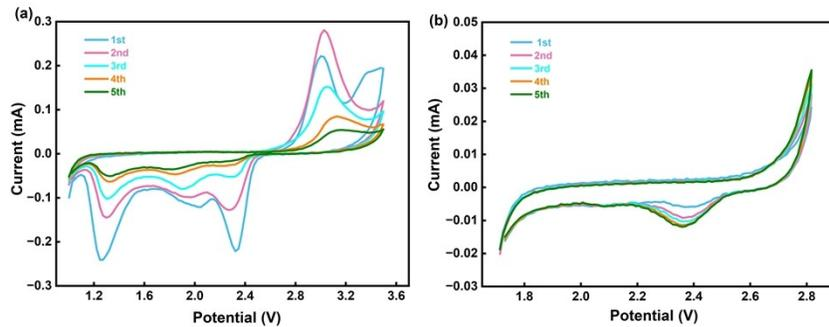
Fig.S7 CV curves of the DPIC/Li cell in the potential window of (a) 1.0~3.5 V and (b) 1.7~2.8 V, respectively (scan rate: 1 mV s<sup>-1</sup>)
