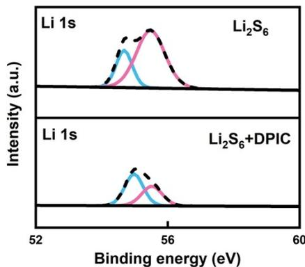
Fig.S2 Li 1s XPS spectra of  $\text{Li}_2\text{S}_6$  solution with/without DPIC
