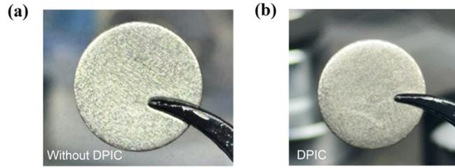
Fig.S4 Surface observation of Li metal after soaking in the electrolyte (a) without and (b) with DPIC for 7 days. The Li surface remains smooth and intact after soaking in the electrolyte with DPIC, and there is a negligible surface difference between the two cases.
