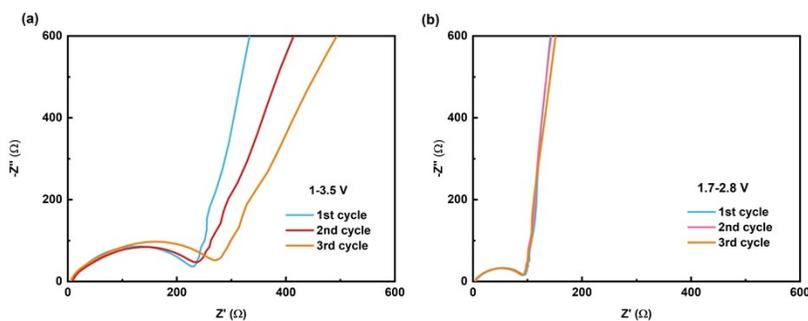
Fig.S8 EIS plots of the DPIC/Li cell during multiple CV scans in the potential window of (a) 1.0~3.5 V and (b) 1.7~2.8 V, respectively
