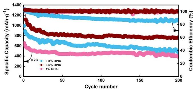
Fig.S11 Cycle performances of Li-S cells with different amounts of DPIC at 0.2C
