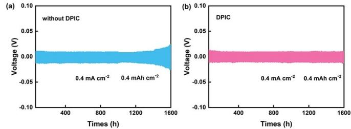
Fig.S5 Plating/stripping cycling tests of the Li symmetrical cells (a) without and (b) with DPIC. The Li symmetrical cell with DPIC delivers more stable plating/stripping cycling with a low overpotential over 1600 h at  $0.4 \text{ mA cm}^{-2}$  compared to the one without it.
