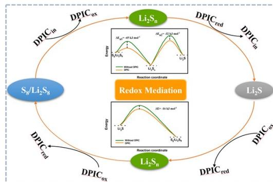
Fig.S6 Schematic diagram of DPIC mediated redox reaction in Li-S cell
