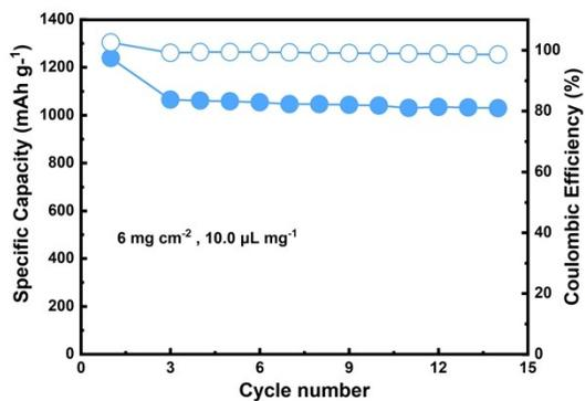
Fig.S12 Cycle test of the Li-S cell in the DPIC electrolyte at a sulfur loading of  $6 \text{ mg cm}^{-2}$  and E/S ratio of  $10.0 \text{ } \mu\text{L mg}^{-1}$  at 0.2C
