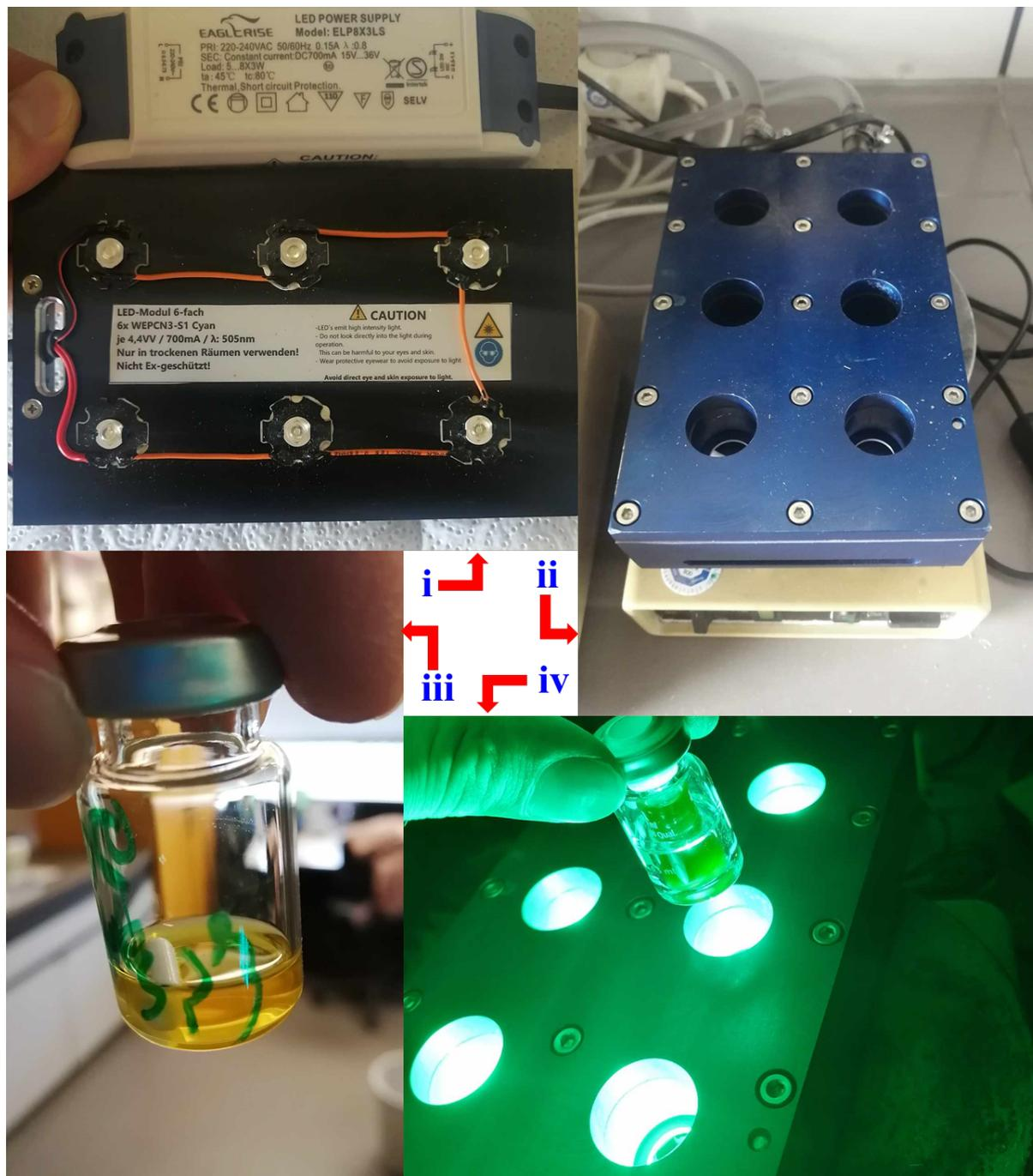
**Fig. S1:** (i) LED-s; (ii) Cooling block; (iii) 5 mL crimp-capped vial charged with reaction mixture and a stirring bar; (iv) Irradiation and cooling setup.
