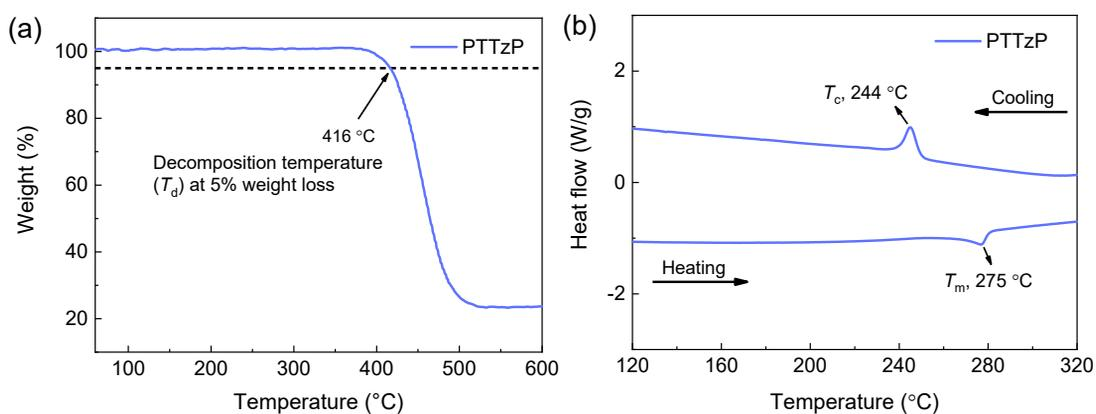
Figure S3. (a) TGA and (b) DSC curves of the polymer PTTzP.
