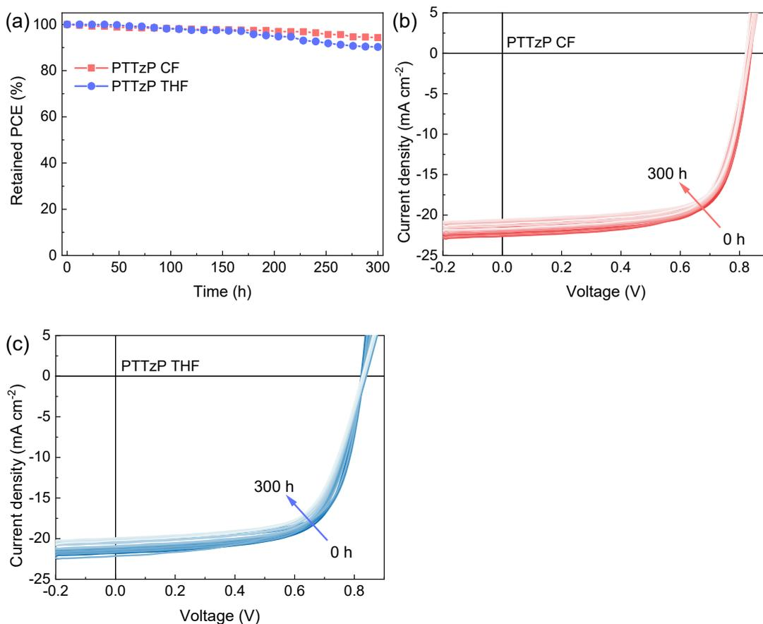
Figure S5. (a) Normalized performance loss of PCE during storage-stability tests, (b-c) devices recorded under AM1.5G illumination storage for 0 to 300 h, with arrows indicating the ageing trend.
