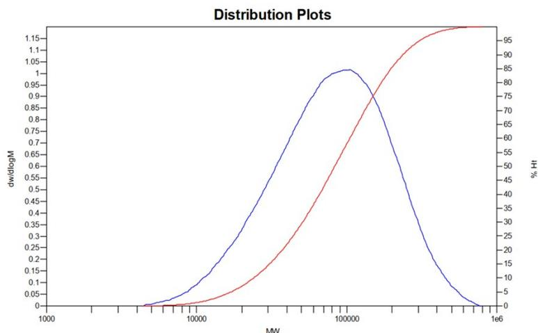
Figure S2. GPC traces of PTTzP measured at 150 °C with 1,2,4-trichlorobenzene as the eluent.
