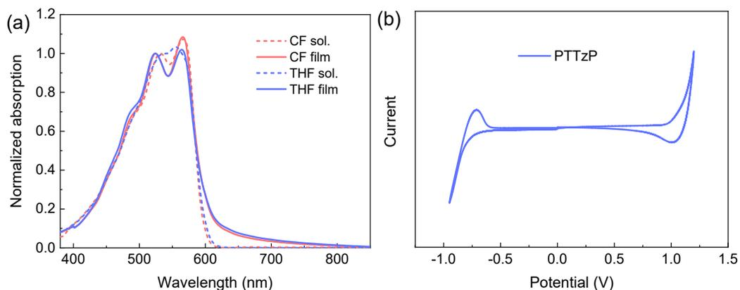
Figure S4. (a) The UV-Vis absorption spectra of PTTzP in CF and THF solution and thin films processed with CF and THF, respectively. (b) cyclic voltammogram of the polymer.
