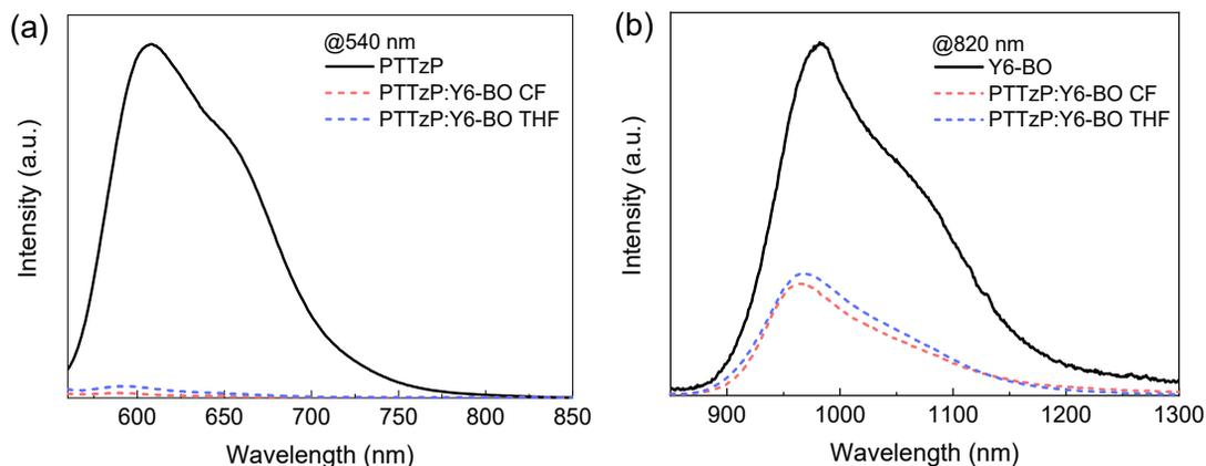
Figure S6. (a) PL spectra of PTTzP neat film and blend films with photoexcitation at 540 nm. (b) PL spectra of the Y6-BO neat film and blend films with photoexcitation at 820 nm.
