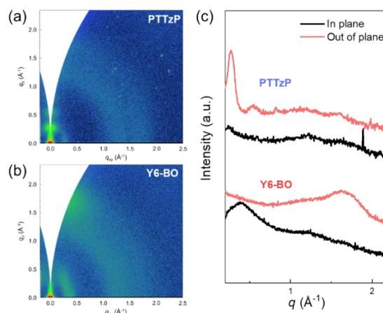
Figure S7. (a) Two-dimensional GIWAXS patterns and (b) one-dimensional line-cut profiles of PTTzP and Y6-BO neat films.
