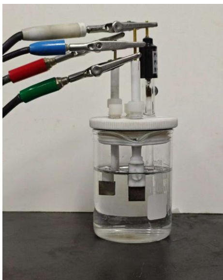
Fig. S6. The electrochemical device for OER performance test.
