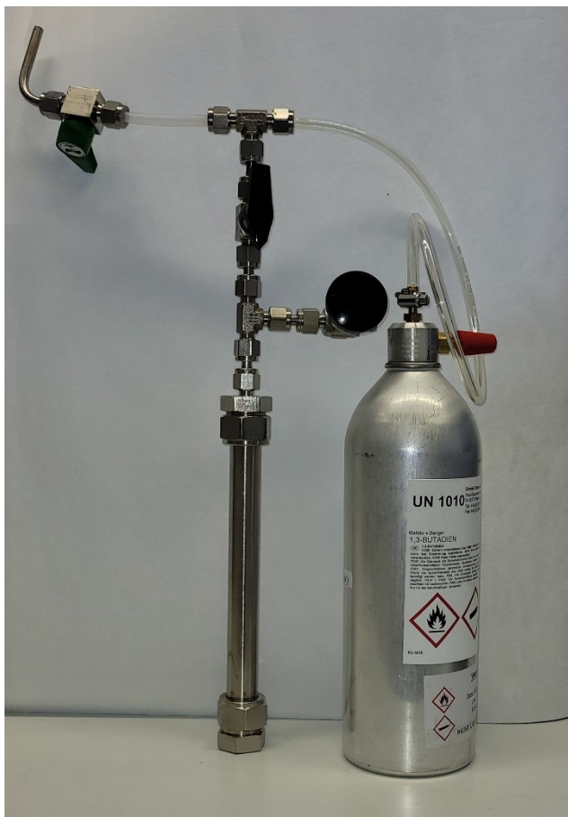
Figure S1 – 1,3-Butadiene bottle connected to container where 1,3-butadiene is condensed.
