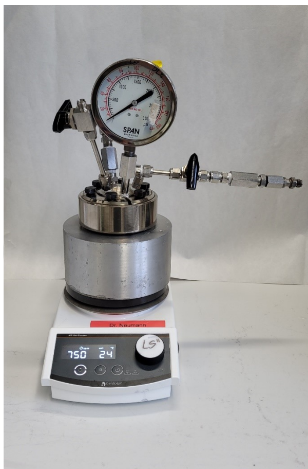
Figure S3 – Autoclave set for telomerization reaction the 1,3-butadiene.
