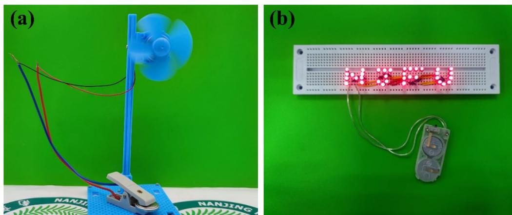
Fig. S4 Photos of fan powered by one SSC device (a) and LED beads powered by two devices in series (b).
