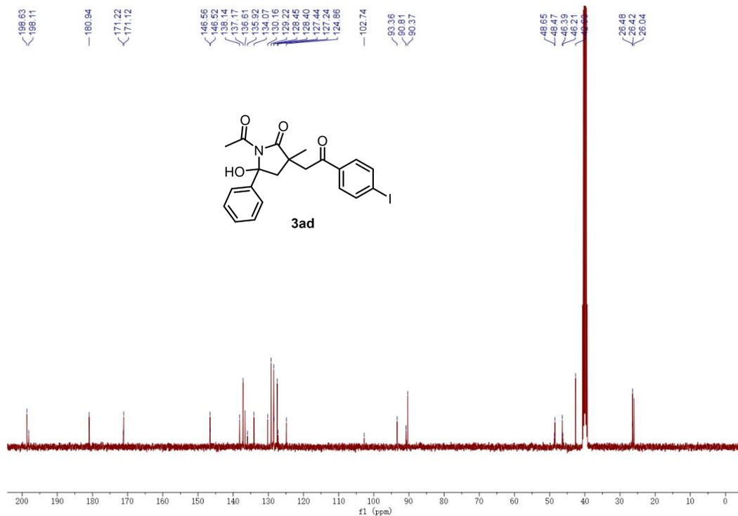
**13C NMR (101 MHz, DMSO-*d*<sub>6</sub>) spectrum of compound 3ad**
