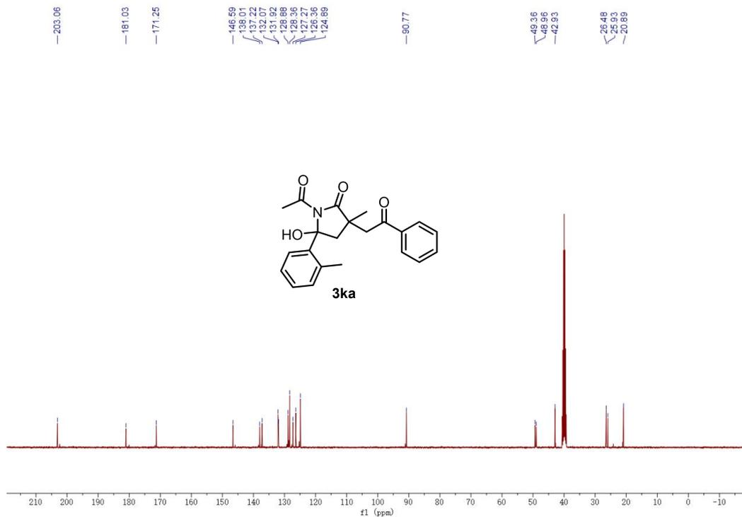
**<sup>13</sup>C NMR (101 MHz, DMSO-*d*<sub>6</sub>) spectrum of compound 3ka**
