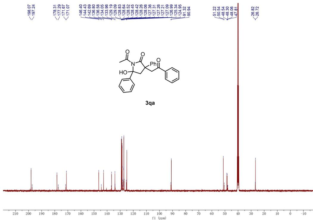
**<sup>13</sup>C NMR (101 MHz, DMSO-*d*<sub>6</sub>) spectrum of compound 3qa**
