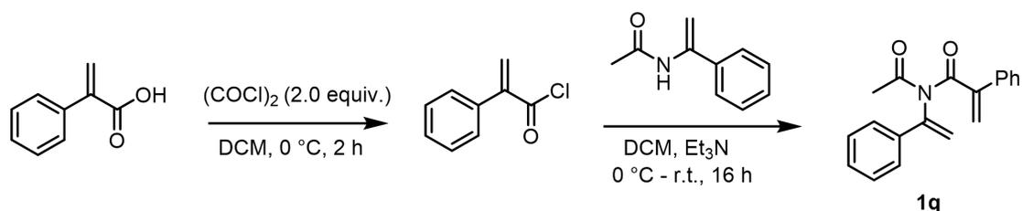
**General procedure for synthesis of 1,5-dienes 1q:** To a 100 mL round-bottom flask was successively charged with atropic acid (15.0 mmol, 1.5 equiv), a drop of DMF, dichloromethane (40.0 mL) and (COCl)<sub>2</sub> (3.8 g, 30 mmol, 2.0 equiv) at 0 °C. The reaction was stirred at this temperature for 1 h. The excess of (COCl)<sub>2</sub> was removed under reduced pressure and the corresponding crude acryloyl chloride was afforded.
