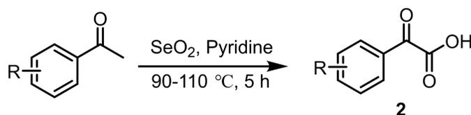
**General procedure for synthesis of benzoylformic acids 2a – 2j:** Add methyl ketone (5.0 mmol), SeO<sub>2</sub> (6.0 mmol), and 20.0 mL pyridine to a 50.0 mL round bottom bottle. Stir the reaction mixture in an oil bath at 110 °C for 1 h, then lower the
