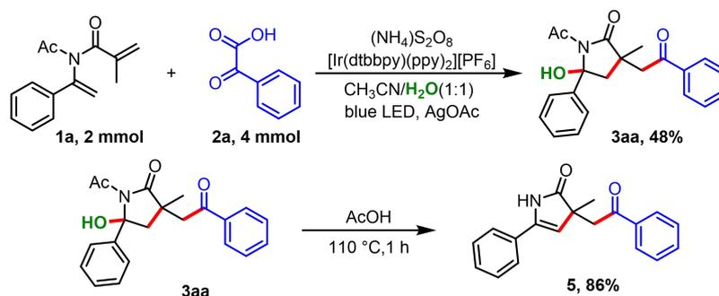
To an oven-dried 100 mL round-bottomed flask equipped with a magnetic stirring bar was added enamine amide **1a** (2.0 mmol, 0.458 g), benzoylformic acid **2a** (0.2 mmol, 0.6 g),  $(\text{NH}_4)_2\text{S}_2\text{O}_8$  (6.0 mmol, 1.369 g),  $[\text{Ir}(\text{dtbbpy})(\text{ppy})_2][\text{PF}_6]$  (2.0 mol%, 0.036 g), AgOAc (10.0 mol%, 0.033 g) and  $\text{CH}_3\text{CN}/\text{H}_2\text{O}$  (20 mL, 1:1) was
