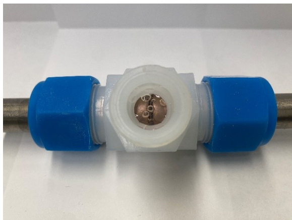
Figure S12. Photograph of the symmetric Mn || Mn Swagelok cell, featuring Mn free-standing film.
