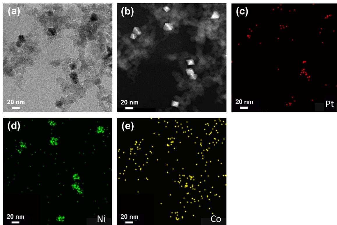
**Fig. S1** Characterization of PtNiCo@fumed. (a) TEM, (b) STEM, and (c, d, e) EDS elemental mapping images.
