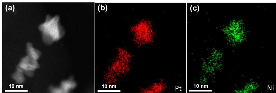
**Fig. S5** Characterization of PtNi/C. (a) STEM, and (b, c) EDS elemental mapping images.
