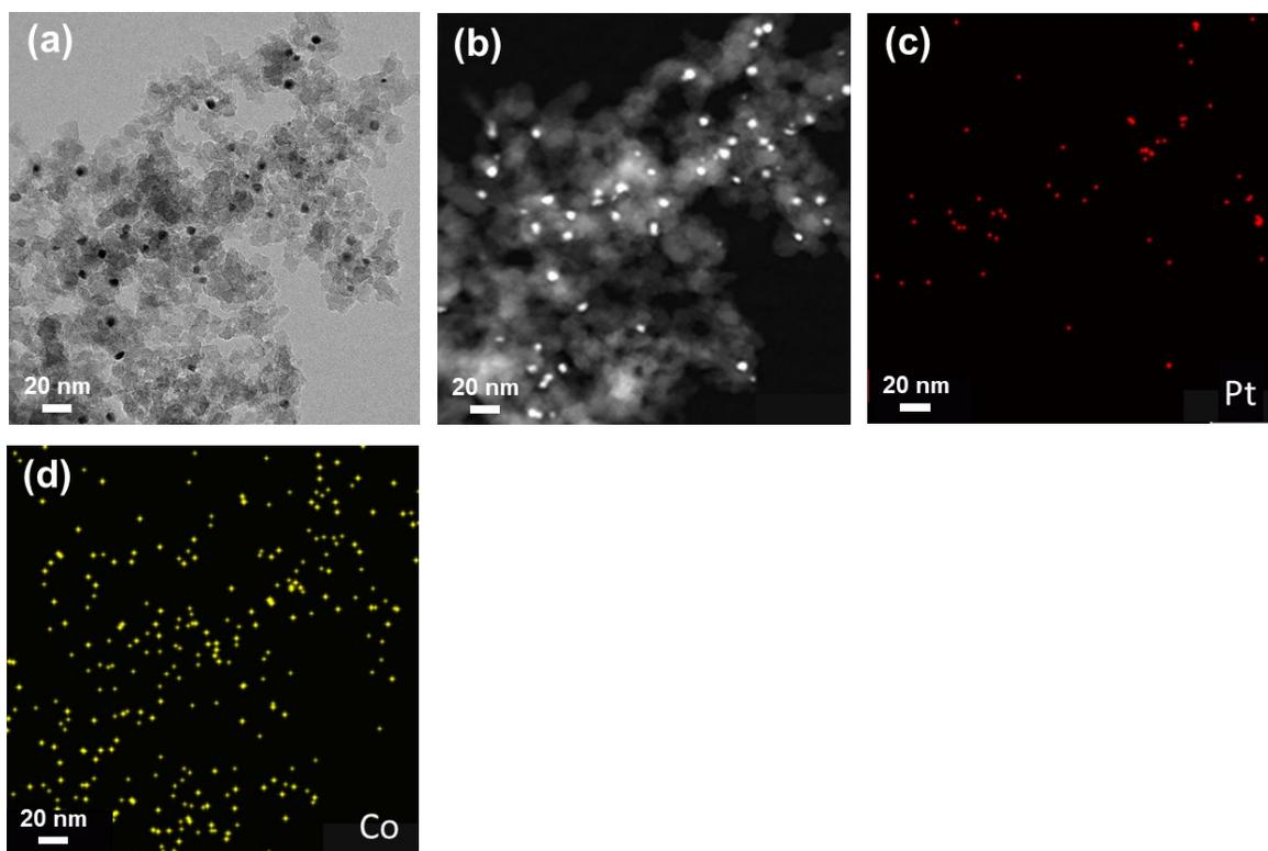
**Fig. S3** Characterization of PtCo@fumed. (a) TEM, (b) STEM, and (c, d) EDS elemental mapping images.
