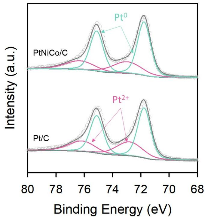
**Figure S4.** Core-level Pt 4f XPS spectra of PtNiCo/C and commercial Pt/C.
