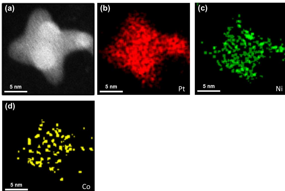
**Fig. S10** Characterization of PtNiCo/C after 20,000 cycles of stability test. (a) STEM, and (b, c, d) EDS elemental mapping images.
