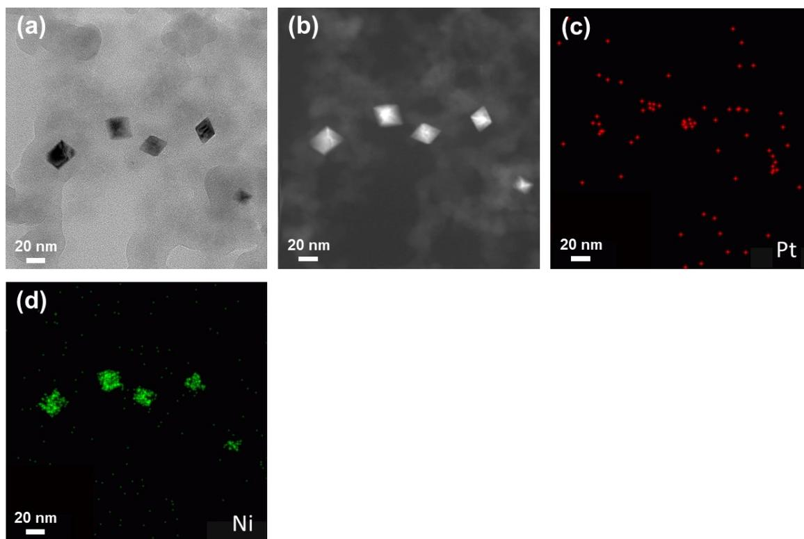
**Fig. S2** Characterization of PtNi@fumed. (a) TEM, (b) STEM, and (c, d) EDS elemental mapping images.
