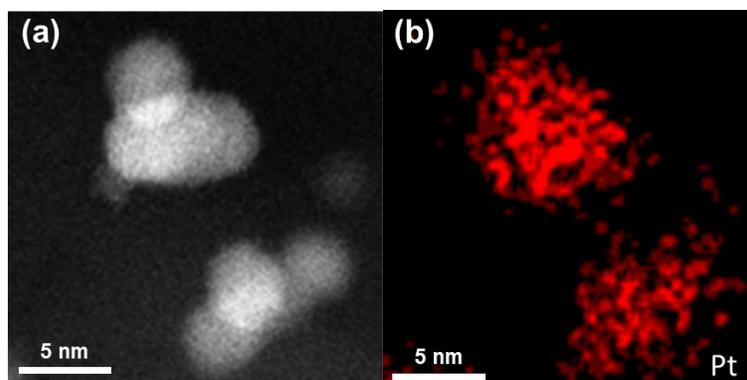
**Fig. S9** Characterization of commercial Pt/C after 20,000 cycles of stability test. (a) STEM, and (b) EDS elemental mapping images.
