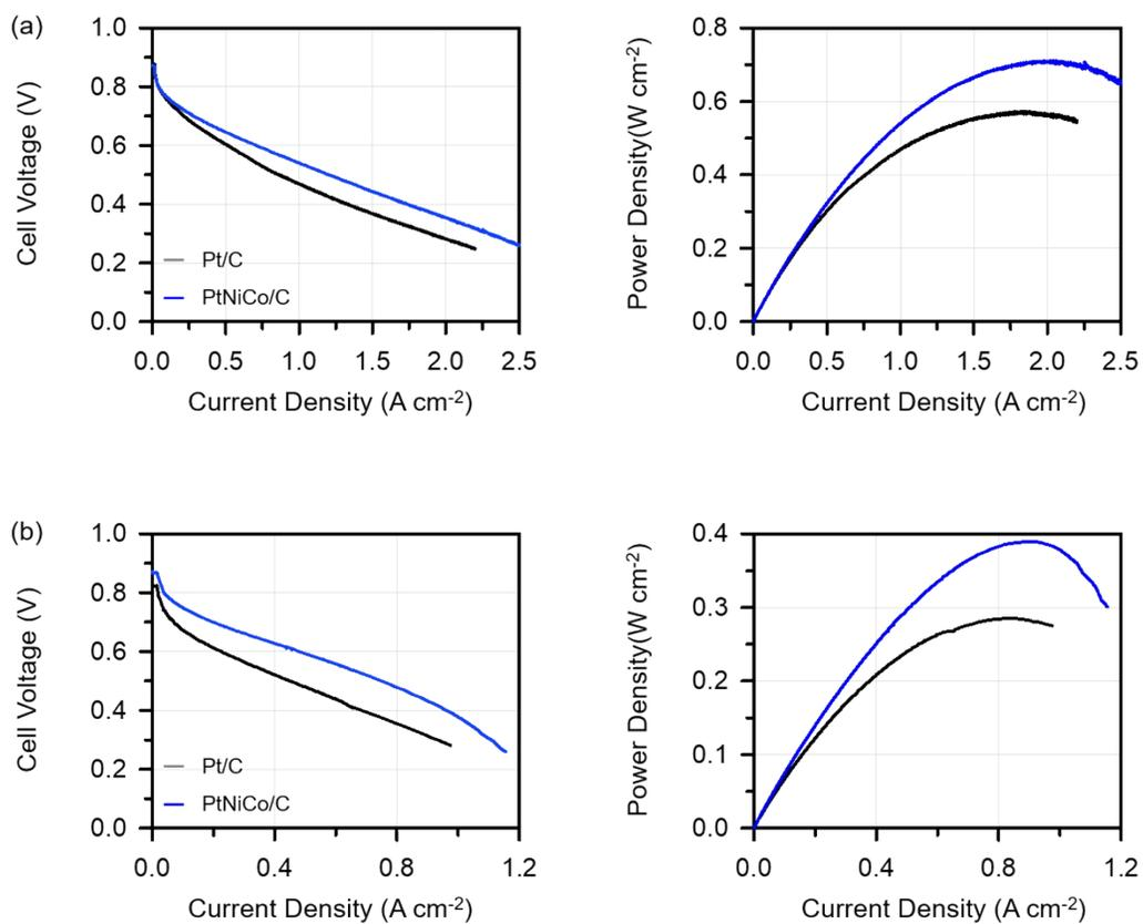
**Figure S11.**  $j$ - $V$  polarization and power density curves of Pt/C and PtNiCo/C MEA under (a) H<sub>2</sub>/O<sub>2</sub>, (b) H<sub>2</sub>/Air conditions.
