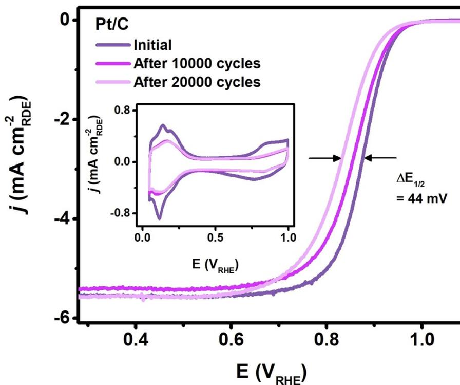
**Fig. S7** ORR polarization curves for Pt/C before and after 10,000 and 20,000 cycles in an O<sub>2</sub>-saturated 0.1 M HClO<sub>4</sub> solution. The insets displaying the CVs before and after the stability test.
