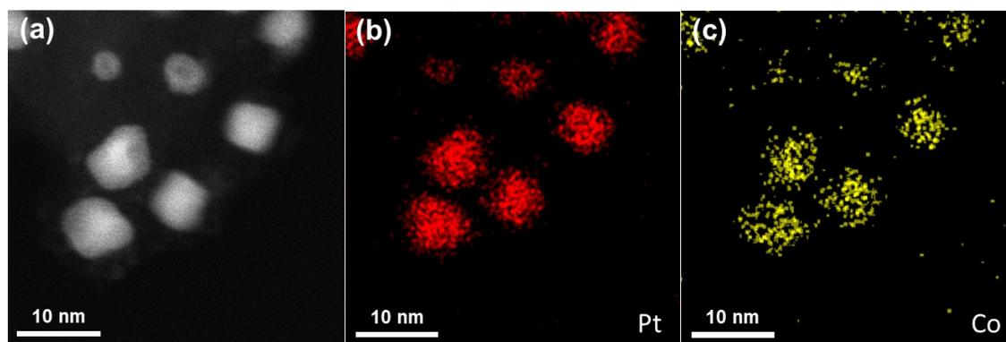
**Fig. S6** Characterization of PtCo/C. (a) TEM, (b) STEM, and (c, d) EDS elemental mapping images.
