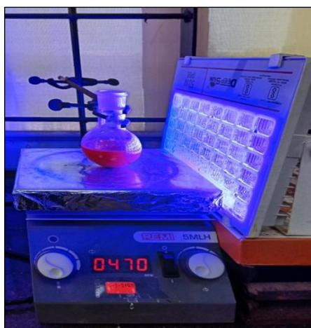
**Figure S2.** Reaction setup for gram scale synthesis of **1a**.
