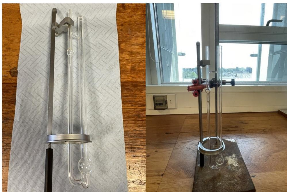
**Figure S3:** Photographs showing the Micro-Ostwald viscometer used to determine the viscosity of  $\text{NaPF}_6$  electrolyte solutions.
