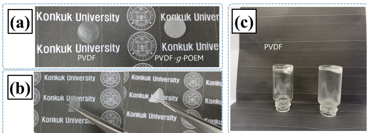
Figure S7. (a) Photographic images of the (a) hydrophobic PVDF and amphiphilic PVDF- g -POEM double comb copolymer based solid-state electrolyte (b) folded solid-state electrolytes held with tweezers (c) the solid-state electrolytes plasticized in DMF.
