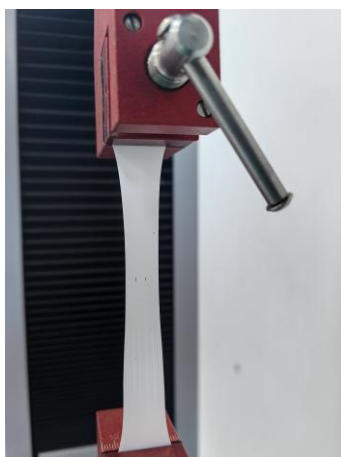
Fig. S7. Digital image of PVDF-HFP/NaTFSI/20BN CPE in stretched condition.
