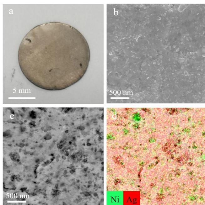
Figure S3. Characterizations of H-Ag/Ni electrode. (a) optical image. (b) Secondary electron image. (c) Backscattered electron image. (d) EDS elemental mapping.
