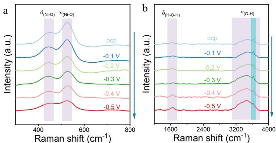
Figure S13. In situ Raman spectra of the H-Ag/Ni collected at different potentials within the range of 0 mV~ -500 mV in 1 M KOH electrolyte.
