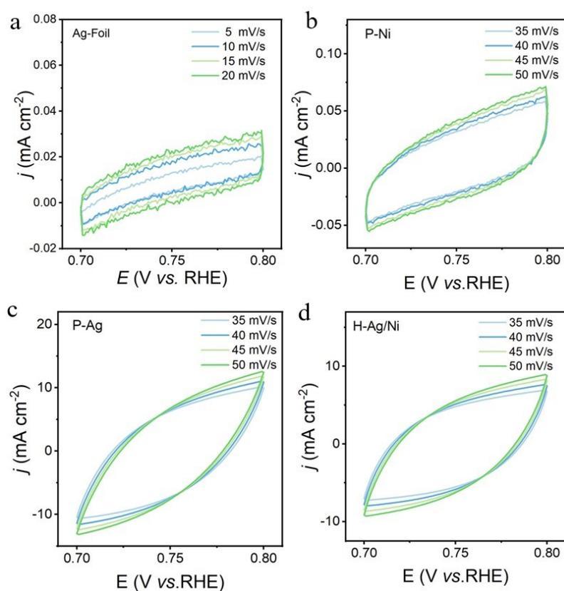
Figure S12. (a-d) Cyclic voltammograms at 5, 10, 15, and 20  $\text{mV s}^{-1}$  scan rates in the 0.7 V~0.8 V vs. RHE potential range. (a) Ag-Foil. (b) P-Ag. (c) P-Ni. (d) H-Ag/Ni.
