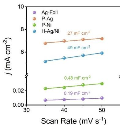
Figure S11. Electric double layer capacitance values ( $C_{dl}$ ) of Ag-Foil, P-Ag, P-Ni and H-Ag/Ni.
