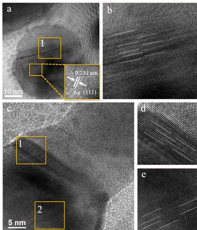
Figure S5. TEM images of H-Ag/Ni. (a) High-resolution TEM image. (b) Zoom-in image of zone 1 in Fig. a. (c) High-resolution TEM image. (d) Magnified image of zone 1 in Figure. c. (e) Magnified image of zone 2 in Figure c.
