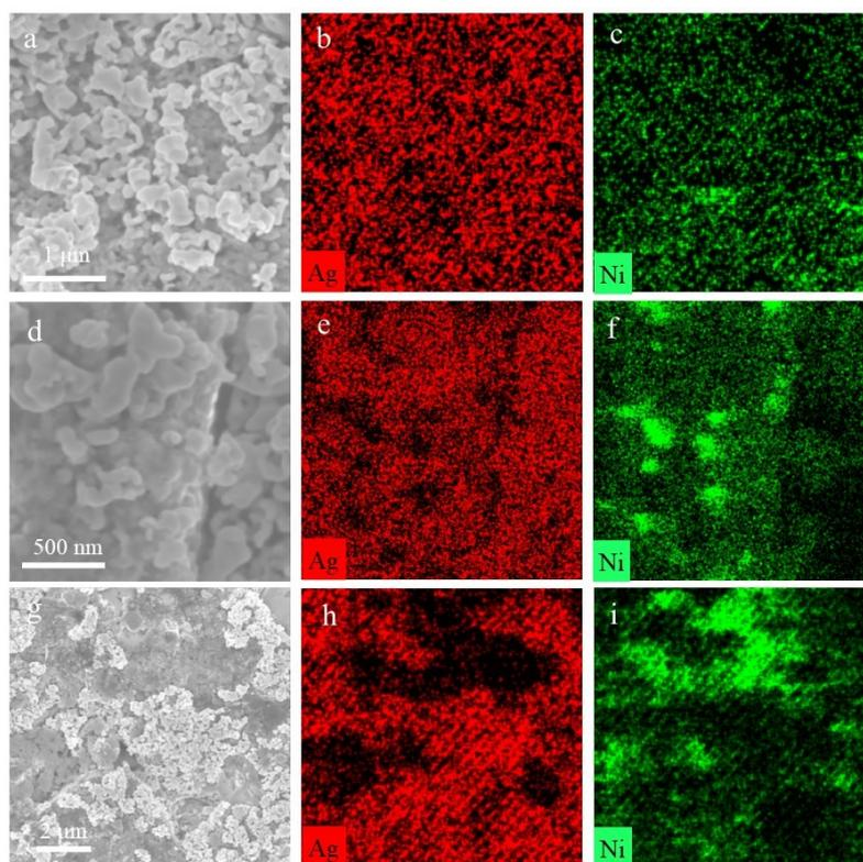
Figure S6. SEM images of H-Ag/Ni-10%, H-Ag/Ni, and H-Ag/Ni-30%. (a)(b)(c) H-Ag/Ni-10%. (d)(e)(f) H-Ag/Ni. (g)(h)(i) H-Ag/Ni-30%.
