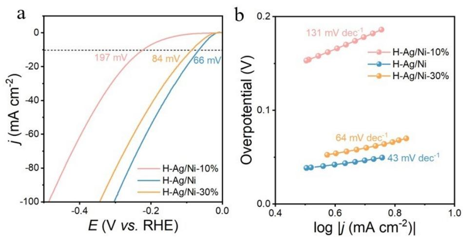
Figure S7. HER performance of different catalysts in 1 M KOH. (a) LSV curves of H-Ag/Ni-10%, H-Ag/Ni and H-Ag/Ni -30%. (b) Tafel slope plot based on the LSV curves in Figure. a.
