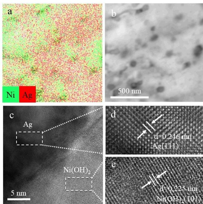
Figure S15. SEM and TEM images of H-Ag/Ni self-supported electrode after stability test. (a) EDS mapping image. (b) Backscattered electron image. (c) HRTEM image. (d-e) Zoom-in images of the selected zone in Fig. c.
