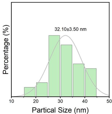
Figure S4. Histogram of particle size distribution of Ni(OH)<sub>2</sub> nanoparticles in H-Ag/Ni.
