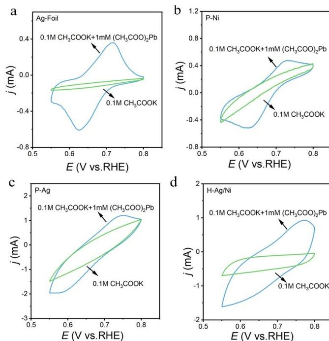
Figure S10. Pb adsorption-desorption voltammograms of (a) Ag-Foil, (b) P-Ag, (c) P-Ni and (d) H-Ag/Ni in 0.1 M  $\text{CH}_3\text{COOK}$  + 1 mM  $(\text{CH}_3\text{COO})_2\text{Pb}$ .
