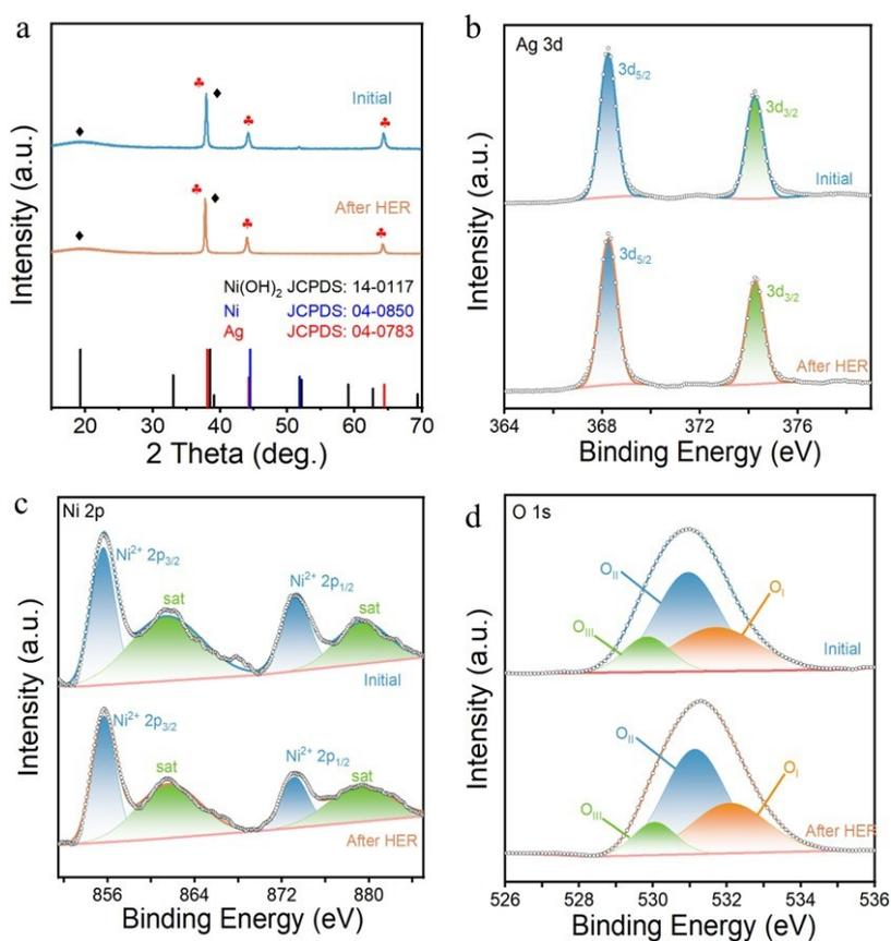
Figure S14. XRD and XPS characterizations of H-Ag/Ni initial and after stability test. (a) XRD. (b) XPS spectra of Ag 3d. (c) XPS spectra of Ni 2p. (d) XPS spectra of O 1s.
