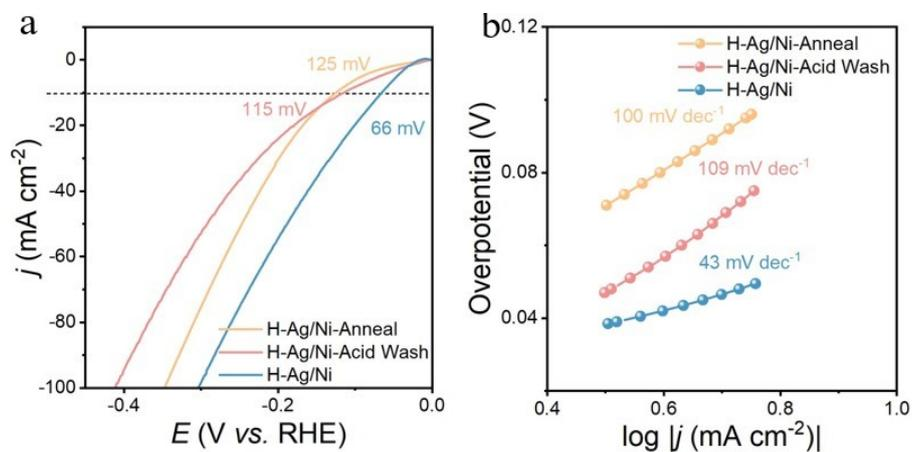
Figure S16. HER performance of different catalysts in 1 M KOH. (a) LSV curves of H-Ag/Ni-Anneal, H-Ag/Ni-Acid Wash and H-Ag/Ni. (b) Tafel slope plot based on the LSV curves in a.
