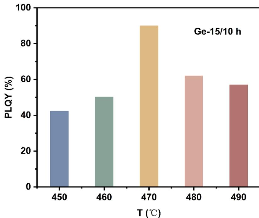
**Figure S2** PLQY Intensity of CsPbBr<sub>3</sub>@Glass samples with different heat treatment temperature.
