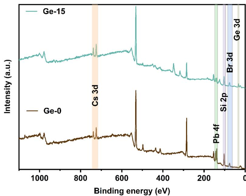
**Figure S3** XPS survey spectra of Si 2p, Ge 3d, Cs 3d, Pb 4f and Br 3d in Ge-0, Ge-15 samples.
