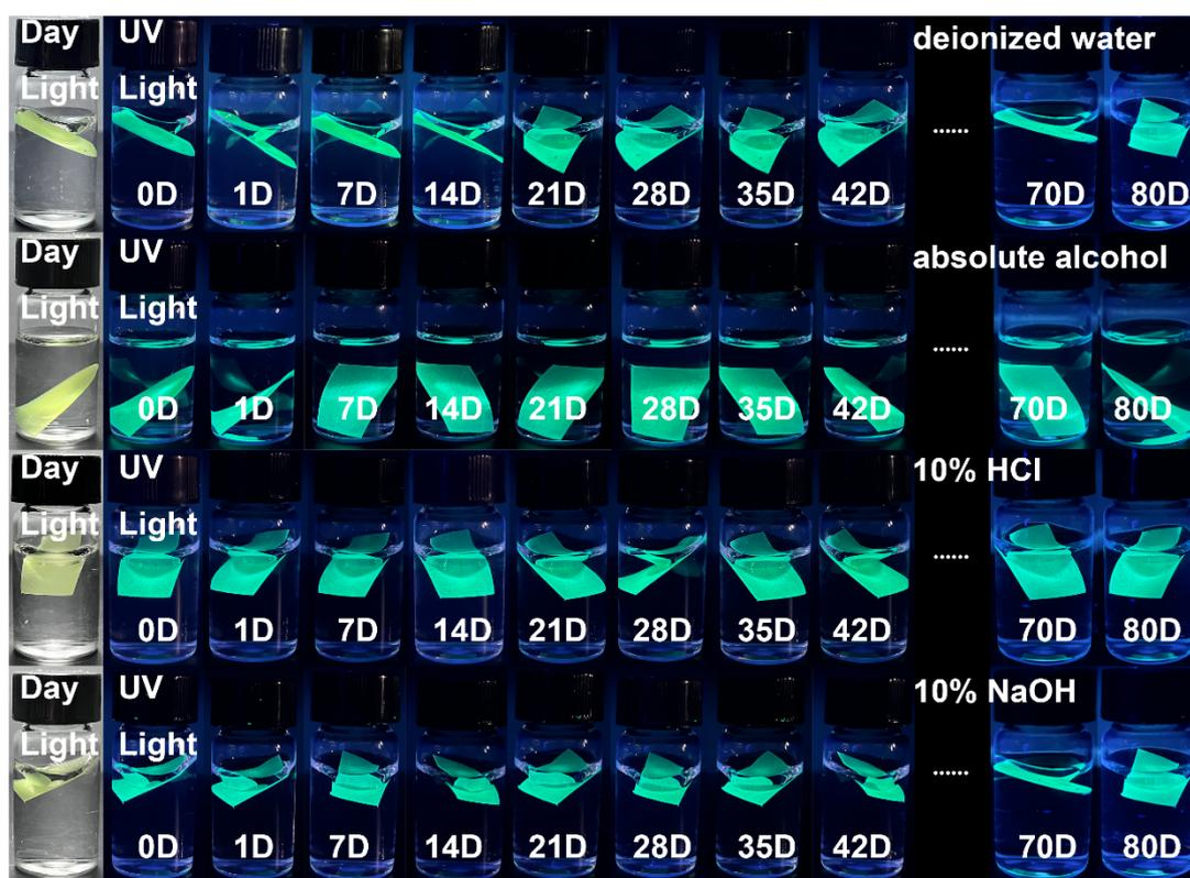
**Figure S7** The day light and UV light photographs of CsPbBr<sub>3</sub>@Glass@EVA film in four different solutions for 80 days.
