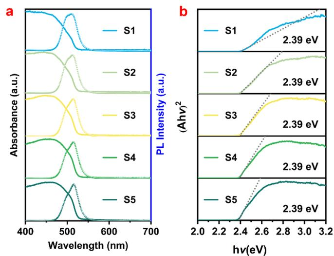
**Figure S6** (a) The fluorescence spectra and UV-Vis absorption spectra and (b) bandgap spectra of the CsPbBr<sub>3</sub>@Glass@EVA film samples.
