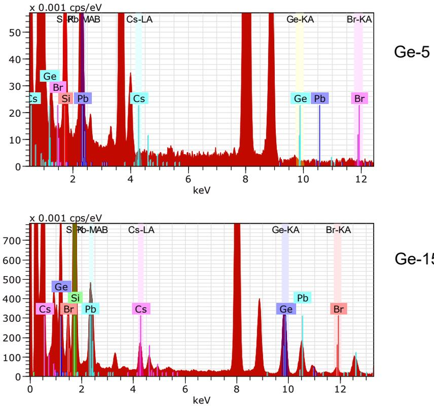
**Figure S4** EDX spectrum of the as-prepared Ge-5 and Ge-15 glass sample, showing the existence of Cs, Pb, Br, Si and Ge elements.
