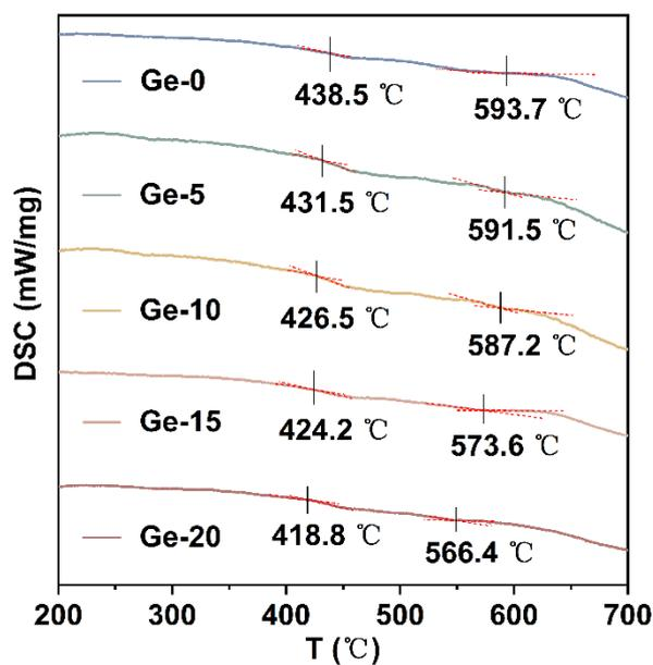
**Figure S1** DSC curves of five kinds of CsPbBr<sub>3</sub>@Glass with different GeO<sub>2</sub> contents without heat treatment.
