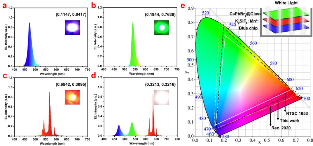
**Figure S8** The PL spectra of blue chips, green CsPbBr<sub>3</sub>@Glass composites, red K<sub>2</sub>SiF<sub>6</sub>:Mn<sup>4+</sup> phosphor and WLED, insets included blue, green, red and white light, respectively. (e) Color gamut of NSTC 1953 standard (white line), the Rec. 2020 standard (yellow line) and this work (black line) in the CIE diagram, inset was the structural schematic of WLED.
