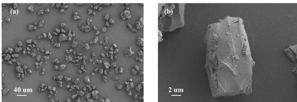
**Fig. S7.** The scanning electron microscopy of  $\text{Na}_{2/3}[\text{Fe}_{1/3}\text{Mn}_{2/3}]\text{O}_2$  material.
