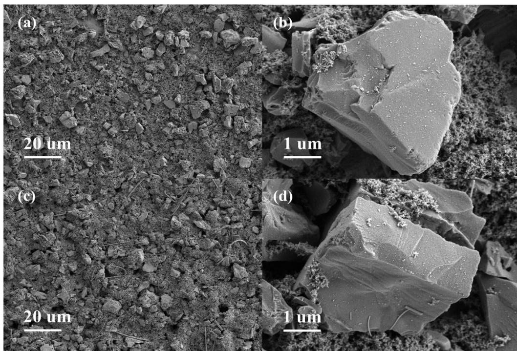
**Fig. S5.** The SEM image of the NaSn@HC anode, (a, b) before cycling and (c, d) after 100 cycles in the full cell.
