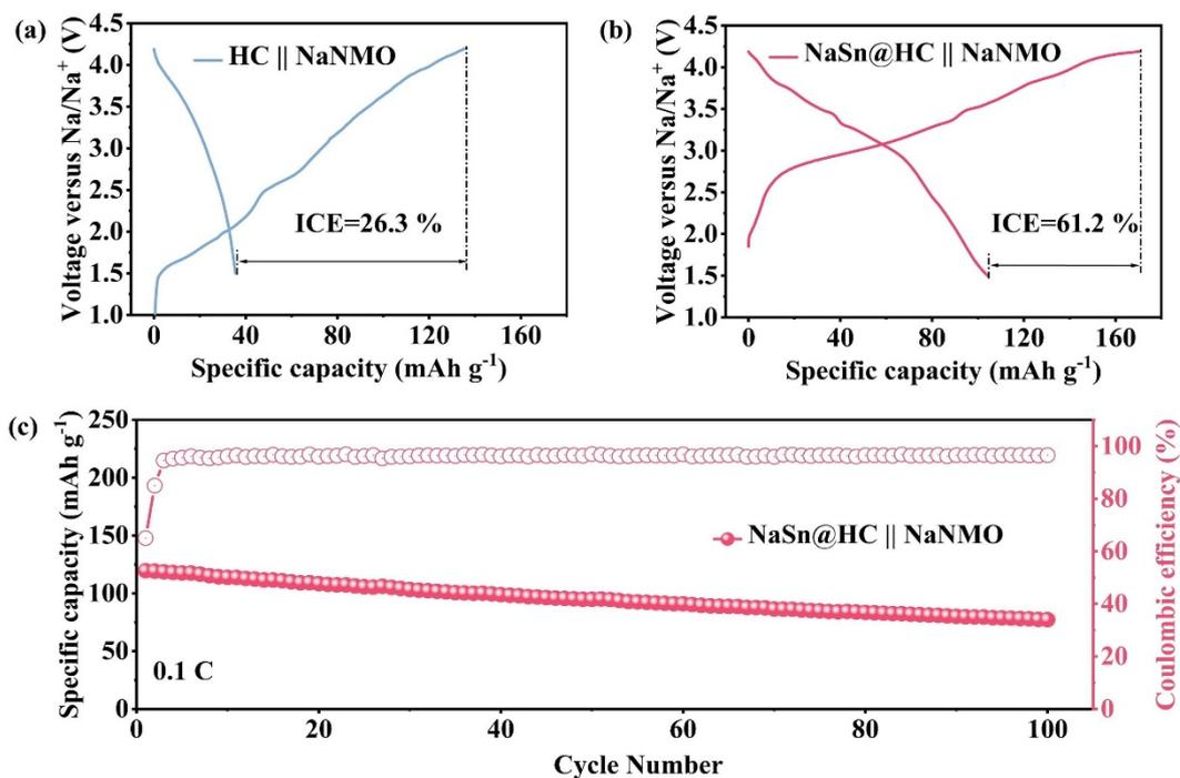
**Fig. S8** (a) First loop charge-discharge curve of NaNMO || HC full cell and (b) NaNMO || NaSn@HC full cell; (c) The long-term cycling performance of NaNMO || NaSn@HC full cell.
