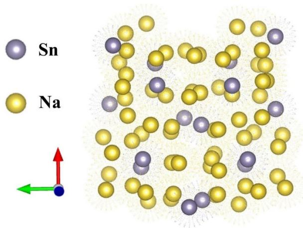
**Fig. S2.** crystal structures of  $\text{Na}_{15}\text{Sn}_4$ .
