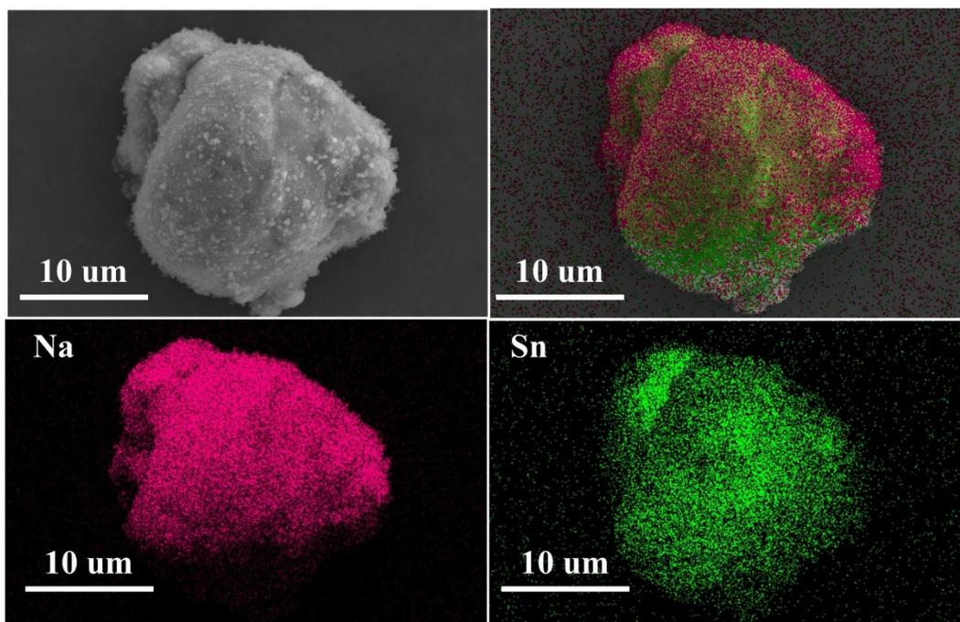
**Fig.** S1. EDS maps of  $\text{Na}_{15}\text{Sn}_4$ .
