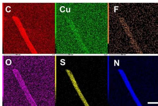
Fig. S11. Elemental mapping of MNP by TEM (scale bar = 200 nm).
