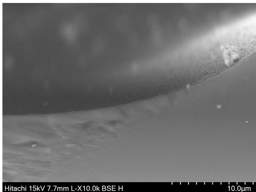
**Figure S17** The cross-sectional SEM image of MIL-100 capillary column.
