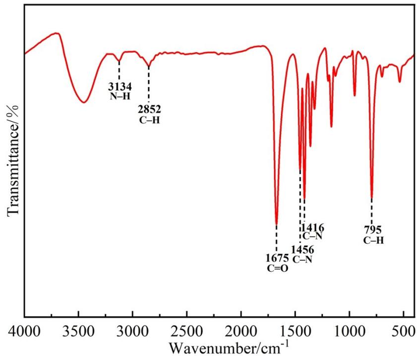
**Figure S10** The FTIR spectra of ZIF-90 (The strong absorption peak observed around 3500 cm<sup>-1</sup> is attributed to residual methanol in the sample).
