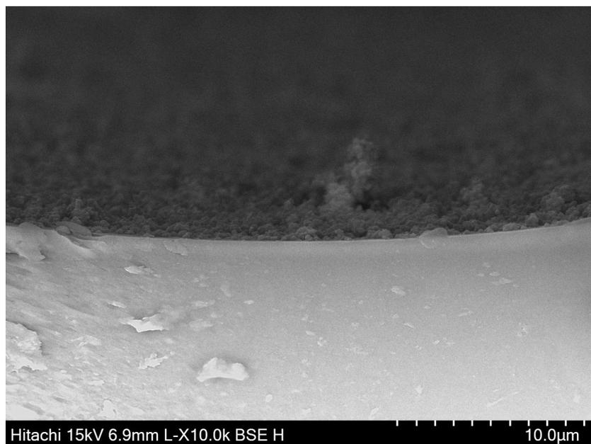
**Figure S14** The cross-sectional SEM image of ZIF-90 capillary column.
