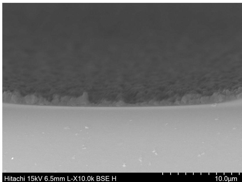
**Figure S15** The cross-sectional SEM image of Cu-BTC capillary column.
