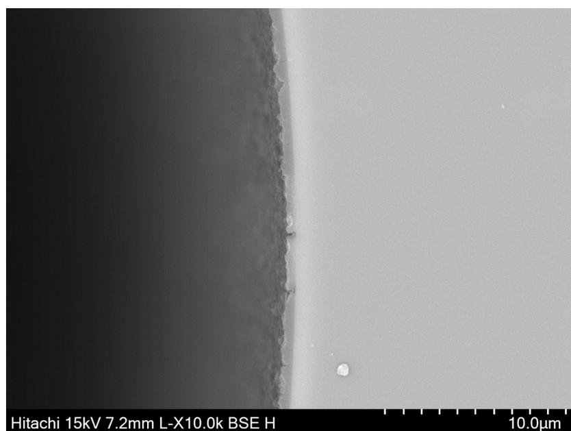
**Figure S21** Cross-sectional SEM image of ZIF-8 capillary column (LBL 120 times).
