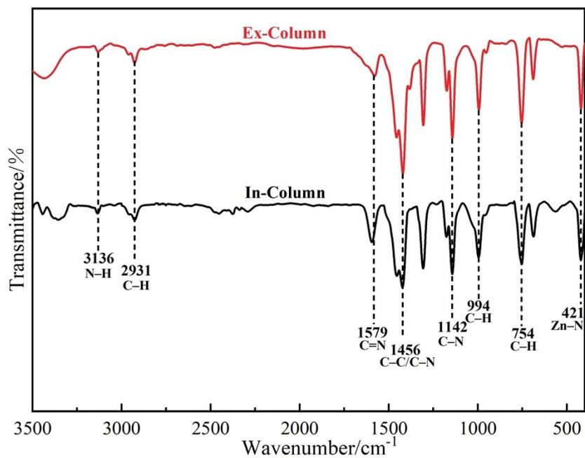
**Figure S2** The FTIR spectra of ZIF-8.
