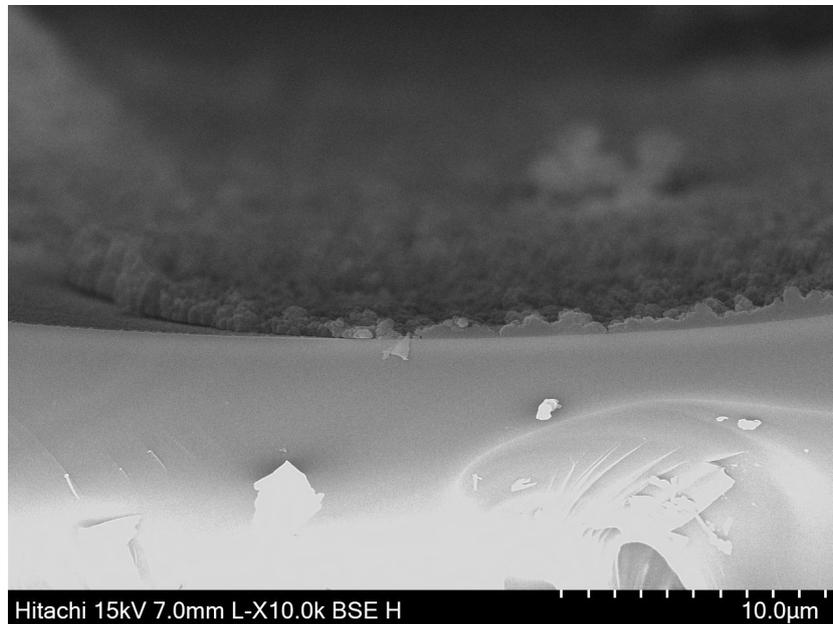
**Figure S19** The cross-sectional SEM image of UiO-66-NH<sub>2</sub> capillary column.
