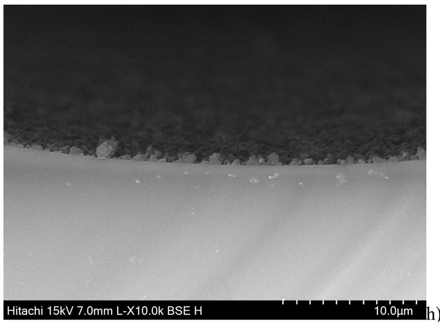
**Figure S28** Cross-sectional SEM image of ZIF-8 capillary column (Continuous flow preparation, Zn(II) 0.05 M and 2-IM 0.1 M, 6 h).
