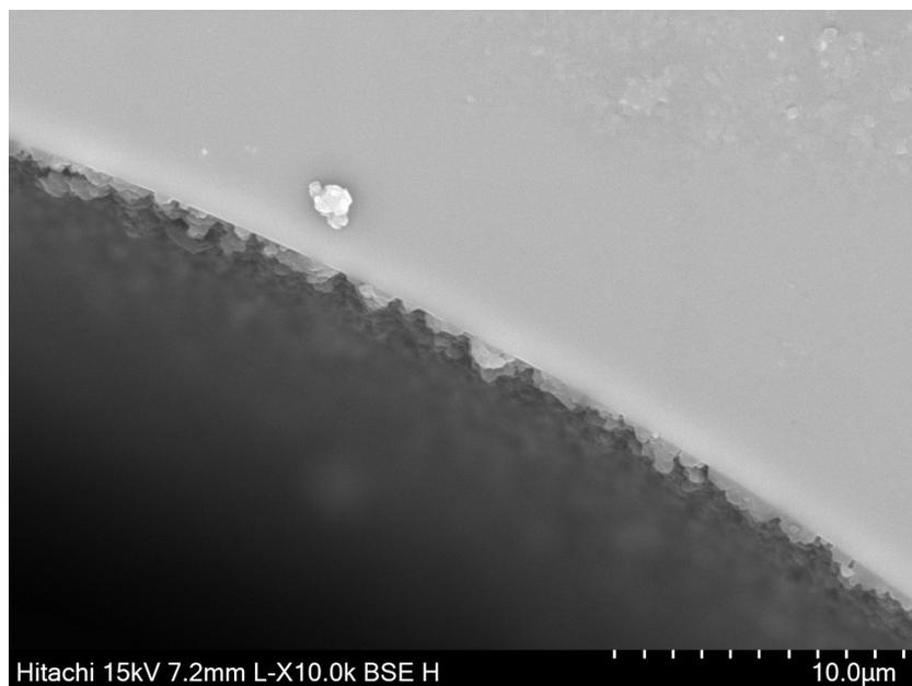
**Figure S18** The cross-sectional SEM image of UiO-66 capillary column.
