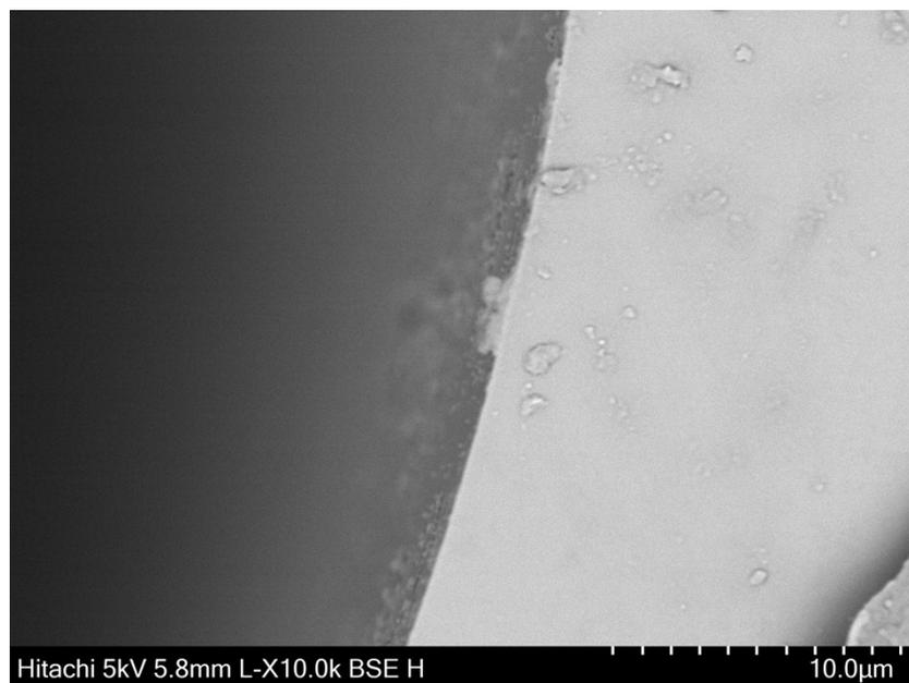
**Figure S22** The cross-sectional SEM image of ZIF-8 capillary column (In-situ growth).
