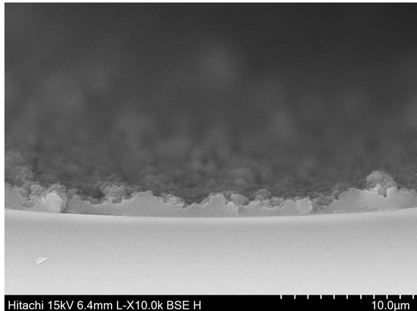
**Figure S23** The cross-sectional SEM image of ZIF-8 capillary column (Continuous flow preparation, Zn(II) 0.1 M and 2-IM 0.2 M, 8 h).
