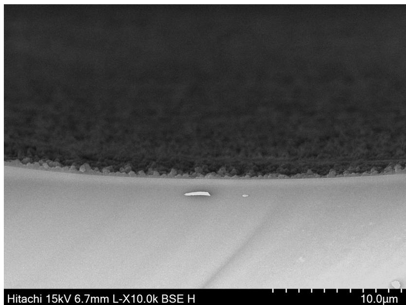
**Figure S16** The cross-sectional SEM image of ZIF-67 capillary column.
