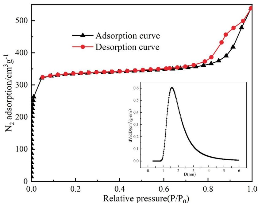
**Figure S4** N<sub>2</sub> adsorption-desorption curve and pore size distribution of ZIF-8.
