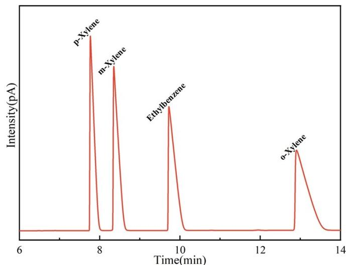
**Figure S8** Chromatographic profile of xylene isomers separated on UiO-66-NH<sub>2</sub> capillary column. **Chromatographic conditions:** flow rate of 30 cm/s; column temperature held at 100 °C for 1 min, then increased to 200 °C at a rate of 30 °C/min.
