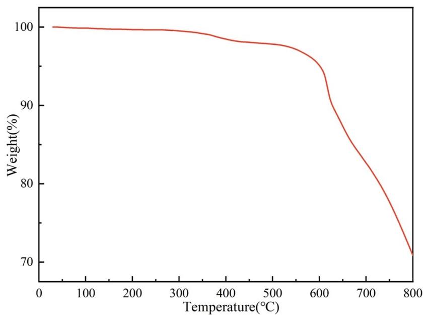
**Figure S3** The TGA curve of ZIF-8 in  $N_2$  atmosphere.
