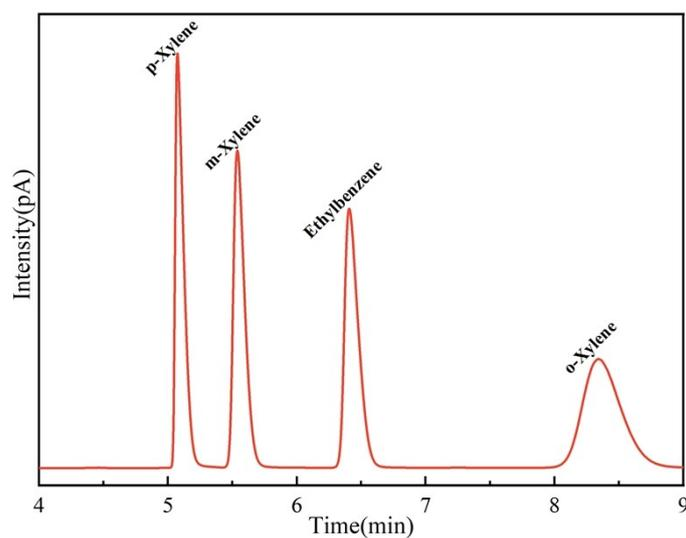
**Figure S7** Chromatographic profile of xylene isomers separated on UiO-66 capillary column. **Chromatographic conditions:** flow rate of 30 cm/s; column temperature held at 100 °C for 1 min, then increased to 200 °C at a rate of 30 °C/min.
