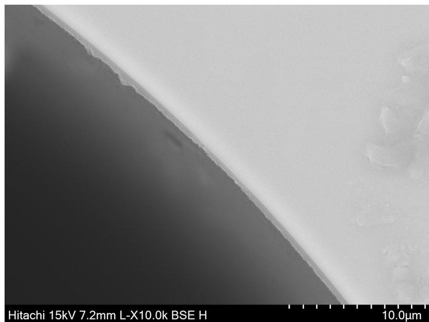
**Figure S20** The cross-sectional SEM image of ZIF-8 capillary column (LBL 60 times).
