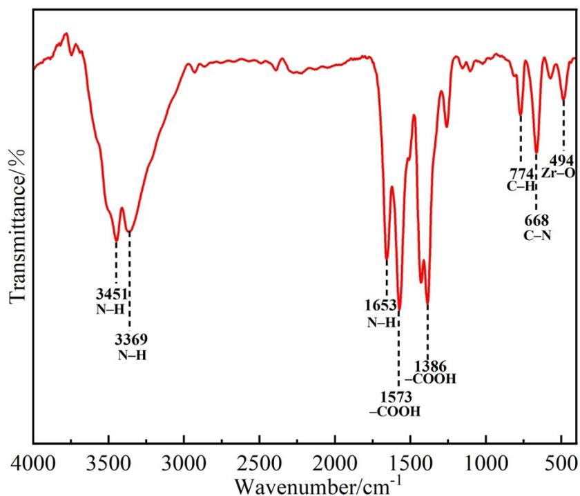
**Figure S9** The FTIR spectra of UiO-66-NH<sub>2</sub>.
