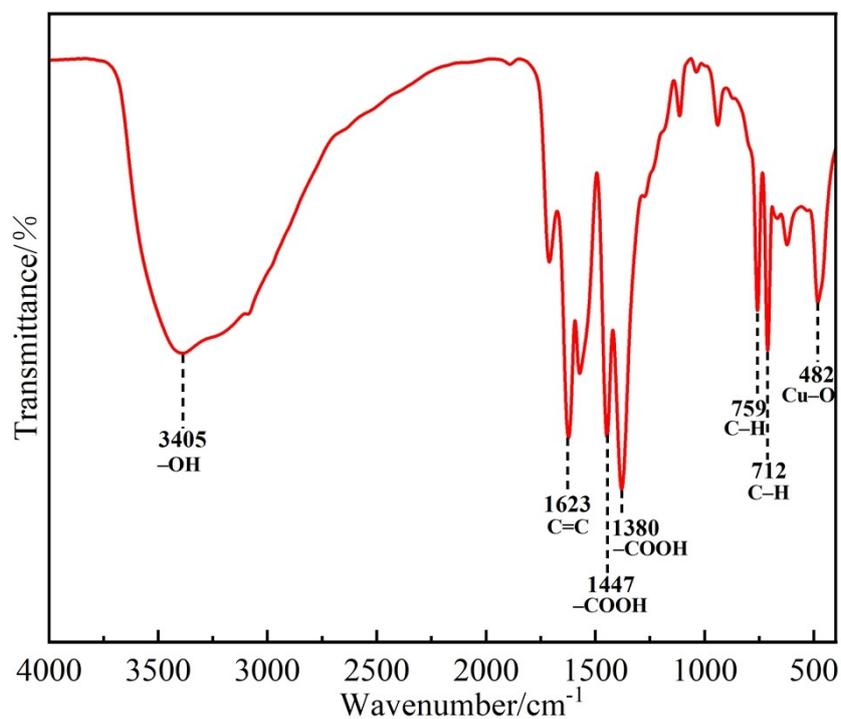
**Figure S11** The FTIR spectra of Cu-BTC.
