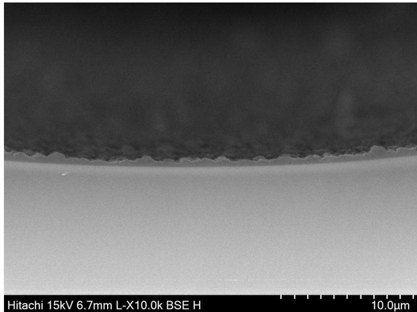
**Figure S25** The cross-sectional SEM image of ZIF-8 capillary column (Continuous flow preparation, Zn(II) 0.1 M and 2-IM 0.2 M, 4 h).
