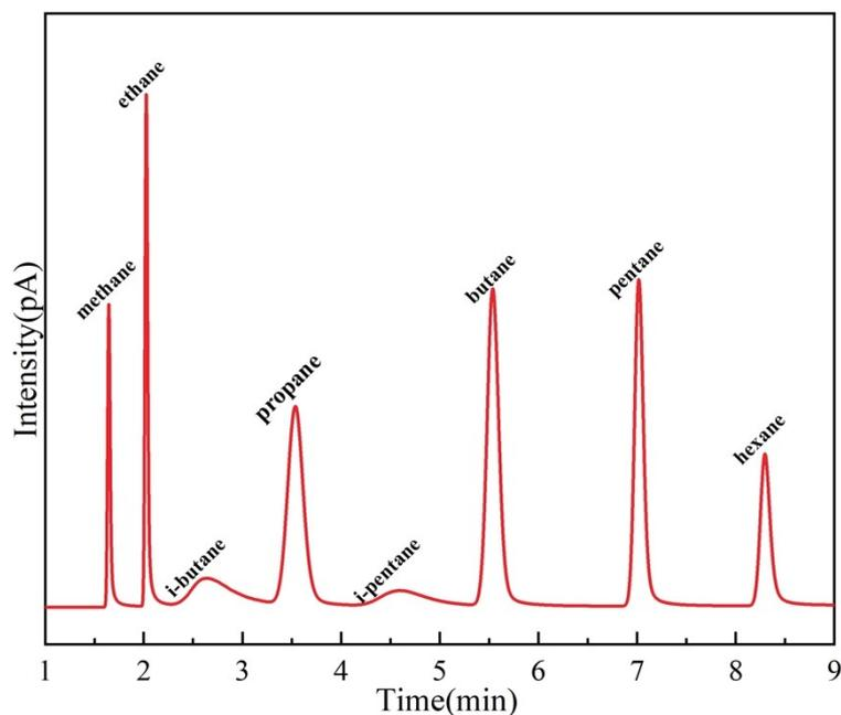
**Figure S6** Chromatographic profile of C1-C6+ alkane mixture separated on ZIF-8 capillary column fabricated via optimized protocol.
