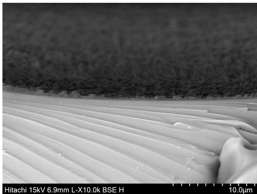
**Figure S24** The cross-sectional SEM image of ZIF-8 capillary column (Continuous flow preparation, Zn(II) 0.1 M and 2-IM 0.2 M, 2 h).
