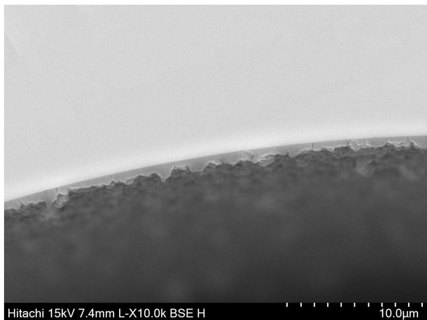
**Figure S26** The cross-sectional SEM image of ZIF-8 capillary column (Continuous flow preparation, Zn(II) 0.1 M and 2-IM 0.2 M, 6 h).
