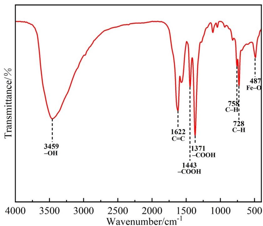
**Figure S13** The FTIR spectra of MIL-100.
