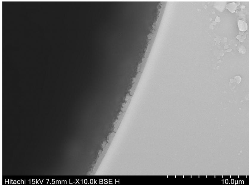
**Figure S27** The cross-sectional SEM image of ZIF-8 capillary column (Continuous flow preparation, Zn(II) 0.025 M and 2-IM 0.05 M, 6 h).
