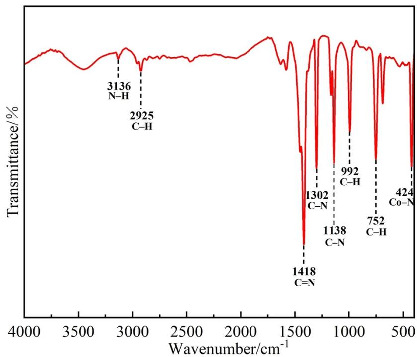
**Figure S12** The FTIR spectra of ZIF-67.
