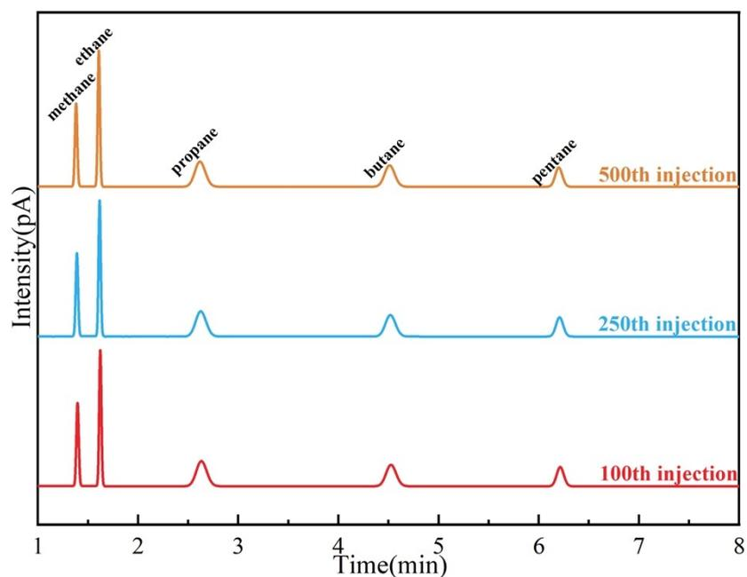
**Figure S5** Stability evaluation of the ZIF-8 capillary column fabricated under optimized preparation protocol. **Chromatographic conditions:** flow rate of 15 cm/s; column temperature held at 35 °C for 1.5 min, then increased to 200 °C at a rate of 30 °C/min.
