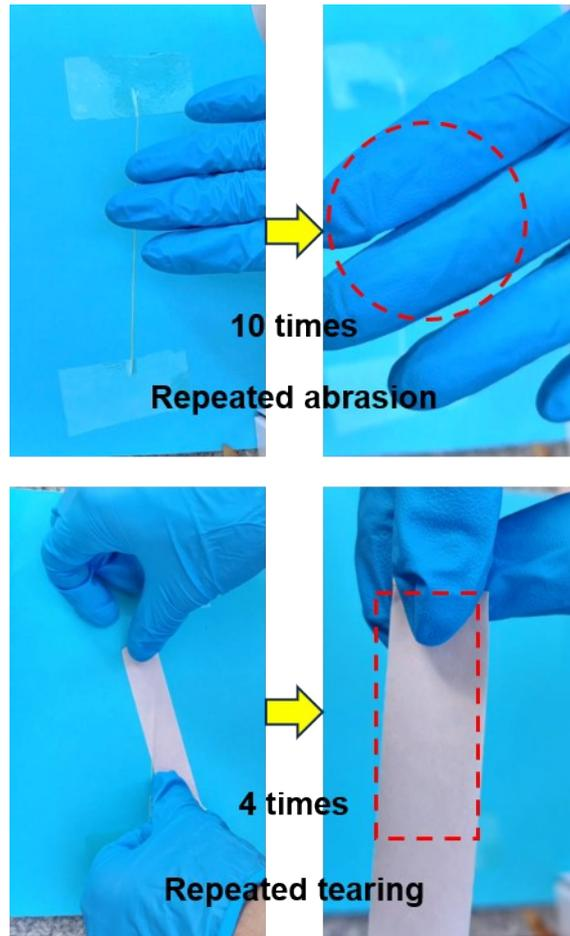
**Fig. S1** The present study investigates the stability of yarn surface coatings through the repeated rubbing of gloves against tape.
