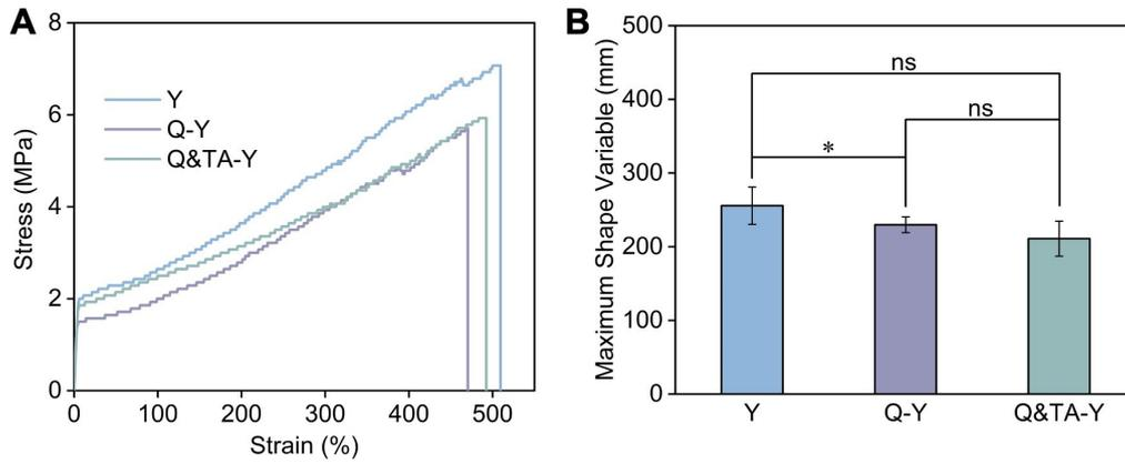
**Fig. S3** A. Representative stress-strain curves obtained by tensile testing for three groups of yarns. B. Maximum stretch of Y, Q-T, and Q&TA-Y. ns  $P > 0.05$ ,  $*P < 0.05$  compared to each group.
