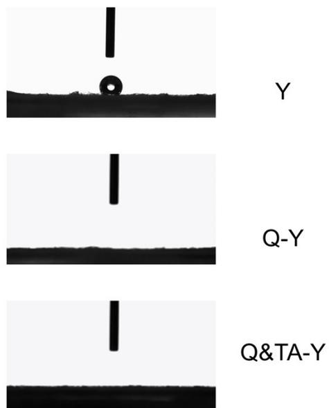
**Fig. S2** Contact angle images of Y, Q-Y, and Q&TA-Y yarns.
