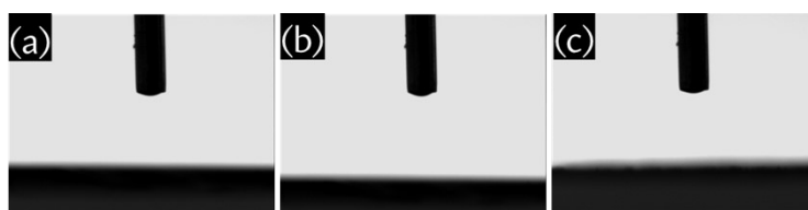
Figure S7: Water contact angle of (a) pristine, (b) annealed and (c) activated amorphous carbon nanofoams.
