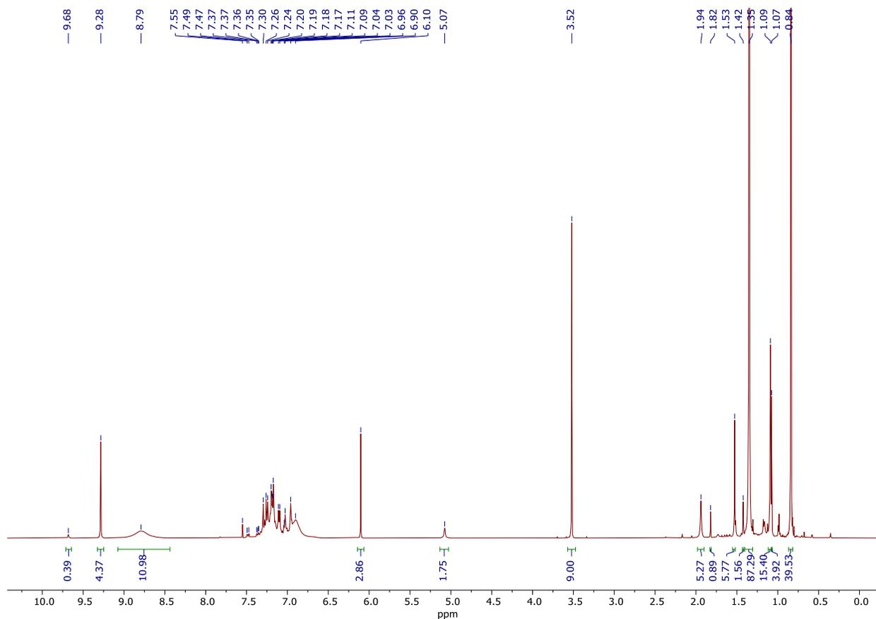
**Figure S89.**  $t = 5$  h  $^1\text{H}$  NMR spectrum of multicomponent coupling of 1-phenyl-1-propyne (1 equiv.), acetonitrile (10 equiv.), and  $\text{py}_3\text{TiCl}_2(\text{NPh})$  in  $\text{C}_6\text{D}_5\text{Br}$  after addition of pivaldehyde (1 equiv.).
