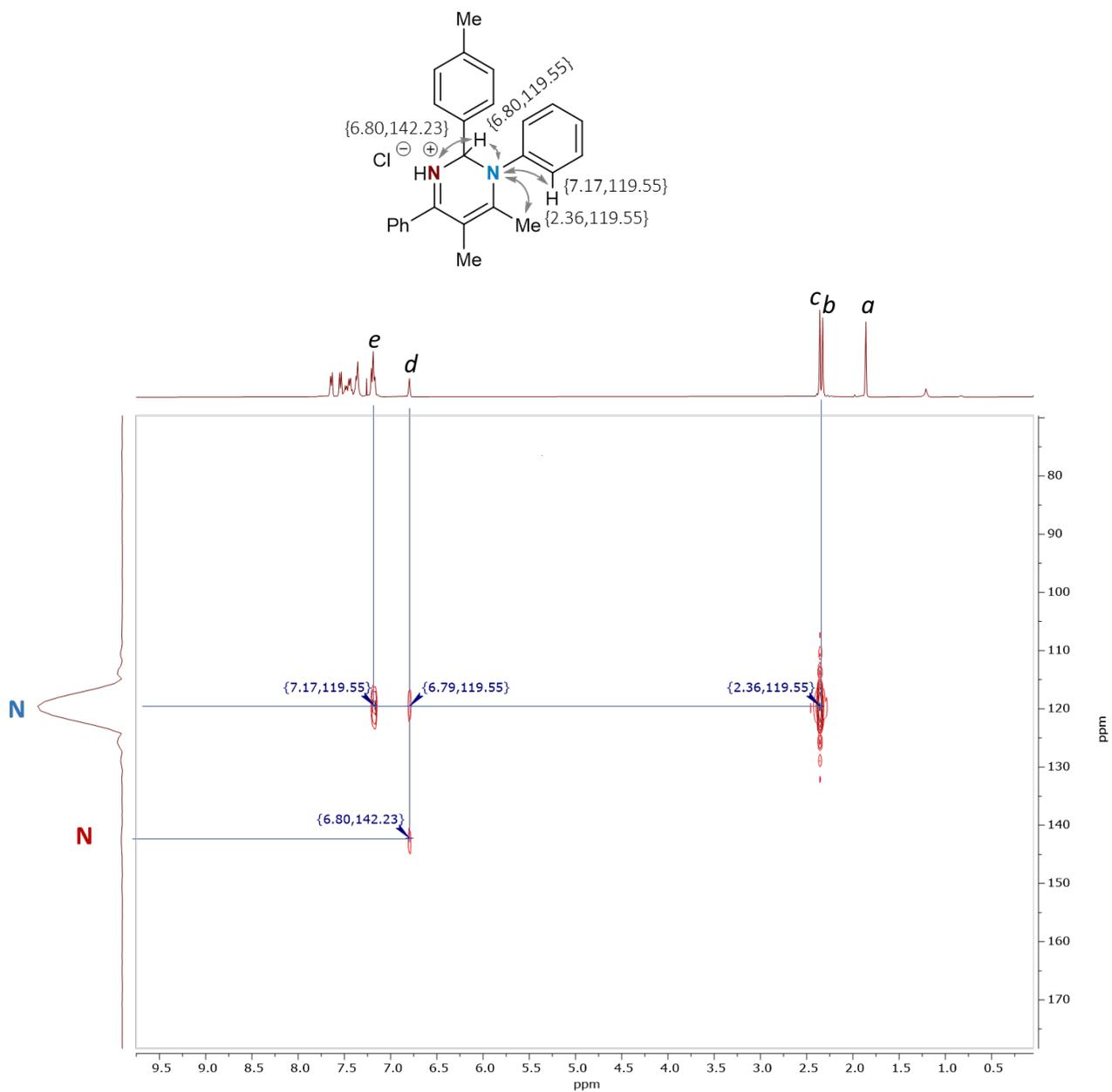
Figure S104.  $^1\text{H}$ - $^{15}\text{N}$  HMBC NMR spectrum of **5fca**•HCl in  $\text{CDCl}_3$ .
