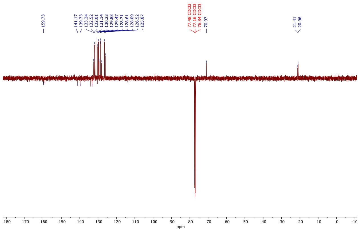
**Figure S112.**  $^{13}\text{C}\{^1\text{H}\}$  APT NMR spectrum of 1,2-dihydropyrimidine (**5aca**•HCl) in  $\text{CDCl}_3$ .
