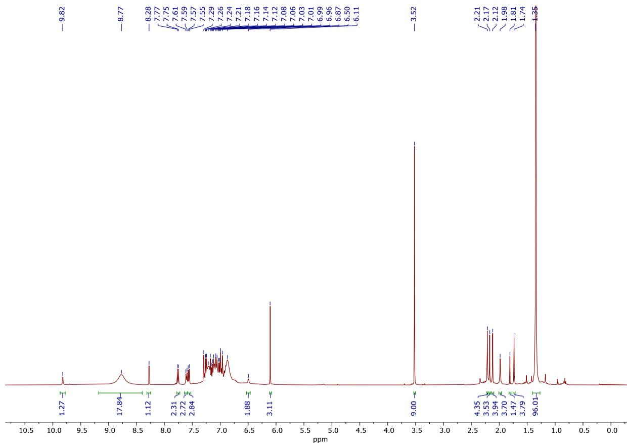
**Figure S20.**  $t = 5$  h  $^1\text{H}$  NMR spectrum of multicomponent coupling of 1-(prop-1-yn-1-yl)-4-(trifluoromethoxy)benzene (1 equiv.), acetonitrile (10 equiv.), and  $\text{py}_3\text{TiCl}_2(\text{NPh})$  in  $\text{C}_6\text{D}_5\text{Br}$  after addition of *p*-tolualdehyde (1 equiv.).
