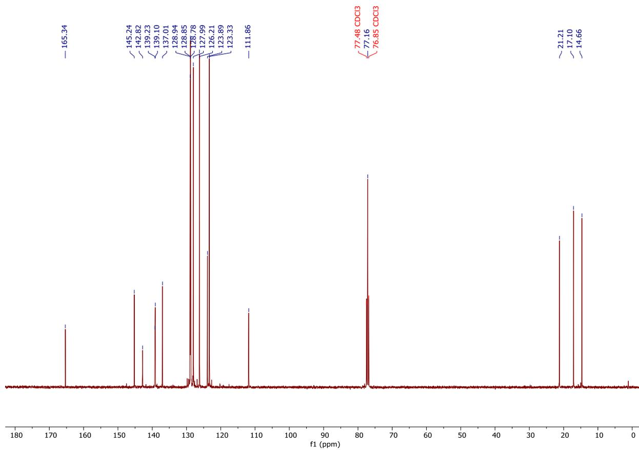
Figure S106.  $^{13}\text{C}\{^1\text{H}\}$  NMR spectrum of **5fca** in  $\text{CDCl}_3$ .
