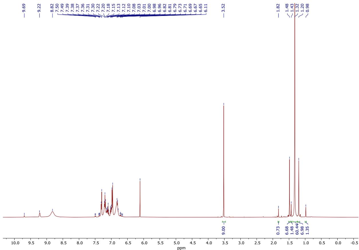
**Figure S80.**  $t = 4$  h  $^1\text{H}$  NMR spectrum of multicomponent coupling of 1-phenyl-1-propyne (1 equiv.), acetonitrile (10 equiv.), and  $\text{py}_3\text{TiCl}_2(\text{NPh})$  in  $\text{C}_6\text{D}_5\text{Br}$ .
