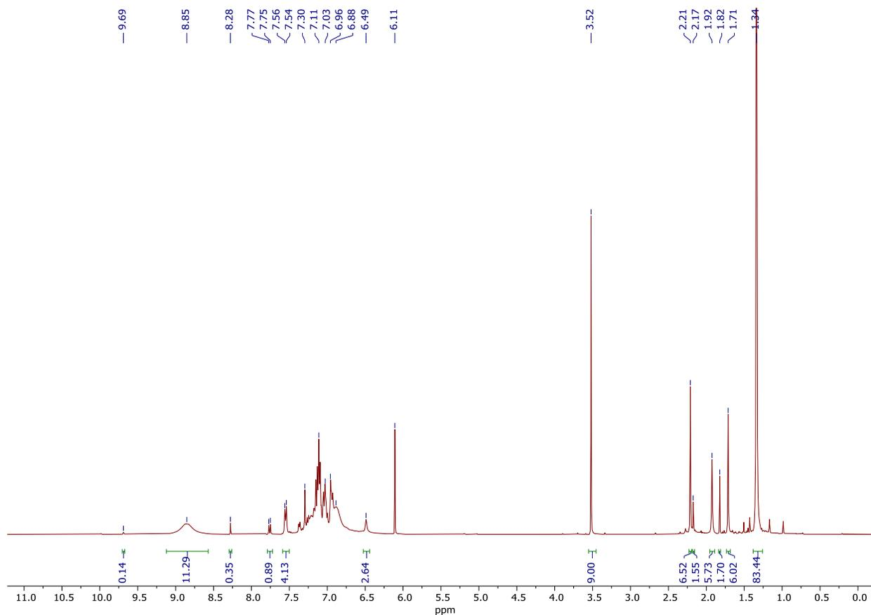
**Figure S12.**  $t = 5$  h  $^1\text{H}$  NMR spectrum of multicomponent coupling of 1-phenyl-1-propyne (1 equiv.), acetonitrile (10 equiv.), and  $\text{py}_3\text{TiCl}_2(\text{NPh})$  in  $\text{C}_6\text{D}_5\text{Br}$  after addition of *p*-tolualdehyde (1 equiv.).
