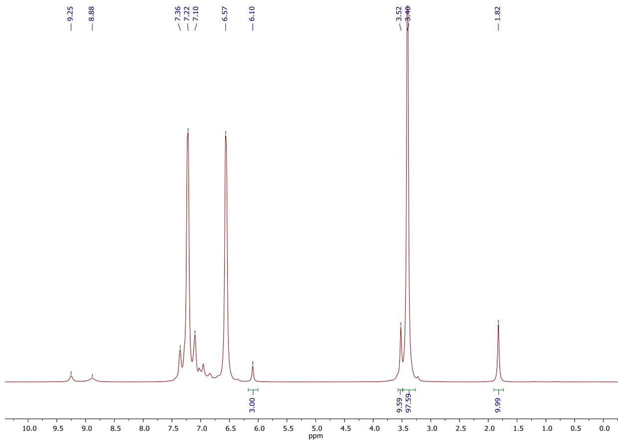
**Figure S44.**  $t = 0$  h  $^1\text{H}$  NMR spectrum of multicomponent coupling of 1-phenyl-1-propyne (1 equiv.), 4-methoxybenzotrile (10 equiv.), and  $\text{py}_3\text{TiCl}_2(\text{NPh})$  in  $\text{C}_6\text{D}_5\text{Br}$ .
