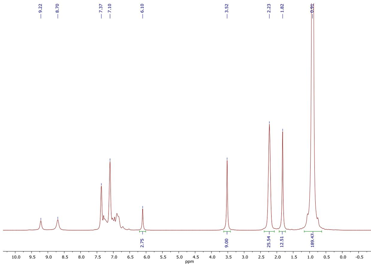
**Figure S61.**  $t = 0$  h  $^1\text{H}$  NMR spectrum of multicomponent coupling of 1-phenyl-1-propyne (1 equiv.), isobutyronitrile (10 equiv.), and  $\text{py}_3\text{TiCl}_2(\text{NPh})$  in  $\text{C}_6\text{D}_5\text{Br}$ .
