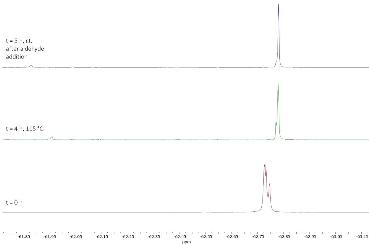
**Figure S59.** Stacked  $^{19}\text{F}$  NMR spectra characterizing the multicompound coupling of 1-phenyl-1-propyne (1 equiv.), 4-trifluoromethylbenzotrile (10 equiv.), *p*-tolualdehyde (1 equiv.), and  $\text{py}_3\text{TiCl}_2(\text{NPh})$  in  $\text{C}_6\text{D}_5\text{Br}$ ; Bottom (red trace):  $t=0$ ; Middle (green trace):  $t = 4$  h at  $115\text{ }^\circ\text{C}$ .
