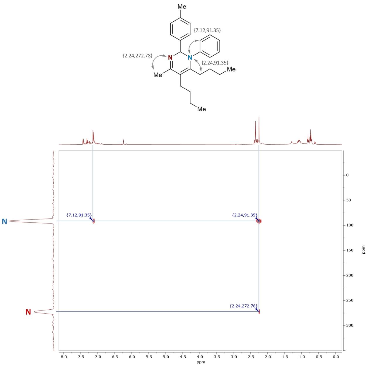
**Figure S136.**  $^1\text{H}$ - $^{15}\text{N}$  HMBC NMR spectrum of 1,2-dihydropyrimidine **5gaa** in  $\text{CDCl}_3$ .
