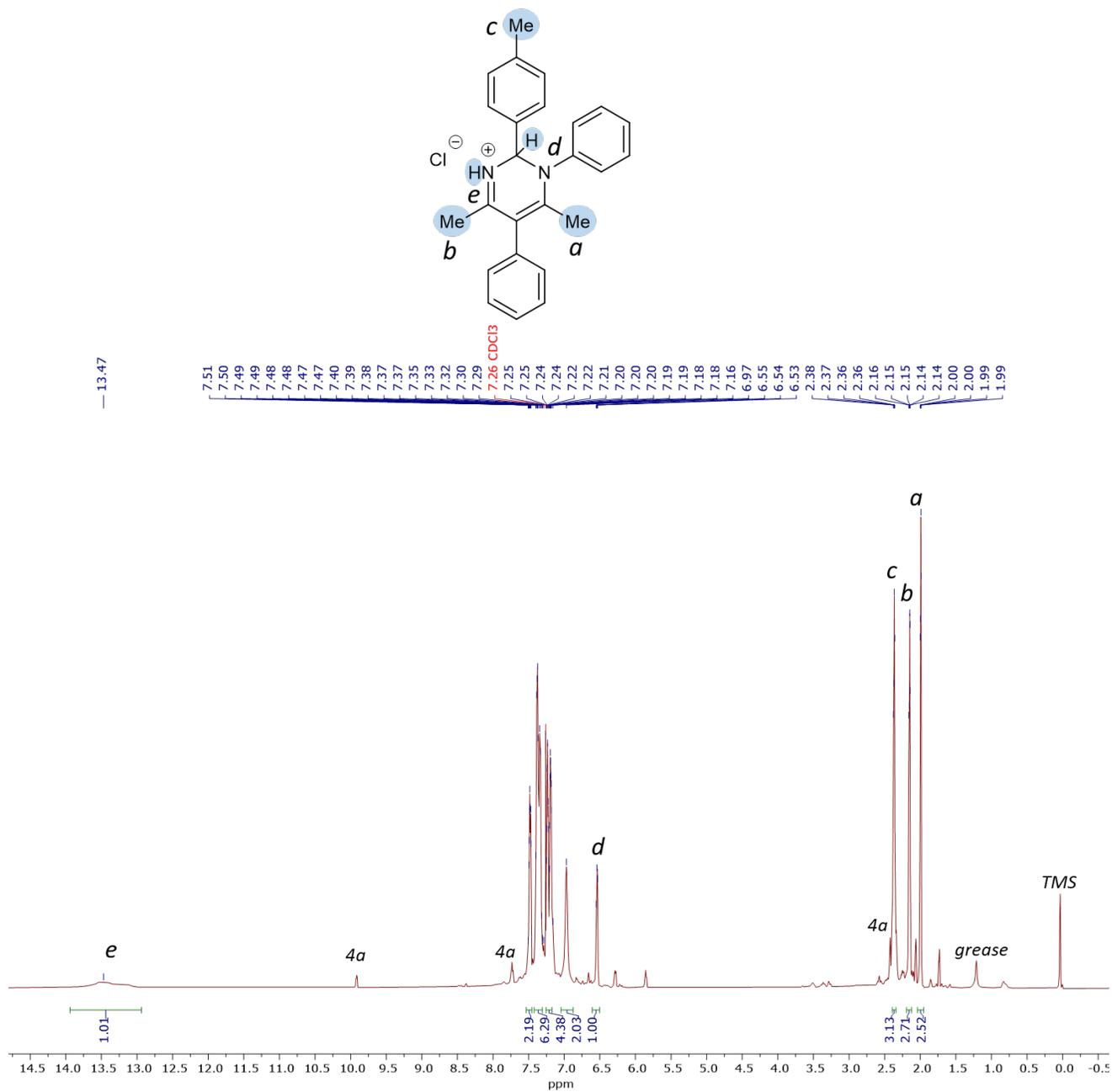
**Figure S90.** <sup>1</sup>H NMR spectrum of **5aaa**•HCl in CDCl<sub>3</sub>.
