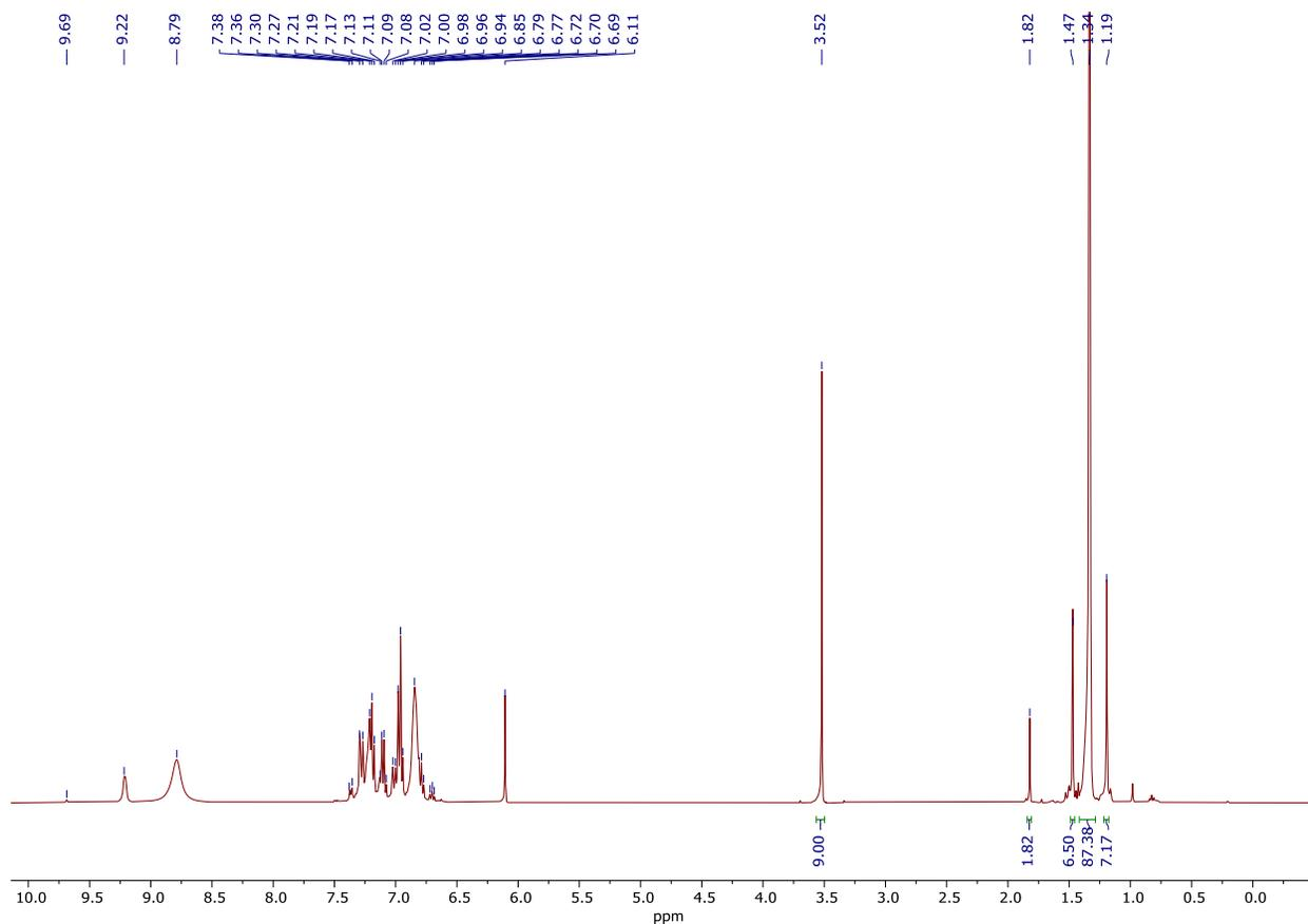
**Figure S84.**  $t = 4$  h  $^1\text{H}$  NMR spectrum of multicomponent coupling of 1-phenyl-1-propyne (1 equiv.), acetonitrile (10 equiv.), and  $\text{py}_3\text{TiCl}_2(\text{NPh})$  in  $\text{C}_6\text{D}_5\text{Br}$ .
