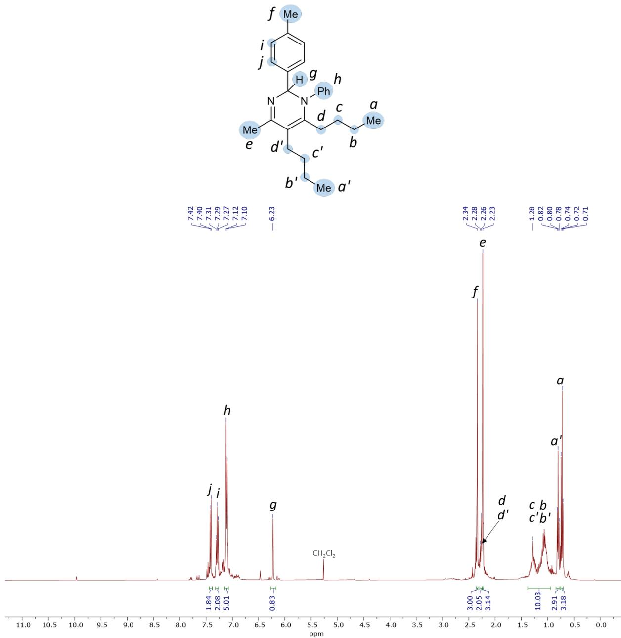
**Figure S131.** <sup>1</sup>H NMR spectrum of 1,2-dihydropyrimidine **5gaa** in CDCl<sub>3</sub>.
