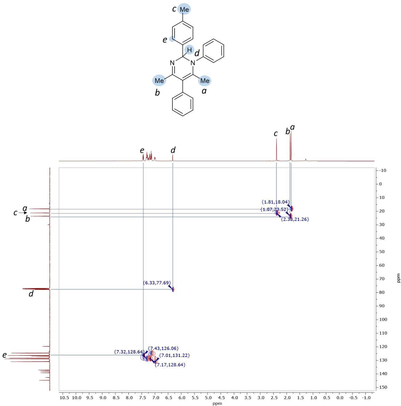
Figure S96.  $^1\text{H}$ - $^{13}\text{C}$  HSQC NMR spectrum of 1,2-dihydropyrimidine **5aaa** in  $\text{CDCl}_3$ .
