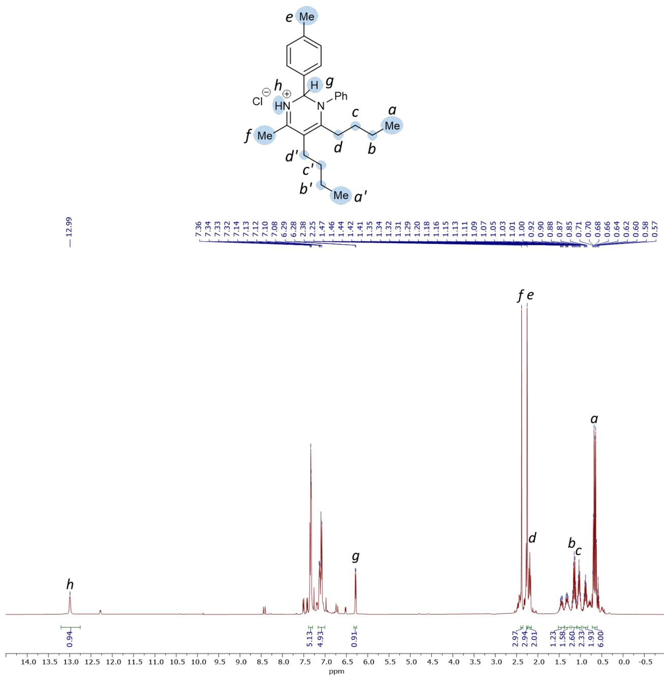
Figure S123. <sup>1</sup>H NMR spectrum of 5gaa•HCl in CDCl<sub>3</sub>.
