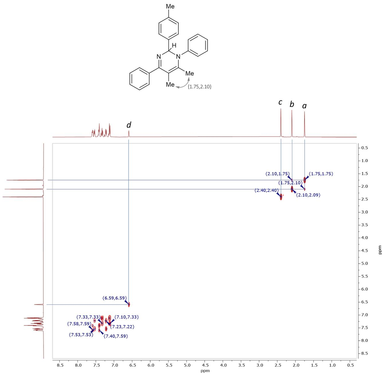
**Figure S107.**  $^1\text{H}$ - $^1\text{H}$  COSY NMR spectrum of **5fca** in  $\text{CDCl}_3$ .
