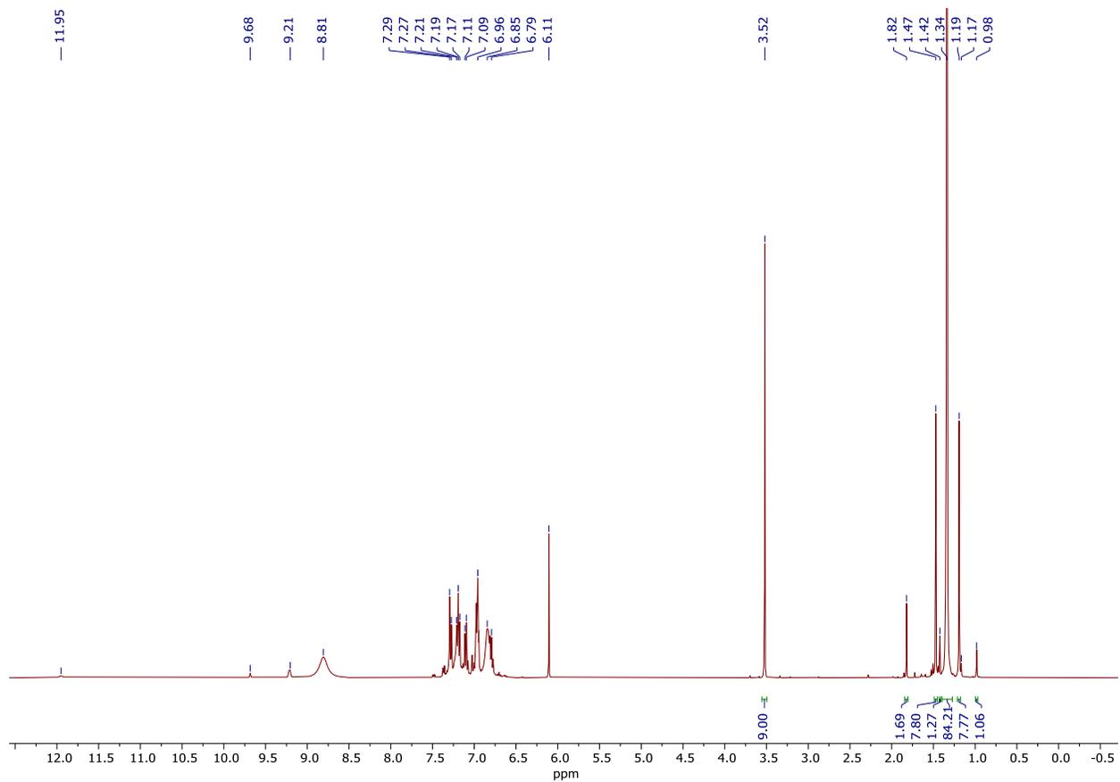
**Figure S11.**  $t = 4$  h  $^1\text{H}$  NMR spectrum of multicomponent coupling of 1-phenyl-1-propyne (1 equiv.), acetonitrile (10 equiv.), and  $\text{py}_3\text{TiCl}_2(\text{NPh})$  in  $\text{C}_6\text{D}_5\text{Br}$ .
