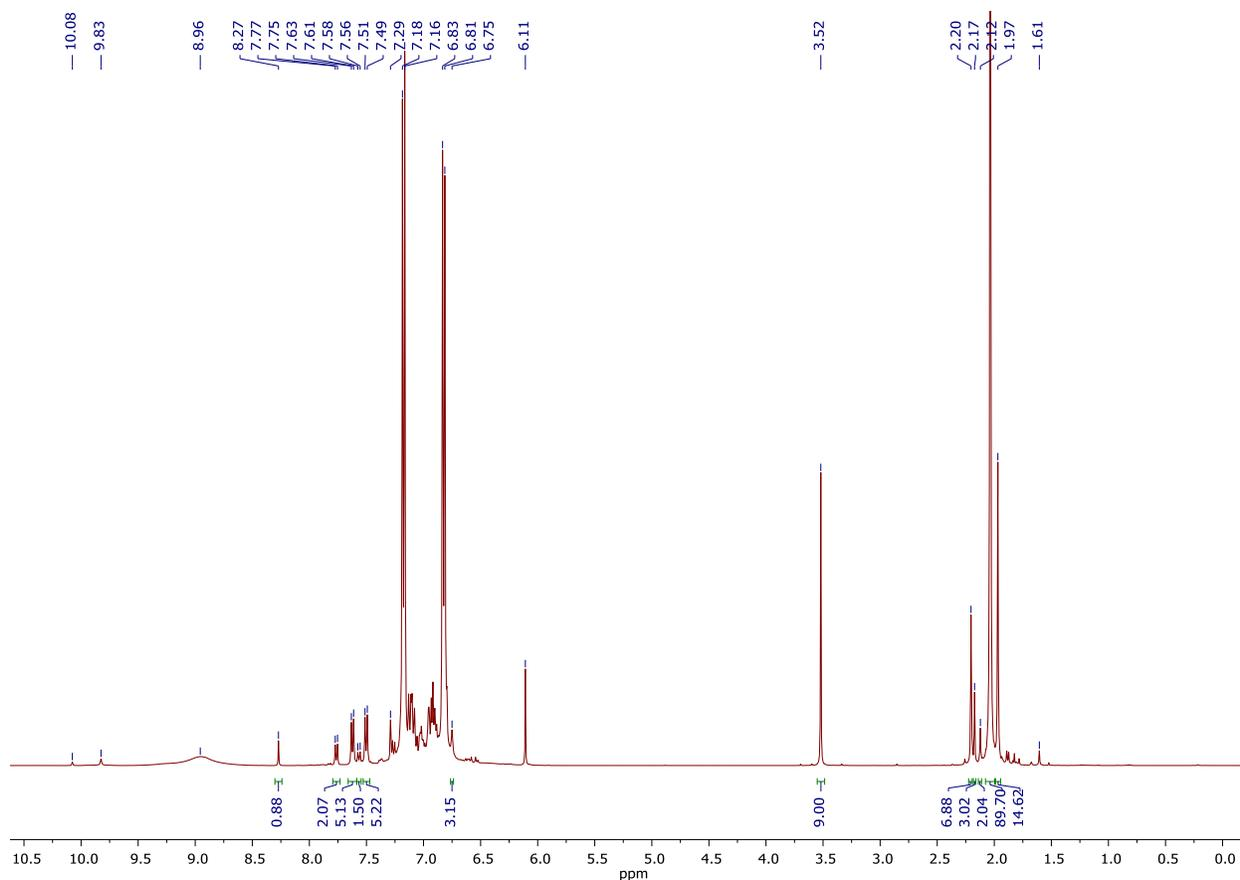
**Figure S54.**  $t = 5$  h  $^1\text{H}$  NMR spectrum of multicomponent coupling of 1-phenyl-1-propyne (1 equiv.), *p*-tolunitrile (10 equiv.), and  $\text{py}_3\text{TiCl}_2(\text{NPh})$  in  $\text{C}_6\text{D}_5\text{Br}$  after addition of *p*-tolualdehyde (1 equiv.).
