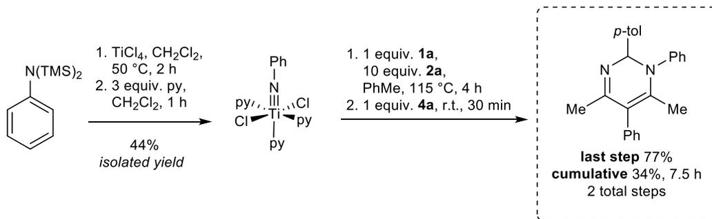
**Figure S142.** Synthetic route to 1,2-dihydropyrimidine (**5aaa**) over three steps beginning with the synthesis of the  $\text{py}_3\text{TiCl}_2(\text{NPh})$
