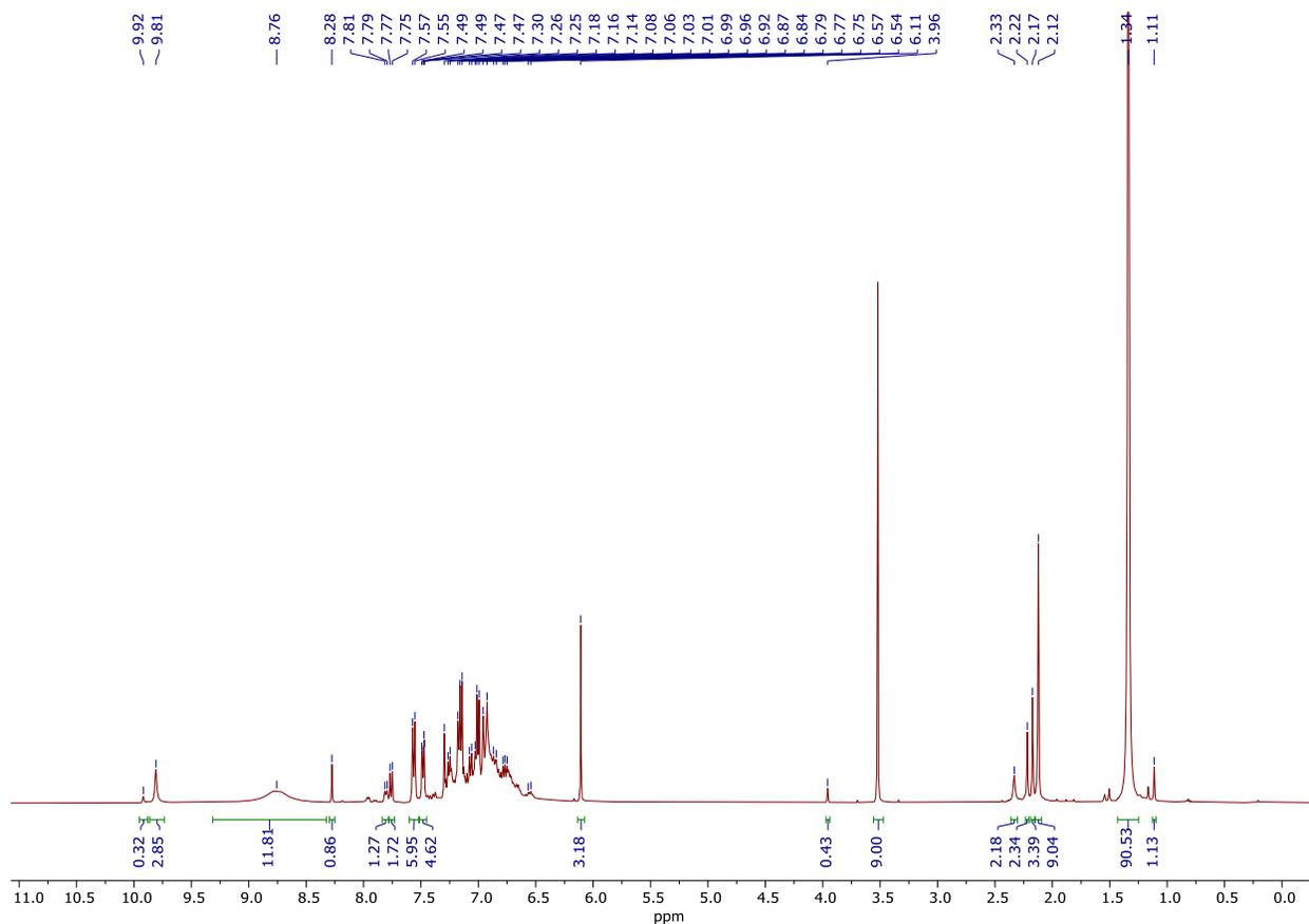
**Figure S30.**  $t = 5$  h  $^1\text{H}$  NMR spectrum of multicomponent coupling of diphenylacetylene (1 equiv.), acetonitrile (10 equiv.), and  $\text{py}_3\text{TiCl}_2(\text{NPh})$  in  $\text{C}_6\text{D}_5\text{Br}$  after addition of  $p$ -tolualdehyde (1 equiv.).
