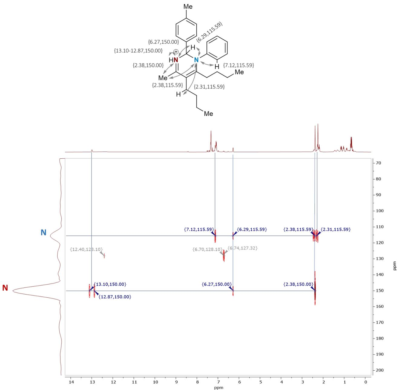
**Figure S130.**  $^1\text{H}$ - $^{15}\text{N}$  HMBC NMR spectrum of **5gaa**•HCl in  $\text{CDCl}_3$ .
