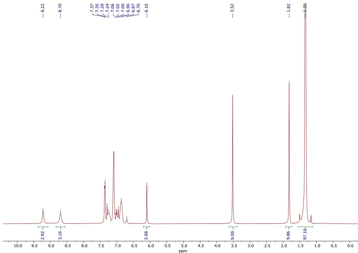
**Figure S69.**  $t = 0$  h  $^1\text{H}$  NMR spectrum of multicomponent coupling of 1-phenyl-1-propyne (1 equiv.), acetonitrile (10 equiv.), and  $\text{py}_3\text{TiCl}_2(\text{NPh})$  in  $\text{C}_6\text{D}_5\text{Br}$ .
