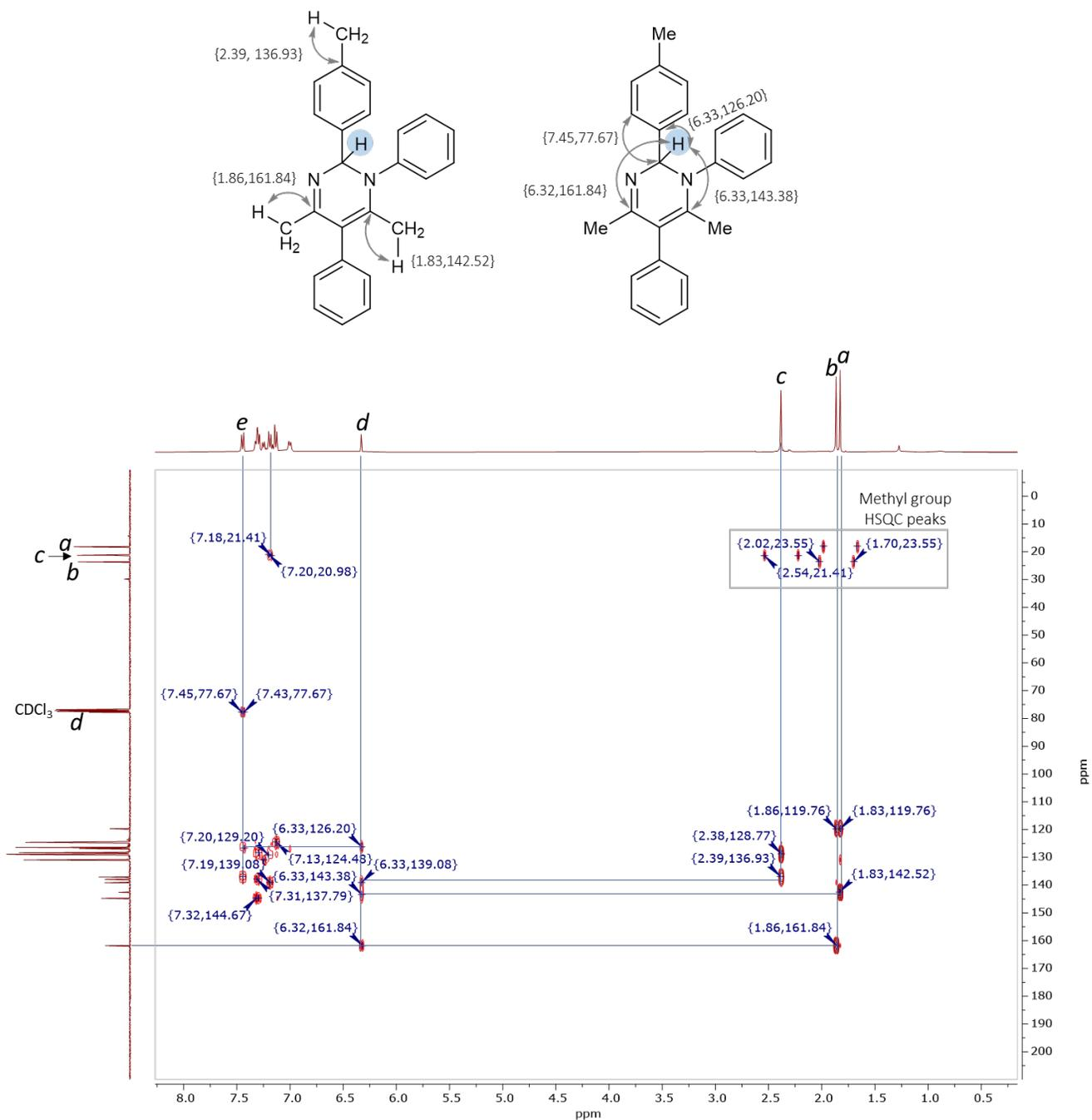
Figure S97.  $^1\text{H}$ - $^{13}\text{C}$  HMBC NMR spectrum of 1,2-dihydropyrimidine **5aaa** in  $\text{CDCl}_3$ .
