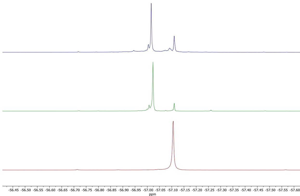
**Figure S21.** Stacked  $^{19}\text{F}$  NMR spectra characterizing the multicomponent coupling of 1-(prop-1-yn-1-yl)-4-(trifluoromethoxy)benzene (1 equiv.), acetonitrile (10 equiv.), *p*-tolualdehyde (1 equiv.), and  $\text{py}_3\text{TiCl}_2(\text{NPh})$  in  $\text{C}_6\text{D}_5\text{Br}$ ; Bottom (red trace):  $t=0$ ; Middle (green trace):  $t = 4$  h at  $115^\circ\text{C}$ .
