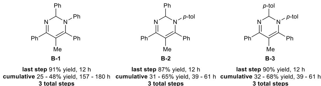
**Figure S139.** Comparison of the final step's yields and reaction time with the cumulative yields and reaction times for three 1,2-dihydropyrimidines in the literature
