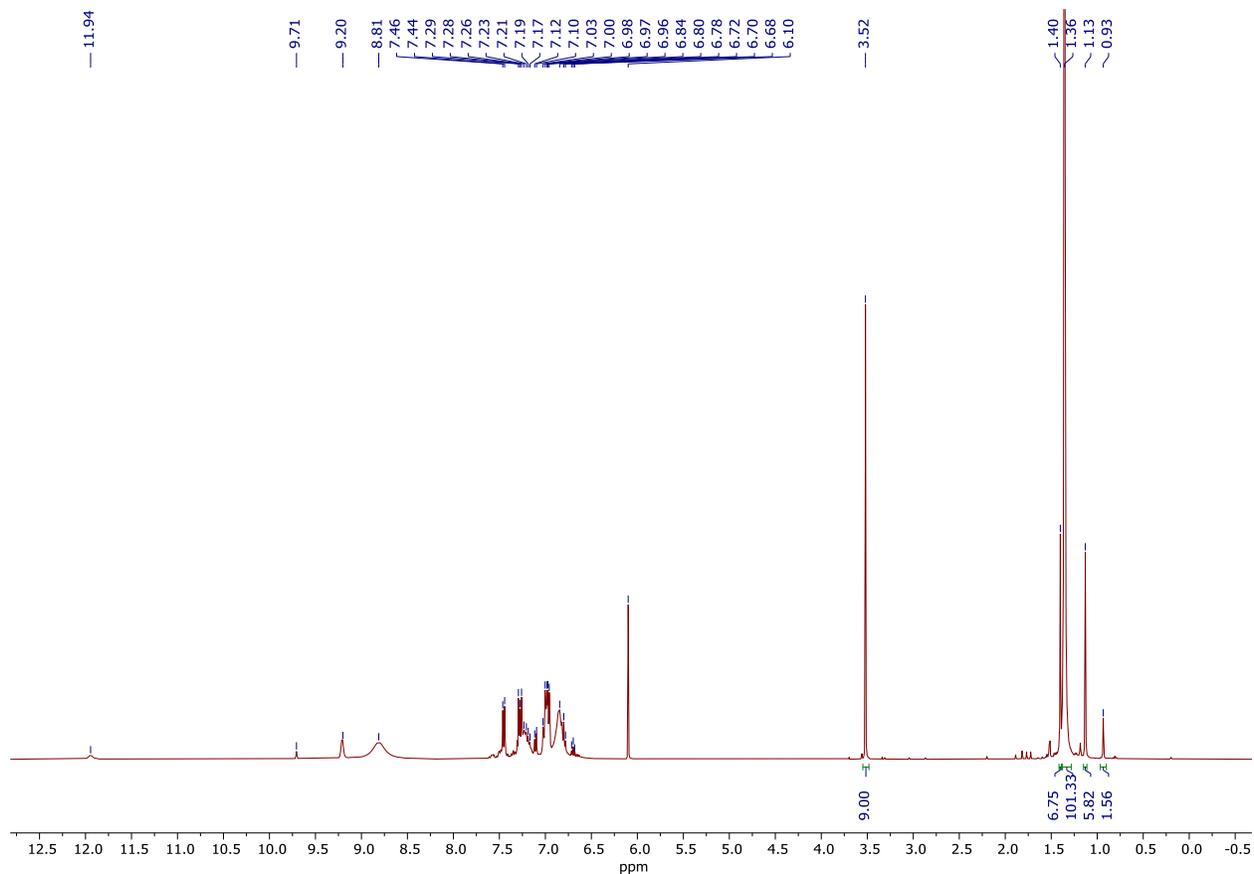
**Figure S24.**  $t = 4$  h  $^1\text{H}$  NMR spectrum of multicomponent coupling of 1-(prop-1-yn-1-yl)-4-(trifluoromethyl)benzene (1 equiv.), acetonitrile (10 equiv.), and  $\text{py}_3\text{TiCl}_2(\text{NPh})$  in  $\text{C}_6\text{D}_5\text{Br}$ .
