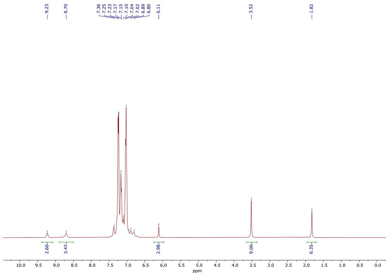
**Figure S48.**  $t = 0$  h  $^1\text{H}$  NMR spectrum of multicomponent coupling of 1-phenyl-1-propyne (1 equiv.), benzonitrile (10 equiv.), and  $\text{py}_3\text{TiCl}_2(\text{NPh})$  in  $\text{C}_6\text{D}_5\text{Br}$ .
