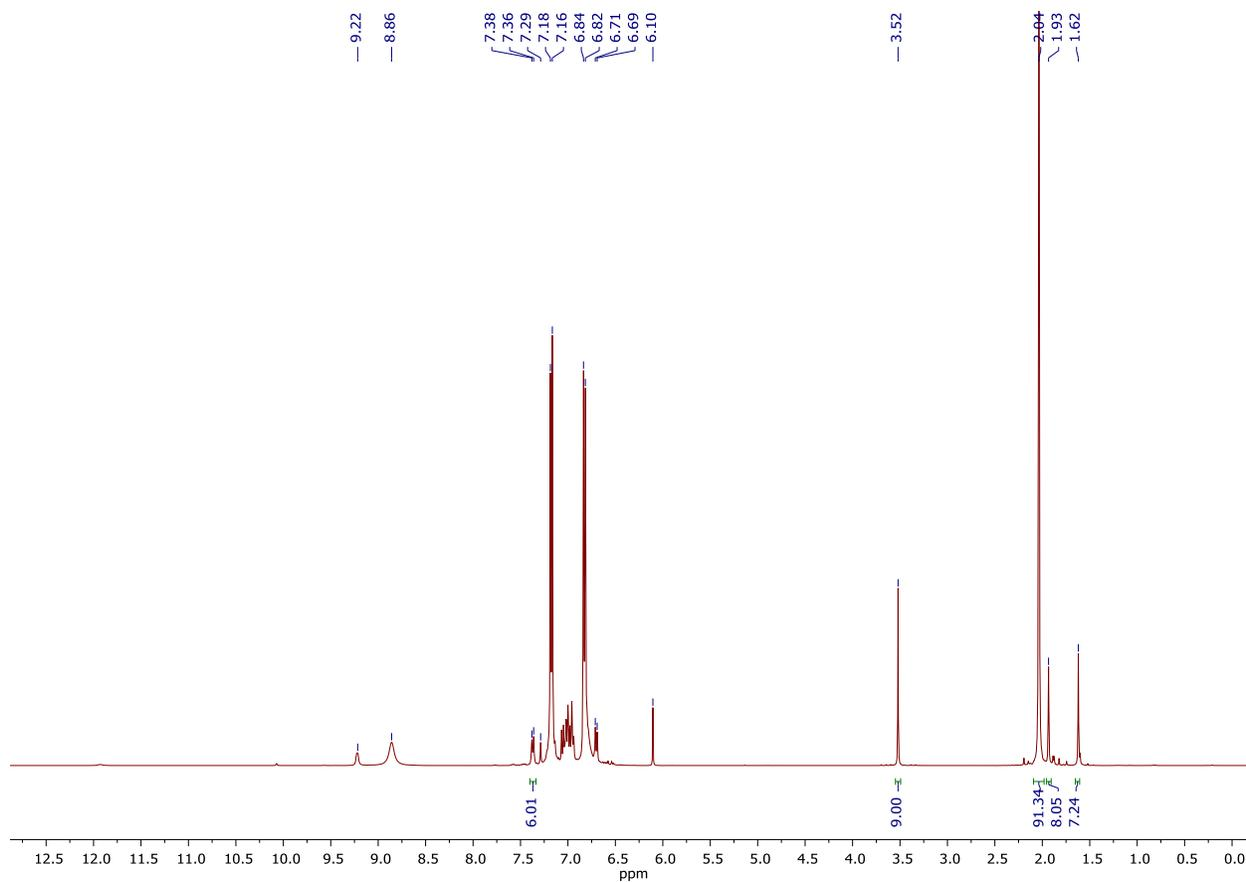
**Figure S53.**  $t = 4$  h  $^1\text{H}$  NMR spectrum of multicomponent coupling of 1-phenyl-1-propyne (1 equiv.), *p*-tolunitrile (10 equiv.), and  $\text{py}_3\text{TiCl}_2(\text{NPh})$  in  $\text{C}_6\text{D}_5\text{Br}$ .
