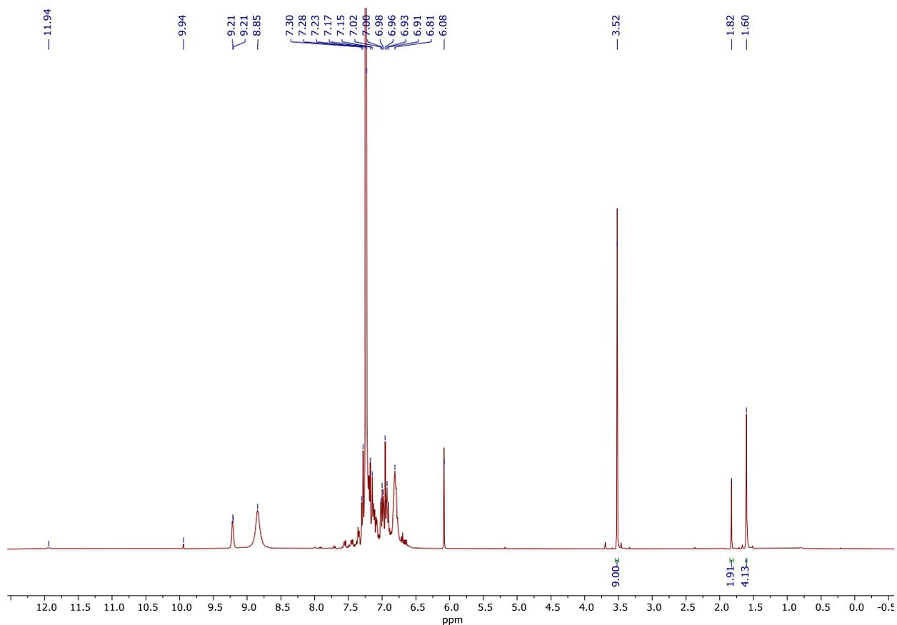
**Figure S57.**  $t = 4$  h  $^1\text{H}$  NMR spectrum of multicomponent coupling of 1-phenyl-1-propyne (1 equiv.), 4-trifluoromethylbenzotrile (10 equiv.), and  $\text{py}_3\text{TiCl}_2(\text{NPh})$  in  $\text{C}_6\text{D}_5\text{Br}$ .
