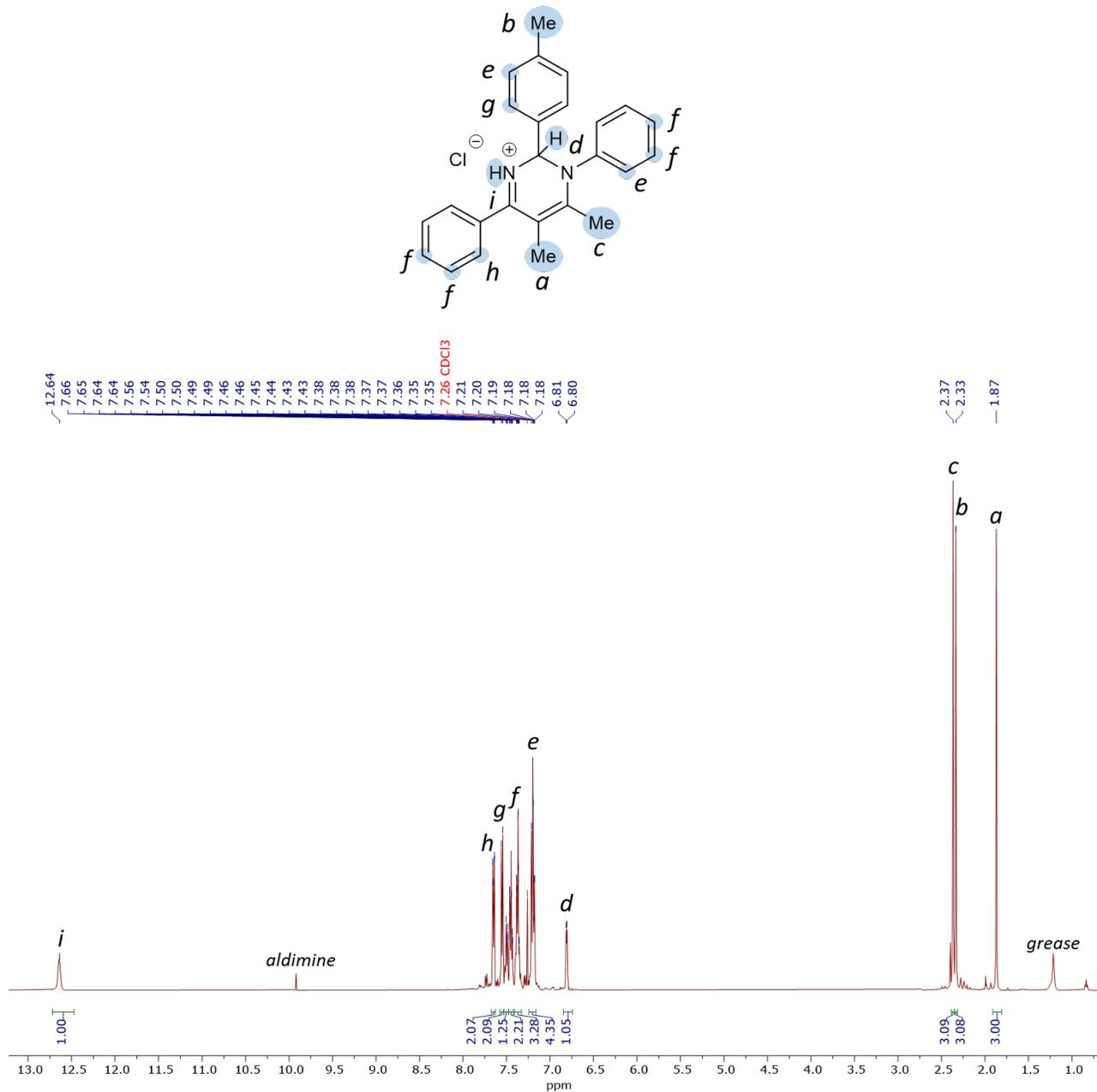
Figure S99. <sup>1</sup>H NMR spectrum of 5fca•HCl in CDCl<sub>3</sub>.
