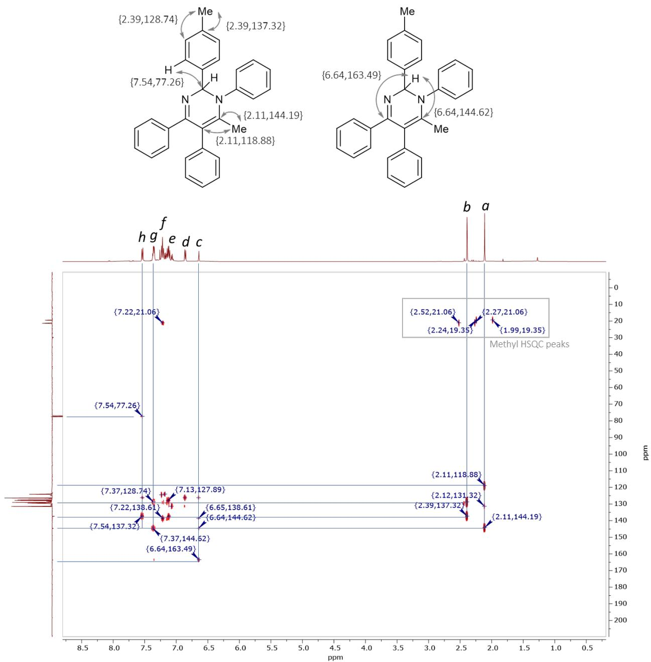
Figure S121.  $^1\text{H}$ - $^{13}\text{C}$  HMBC NMR spectrum of 1,2-dihydropyrimidine **5aca** in  $\text{CDCl}_3$ .
