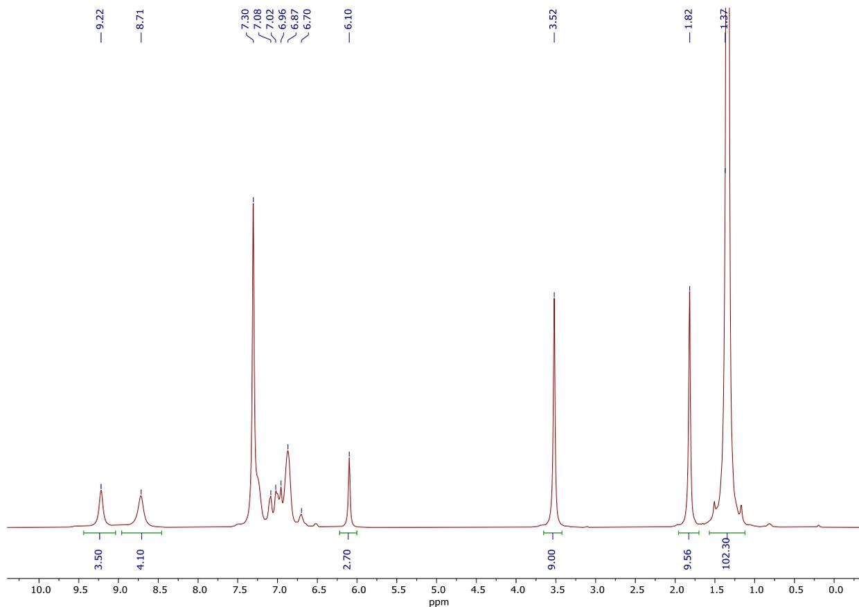
**Figure S23.**  $t = 0$  h  $^1\text{H}$  NMR spectrum of multicomponent coupling of 1-(prop-1-yn-1-yl)-4-(trifluoromethyl)benzene (1 equiv.), acetonitrile (10 equiv.), and  $\text{py}_3\text{TiCl}_2(\text{NPh})$  in  $\text{C}_6\text{D}_5\text{Br}$ .
