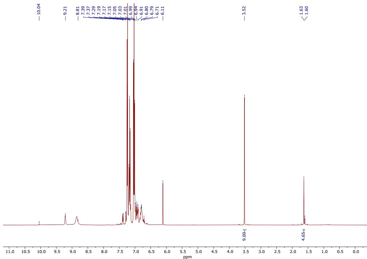
**Figure S49.**  $t = 4$  h  $^1\text{H}$  NMR spectrum of multicomponent coupling of 1-phenyl-1-propyne (1 equiv.), benzonitrile (10 equiv.), and  $\text{py}_3\text{TiCl}_2(\text{NPh})$  in  $\text{C}_6\text{D}_5\text{Br}$ .
