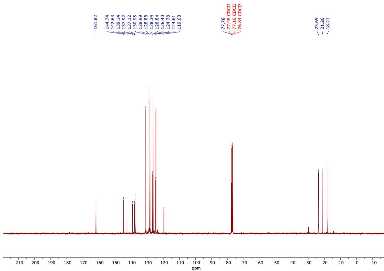
Figure S94.  $^{13}\text{C}\{^1\text{H}\}$  NMR spectrum of 1,2-dihydropyrimidine **5aaa** in  $\text{CDCl}_3$ .
