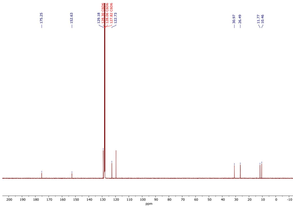
**Figure S2.**  $^{13}\text{C}\{^1\text{H}\}$  NMR spectrum of *N*-phenylpentan-3-imine in  $\text{C}_6\text{D}_6$ .
