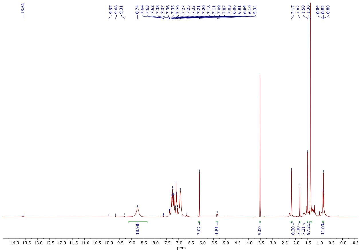
**Figure S85.**  $t = 5$  h  $^1\text{H}$  NMR spectrum of multicomponent coupling of 1-phenyl-1-propyne (1 equiv.), acetonitrile (10 equiv.), and  $\text{py}_3\text{TiCl}_2(\text{NPh})$  in  $\text{C}_6\text{D}_5\text{Br}$  after addition of valeraldehyde (1 equiv.).
