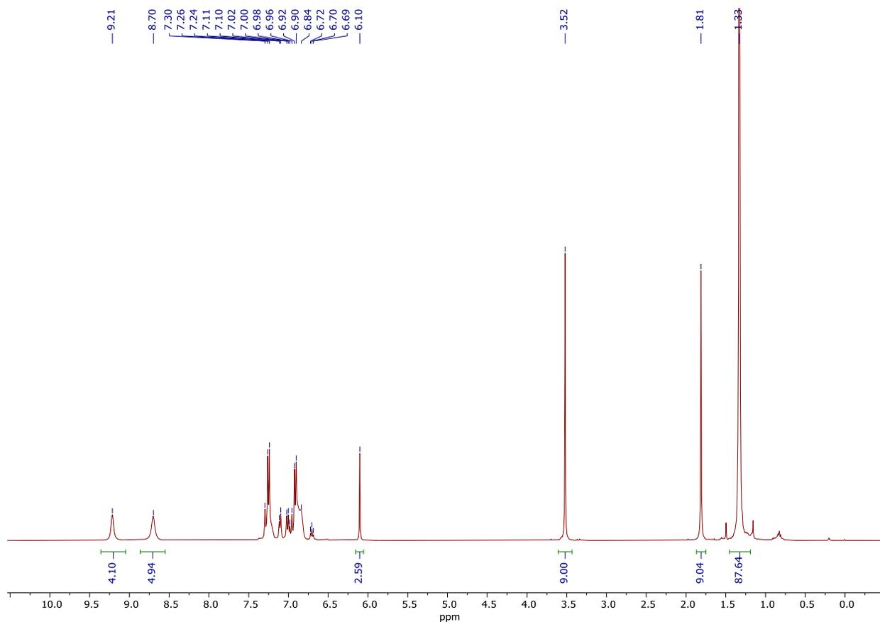
**Figure S18.**  $t = 0$  h  $^1\text{H}$  NMR spectrum of multicomponent coupling of 1-(prop-1-yn-1-yl)-4-(trifluoromethoxy)benzene (1 equiv.), acetonitrile (10 equiv.), and  $\text{py}_3\text{TiCl}_2(\text{NPh})$  in  $\text{C}_6\text{D}_5\text{Br}$ .
