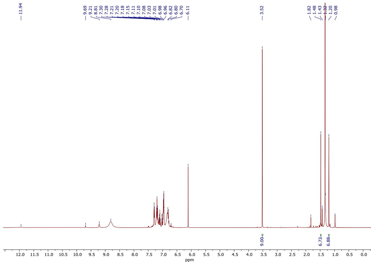
**Figure S70.**  $t = 4$  h  $^1\text{H}$  NMR spectrum of multicomponent coupling of 1-phenyl-1-propyne (1 equiv.), acetonitrile (10 equiv.), and  $\text{py}_3\text{TiCl}_2(\text{NPh})$  in  $\text{C}_6\text{D}_5\text{Br}$ .
