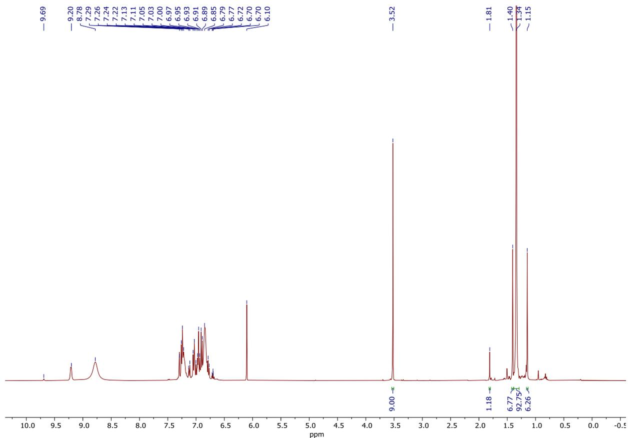
**Figure S19.**  $t = 4$  h  $^1\text{H}$  NMR spectrum of multicomponent coupling of 1-(prop-1-yn-1-yl)-4-(trifluoromethoxy)benzene (1 equiv.), acetonitrile (10 equiv.), and  $\text{py}_3\text{TiCl}_2(\text{NPh})$  in  $\text{C}_6\text{D}_5\text{Br}$ .
