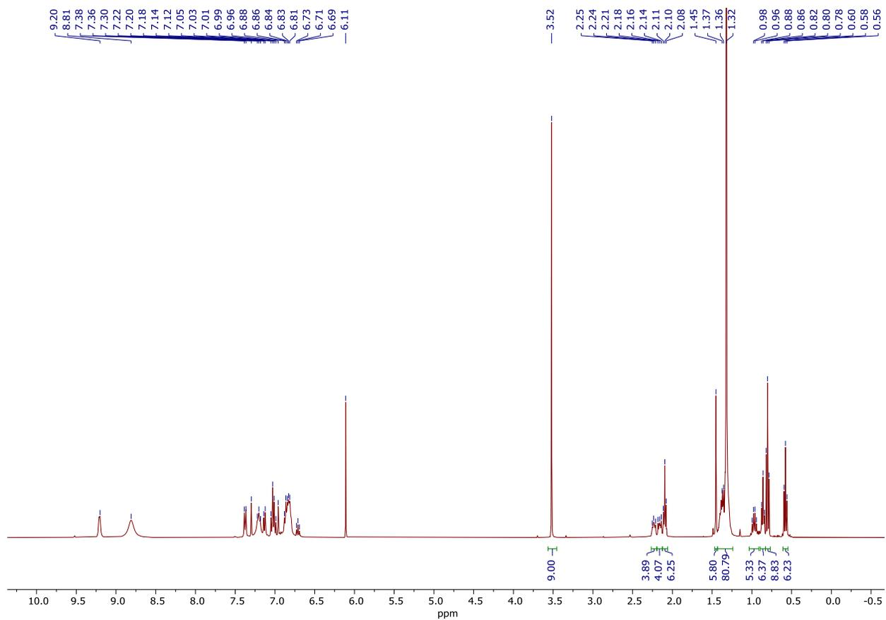
**Figure S41.**  $t = 4$  h  $^1\text{H}$  NMR spectrum of multicomponent coupling of 5-decyne (1 equiv.), acetonitrile (10 equiv.), and  $\text{py}_3\text{TiCl}_2(\text{NPh})$  in  $\text{C}_6\text{D}_5\text{Br}$ .
