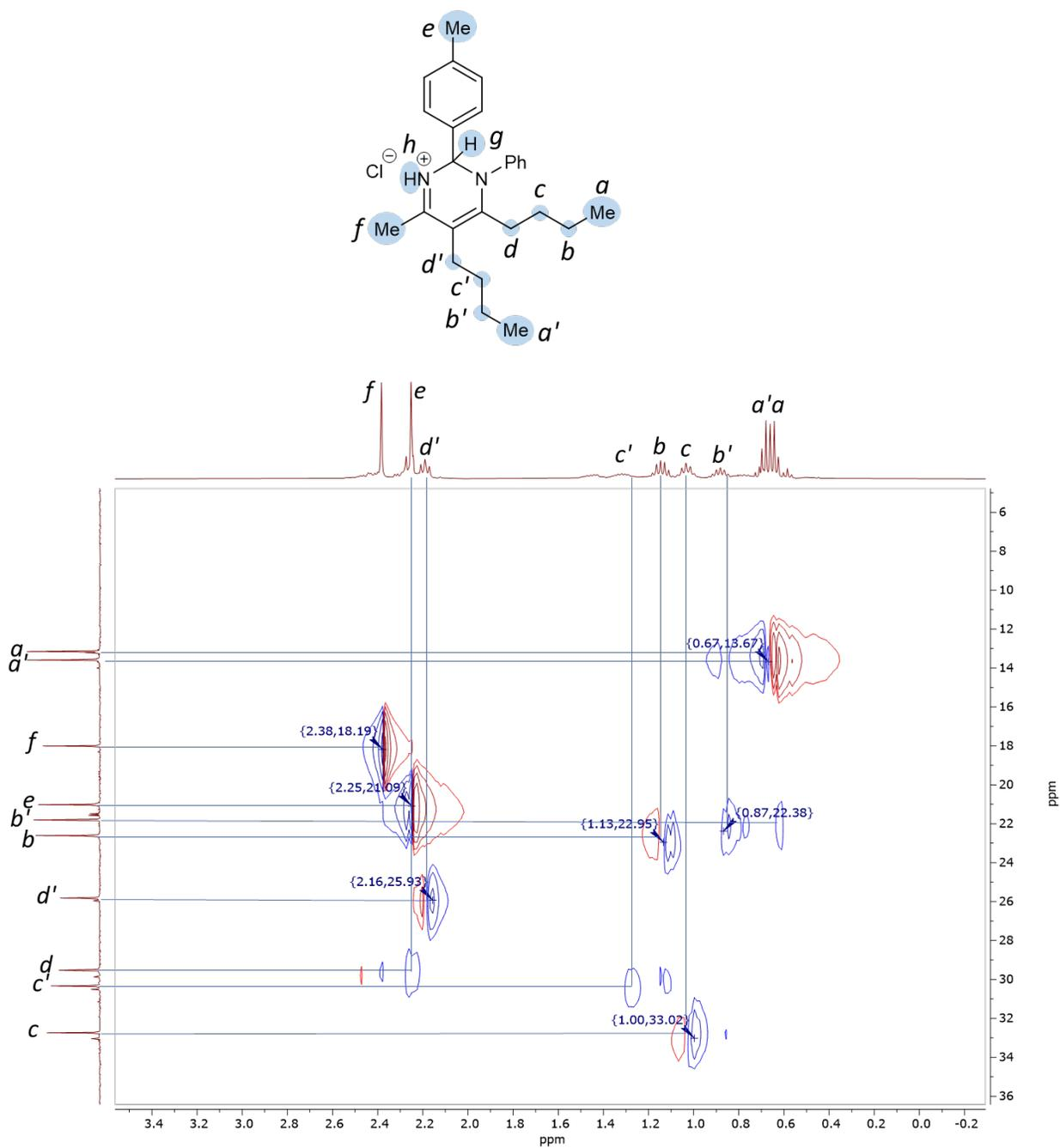
**Figure S127.** Zoomed in  $^1\text{H}$ - $^{13}\text{C}$  HSQC spectrum of **5gaa**•HCl in  $\text{CDCl}_3$ .
