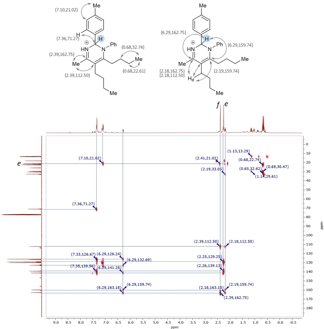
Figure S128.  $^1\text{H}$ - $^{13}\text{C}$  HMBC NMR spectrum of **5gaa**•HCl in  $\text{CDCl}_3$ .
