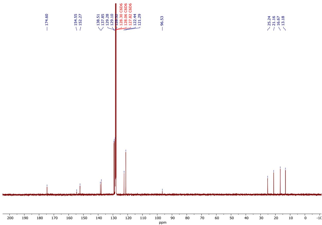
**Figure S4.**  $^{13}\text{C}\{^1\text{H}\}$  NMR spectrum of 2-methyl-3-(phenylimino)-1-(p-tolyl)pent-1-en-1-amine in  $\text{C}_6\text{D}_6$ .
