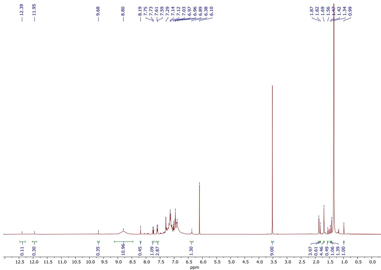
**Figure S71.**  $t = 5$  h  $^1\text{H}$  NMR spectrum of multicomponent coupling of 1-phenyl-1-propyne (1 equiv.), acetonitrile (10 equiv.), and  $\text{py}_3\text{TiCl}_2(\text{NPh})$  in  $\text{C}_6\text{D}_5\text{Br}$  after addition of 4-trifluoromethoxybenzaldehyde (1 equiv.).
