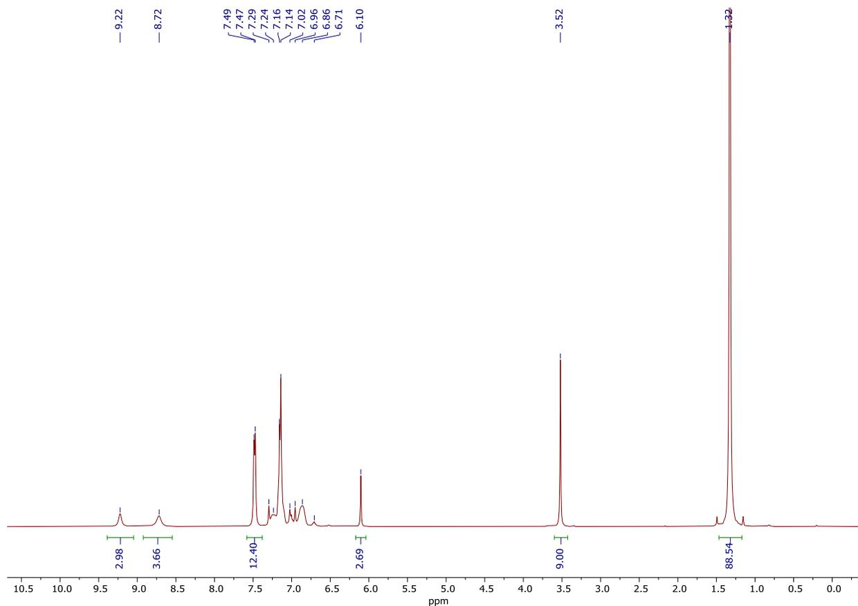
**Figure S28.**  $t = 0$  h  $^1\text{H}$  NMR spectrum of multicomponent coupling of diphenylacetylene (1 equiv.), acetonitrile (10 equiv.), and  $\text{py}_3\text{TiCl}_2(\text{NPh})$  in  $\text{C}_6\text{D}_5\text{Br}$ .
