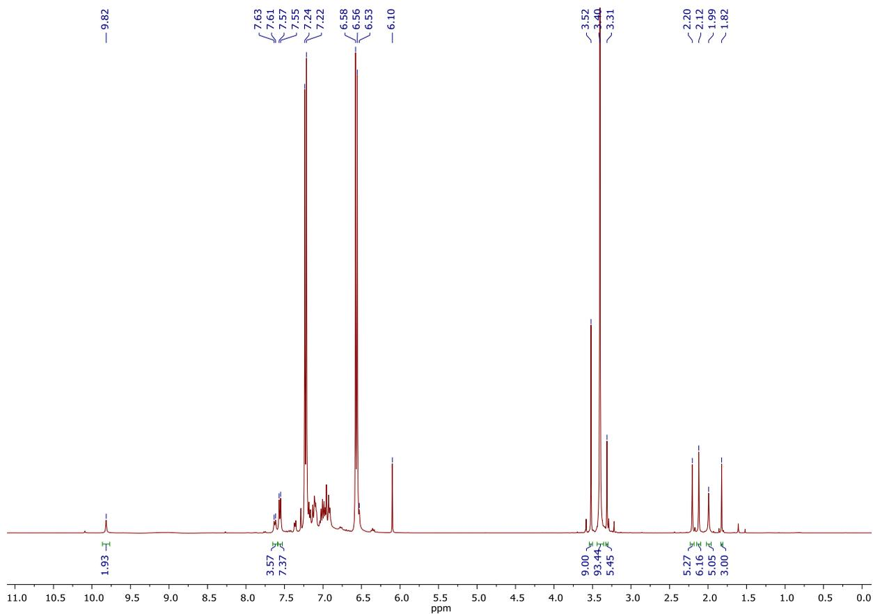
**Figure S46.**  $t = 5$  h  $^1\text{H}$  NMR spectrum of multicomponent coupling of 1-phenyl-1-propyne (1 equiv.), 4-methoxybenzotrile (10 equiv.), and  $\text{py}_3\text{TiCl}_2(\text{NPh})$  in  $\text{C}_6\text{D}_5\text{Br}$  after addition of *p*-tolualdehyde (1 equiv.).
