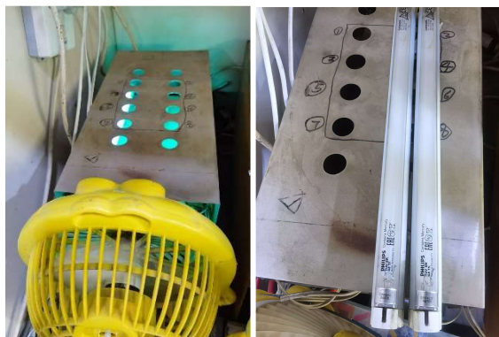
Figure S2. Photochemical reaction setup under 254 nm conditions. Physical object picture of the 254 nm setup with cooling fan (Left) and lamps (right).
