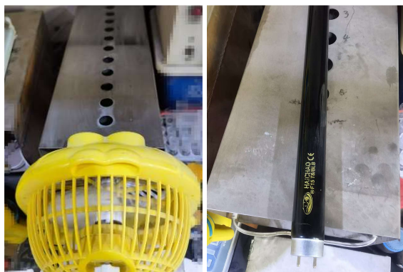
Figure S3. Photochemical reaction setup under 365 nm conditions. Physical object picture of the 365 nm setup with cooling fan (Left) and lamps (right).
