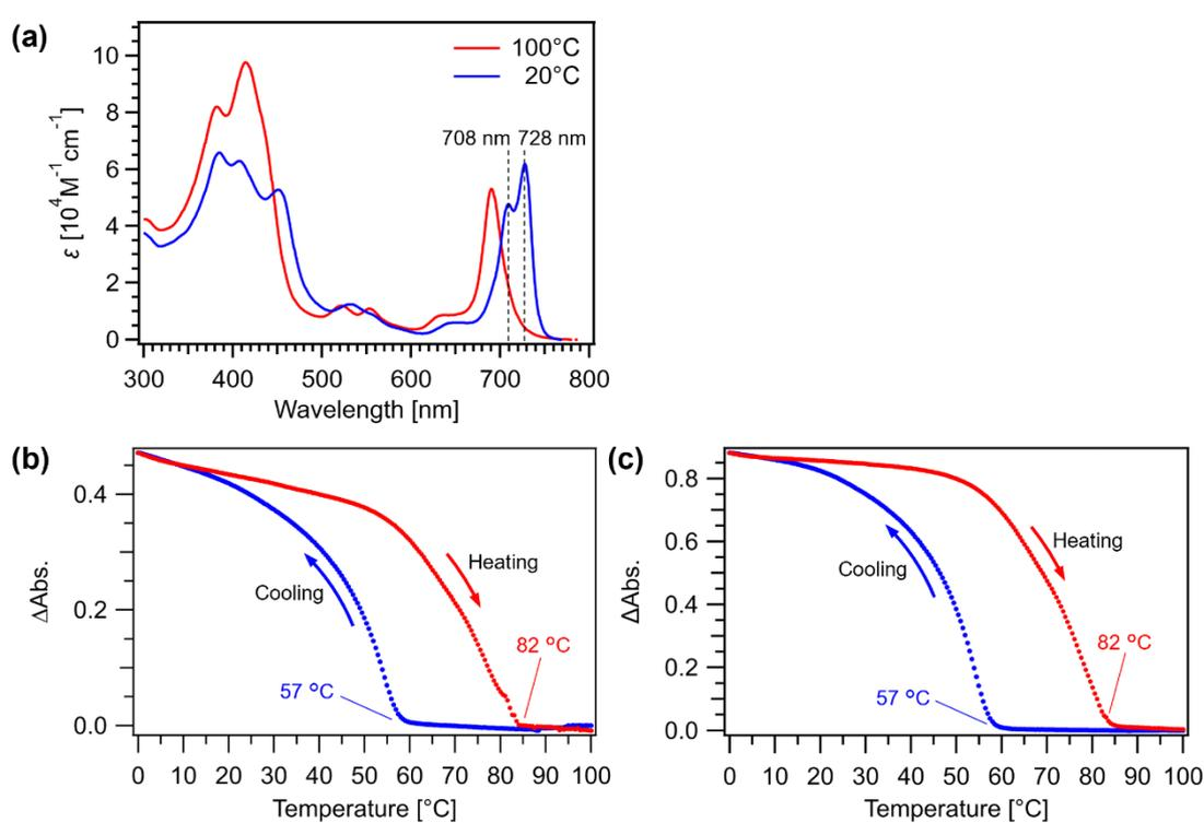
**Figure S1.** (a) UV/Vis absorption spectra of **Chl<sub>d</sub>** at 100 °C (red) and 20 °C (blue) during cooling a solution ( $c = 100 \mu\text{M}$ ) in MCH from 100 °C (red) to 20 °C (blue) at a rate of  $1 \text{ }^\circ\text{C min}^{-1}$ . (b,c) Cooling (blue) and heating (red) curves of **Chl<sub>d</sub>** obtained by plotting change in the absorption at 708 (b) and 728 nm (c) as a function of temperature.
