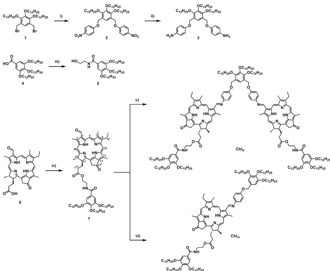
**Scheme S1.** Synthesis of **Chl<sub>d</sub>** and **Chl<sub>m</sub>**. Reagents and conditions: i) 4-nitrophenol,  $K_2CO_3$ , DMF, 70 °C; ii) zinc powder,  $CH_2Cl_2$ /AcOH, r.t.; iii) 2-aminoethanol, 1-(3-dimethylaminopropyl)-3-ethylcarbodiimide hydrochloride (EDC·HCl), *N,N'*-dimethyl-4-aminopyridine (DMAP),  $CH_2Cl_2$ , r.t.; iv) **5**, EDC·HCl, DMAP,  $CH_2Cl_2$ , r.t.; v) **3**,  $CH_2Cl_2$ /EtOH, 70 °C; vi) 4-((3,4,5-tris(dodecyloxy)benzyl)oxy)aniline,  $CH_2Cl_2$ /EtOH, 70 °C.
