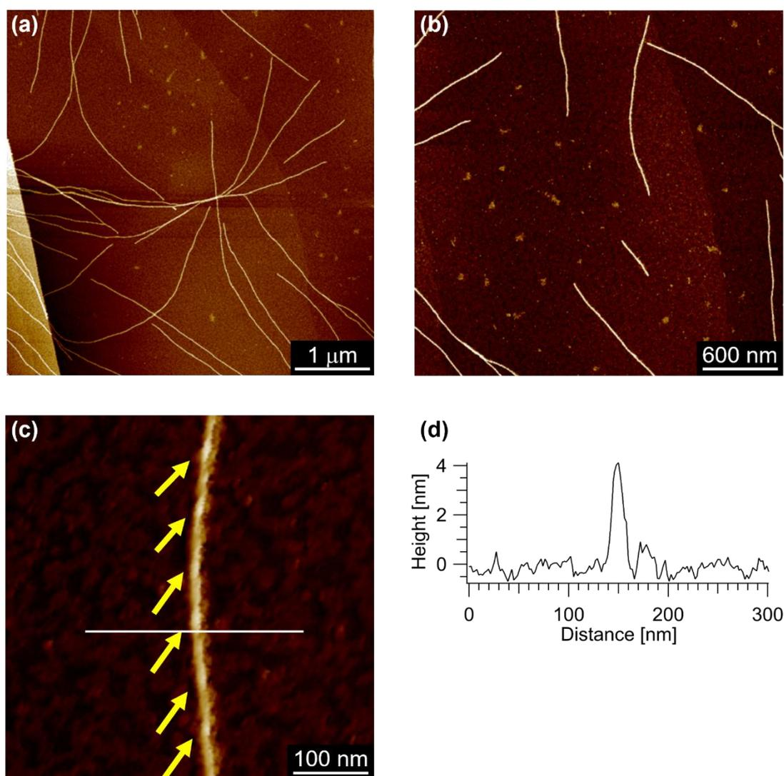
**Figure S9.** (a–c) AFM images of nanofibers of **Por<sub>d</sub>** formed in MCH ( $c = 100 \mu\text{M}$ ). The yellow arrows in (c) show the helicity of a nanofiber. (d) Cross-sectional analysis of a nanofiber of **Por<sub>d</sub>** along the white line in (c).
