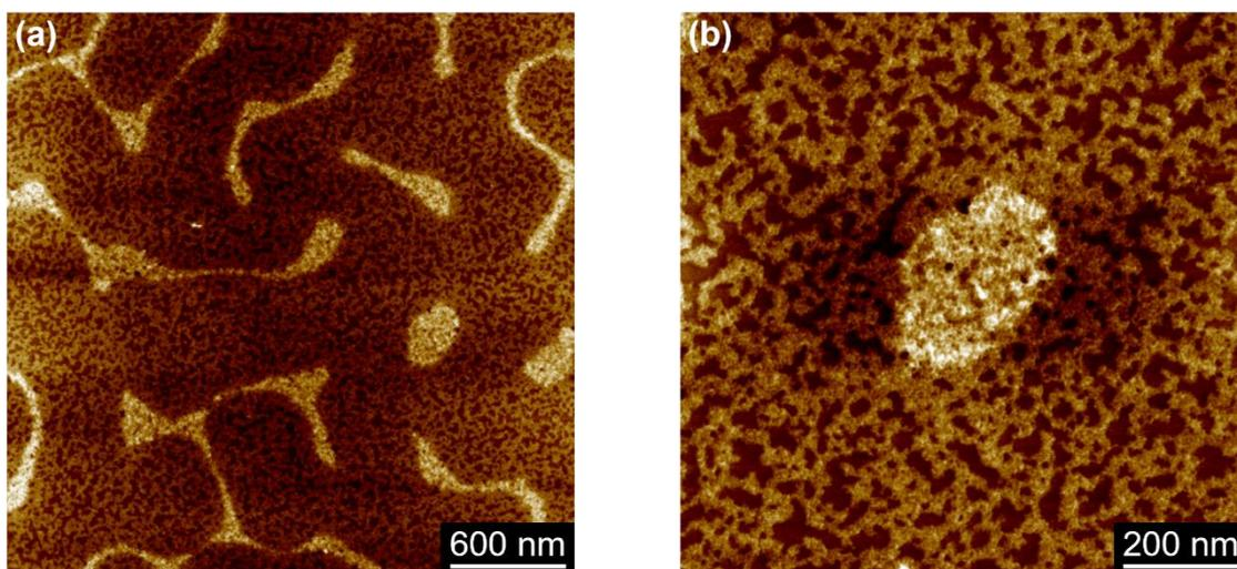
**Figure S8.** (a,b) AFM images of ill-defined agglomerates of **Por<sub>m</sub>** formed in MCH ( $c = 200 \mu\text{M}$ ).
