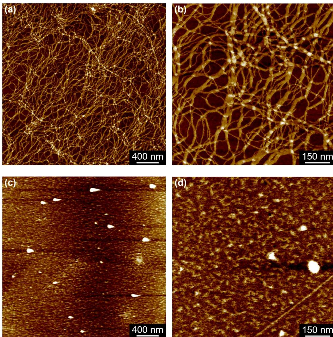
**Figure S4.** (a,b) AFM images of helical nanofibers of **Chl<sub>a</sub>** ( $c = 100 \mu\text{M}$ ) formed in MCH. (c,d) AFM images of ill-defined agglomerates of **Chl<sub>m</sub>** ( $c = 300 \mu\text{M}$ ) formed in MCH.
