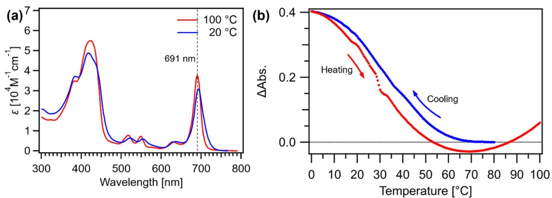
**Figure S3.** (a) UV/Vis absorption spectra of  $\text{Chl}_m$  at 100 and 20 °C during cooling a solution ( $c = 300 \mu\text{M}$ ) in MCH from 100 to 20 °C at a rate of  $1 \text{ }^\circ\text{C min}^{-1}$ . (b) Cooling (blue) and heating (red) curves of  $\text{Chl}_m$  obtained by plotting change in the absorption at 691 nm as a function of temperature.
