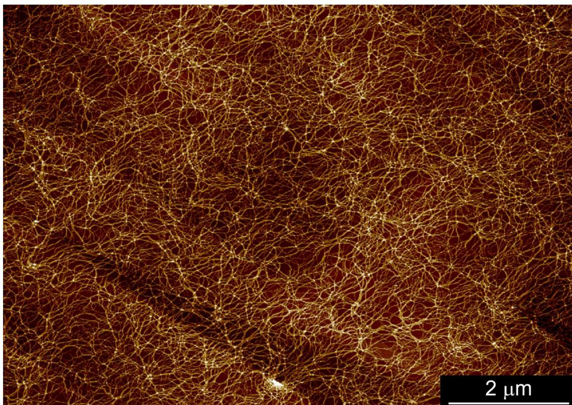
**Figure S5.** Wide-range AFM image of nanofibers of **Chl<sub>a</sub>** formed in MCH ( $c = 100 \mu\text{M}$ ) at  $20 \text{ }^\circ\text{C}$ .
