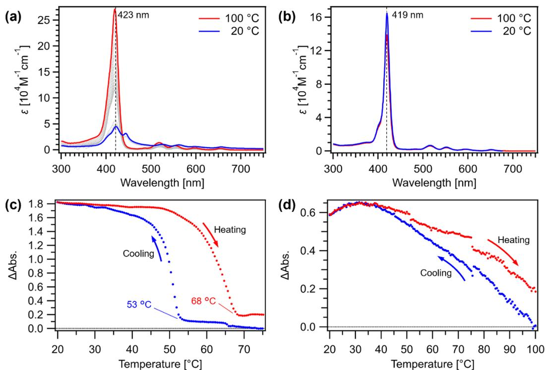
**Figure S7.** (a,b) UV/Vis absorption spectra of **Por<sub>d</sub>** (a) and **Por<sub>m</sub>** (b) during cooling their corresponding solutions in MCH from 100 (red) to 20 °C (blue) at a rate of  $1 \text{ }^\circ\text{C min}^{-1}$  at  $c = 100$  and  $200 \text{ } \mu\text{M}$ , respectively. (c,d) Cooling (blue) and heating (red) curves of **Por<sub>d</sub>** (c) and **Por<sub>m</sub>** (d) obtained by plotting change in the absorption at 423 nm as a function of temperature.
