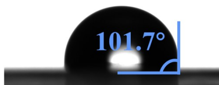
Fig. S3 Contact angle measurements of zinc metal with BE and NK electrolytes.
