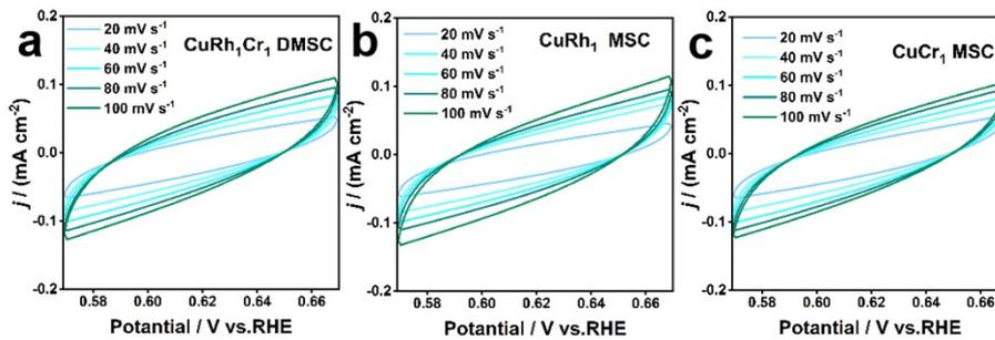
**Figure S8** CuRh<sub>1</sub>Cr<sub>1</sub> DMSC and comparison sample ECSA test.
