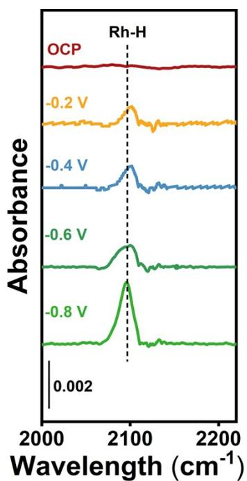
**Figure S9** In-situ infrared testing of CuRh<sub>1</sub> MSC at different reduction potentials.
