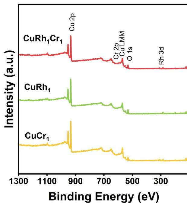
Figure S5 The full XPS spectra of CuRh<sub>1</sub>Cr<sub>1</sub> DMSC and the reference sample
