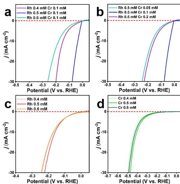
**Figure S7** CuRh<sub>1</sub>Cr<sub>1</sub> DMSC and comparison sample concentration gradient orthogonal experiment LSV test. a) b) CuRh<sub>1</sub>Cr<sub>1</sub> DMSC, c) CuRh<sub>1</sub> MSC, d) CuCr<sub>1</sub> MSC.
