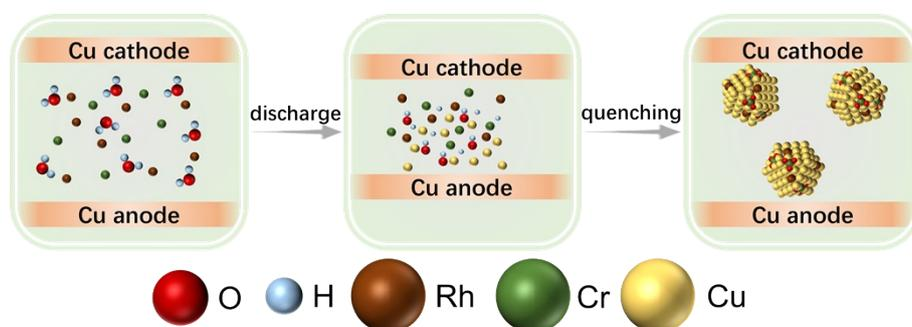
**Figure S1** Schematic illustration of the synthetic procedure for  $\text{CuRh}_1\text{Cr}_1$  DMSC.
