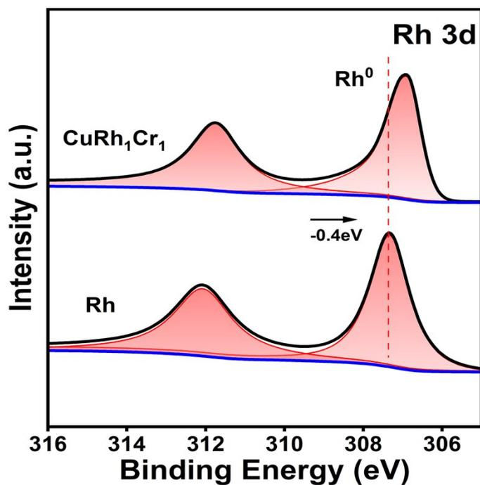
**Figure S6** Rh 3d XPS spectra of CuRh<sub>1</sub> MSC and Metallic Rh
