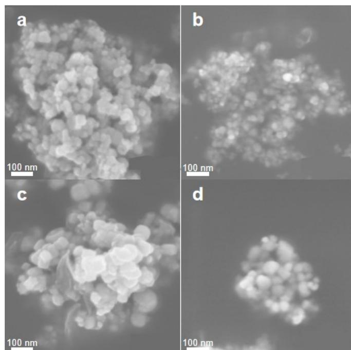
**Figure S2** SEM images of  $\text{CuRh}_1\text{Cr}_1$  DMSC and comparative samples. a)  $\text{CuRh}_1\text{Cr}_1$  DMSC. b)  $\text{CuRh}_1$  MSC. c)  $\text{CuCr}_1$  MSC. d) Cu.
