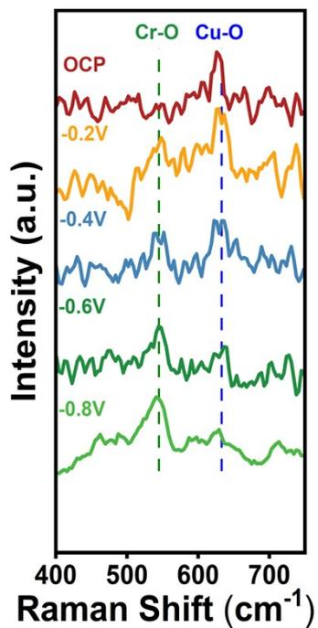
Figure S11 In-situ Raman testing of CuCr<sub>1</sub> MSC at different reduction potentials.
