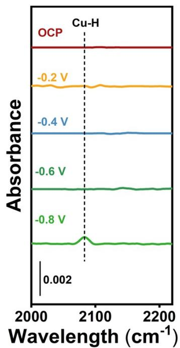
Figure S10 In-situ infrared testing of CuCr<sub>1</sub> MSC at different reduction potentials.
