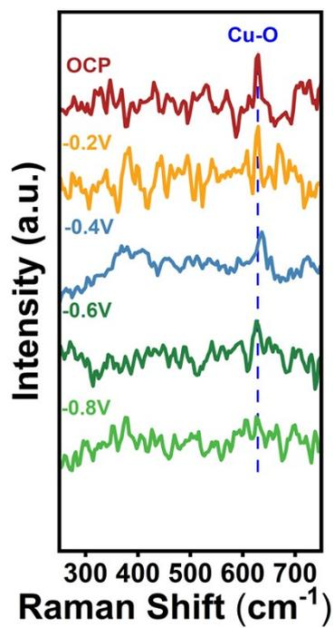
**Figure S12** In-situ Raman testing of CuRh<sub>1</sub> MSC at different reduction potentials.
