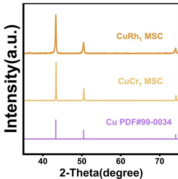
Figure S4 XRD patterns of CuRh<sub>1</sub> MSC and CuCr<sub>1</sub> MSC.
