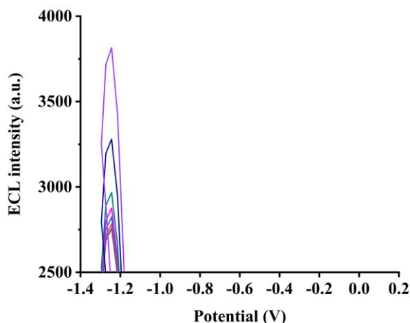
**Fig. S10.** The enlarged ECL-potential curves under varying target DNA concentrations.
