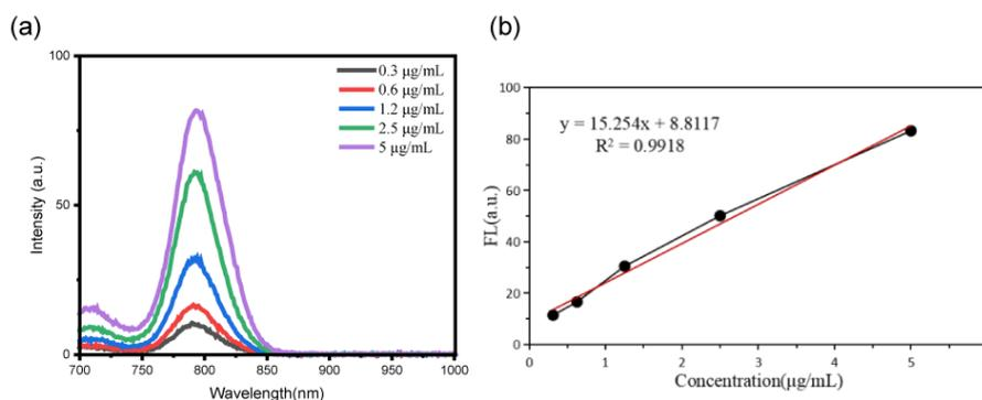
**Fig. S3** The fluorescence of compound C-6 at different concentrations and the standard curves.
