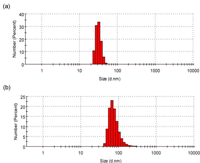
**Fig. S1** (a) Diameter of UCNPs measured by DLS. (b) Diameter of UCNPs@SiO<sub>2</sub> measured by DLS.
