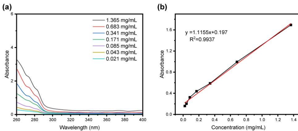
**Fig. S4** The absorbance of compound E-4 at different concentrations and the standard curves.
