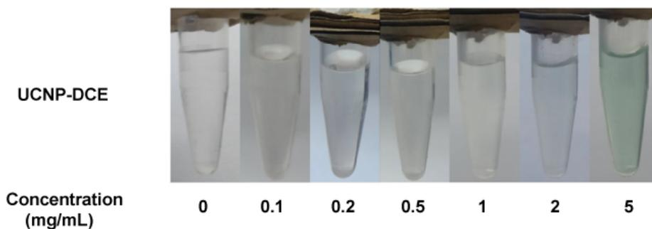
**Fig. S2** UCNPs-DCE at different concentrations in DMF.
