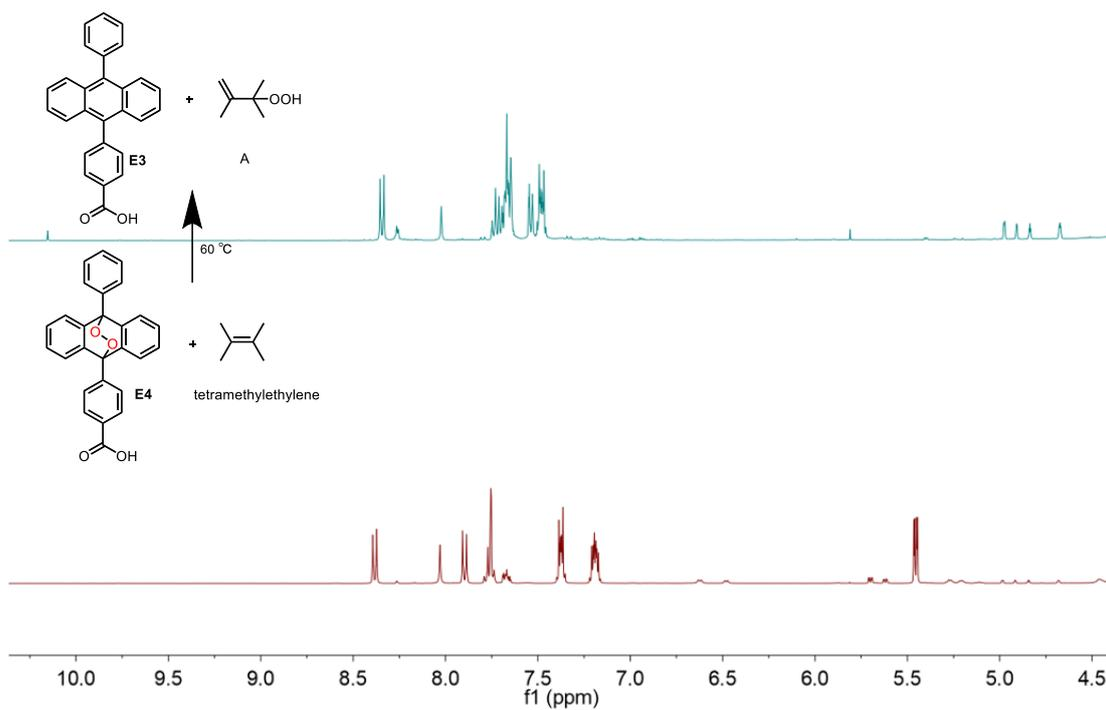
**Fig. S12** Singlet oxygen trapping using tetramethylethylene (1-1 ratio to anthracene endoperoxide).
