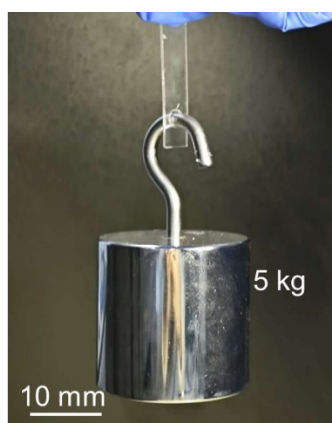
Figure S2. The prepared PMM-0.3-6 eutectogel (with a thickness of 1 mm) withstands the tensile force of a 5 kg weight.
