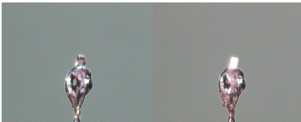
Figure S5 Single crystal of ZnCB-1 at 300 K (left) and 380 K (right) after attempted desolvation, with the latter showing loss of translucency and monocrystallinity.
