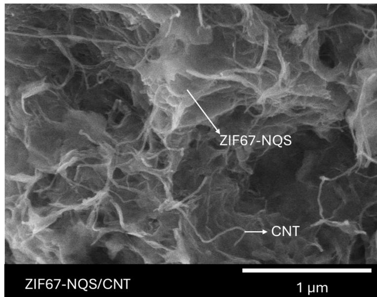
**Fig. S2.** SEM image of ZIF67-NQS/CNT
