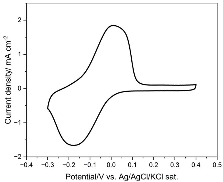
**Fig. S1.** Voltammogram of ZIF67-NQS/CNT in 0.1 M PBS pH 7
