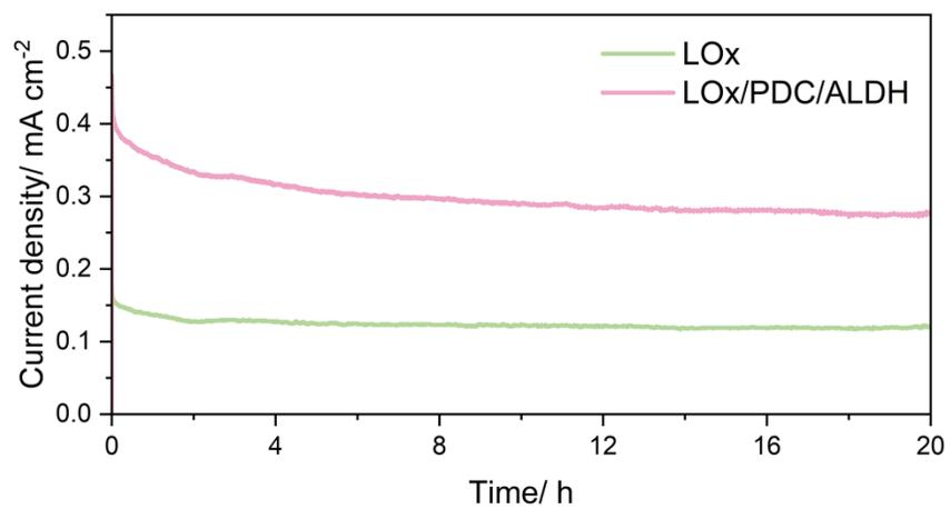
**Fig. S10.** Continuous operational stability of the multi-enzyme cascade electrode on the ZIF67-NQS/CNT platform over 20 h in 12 mM lactate in 0.1 M PBS at constant applied potential of 0.3V.
