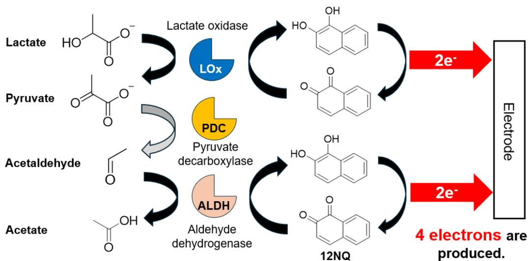
**Fig. S8.** Schematic illustration of electron production in mediated electron transfer reaction of cascade
