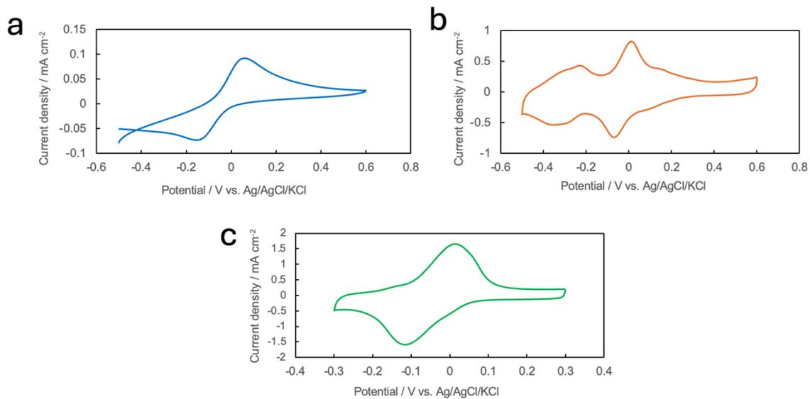
**Fig. S5.** Cyclic voltammetry (CV) in 0.1 M PBS (10 mV/s of scan rates) of a) GCE/NQ, b) CNT-COOH/NQ, and c) ZIF67-NQS/CNT; represents the higher redox active surface coverage of ZIF67-NQS/CNT compared to GCE/NQ and CNT-COOH/NQ.
