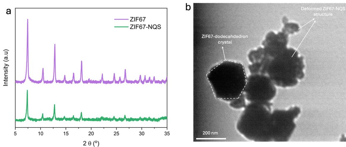
**Fig. S3.** a) Powder X-ray diffraction (PXRD) patterns of ZIF-67 and ZIF67-NQS, showing the reduction in crystallinity upon NQS integration; b) TEM image illustrating the well-defined rhombic dodecahedral crystals of ZIF67 and the deformed, irregular structure of ZIF67-NQS.
