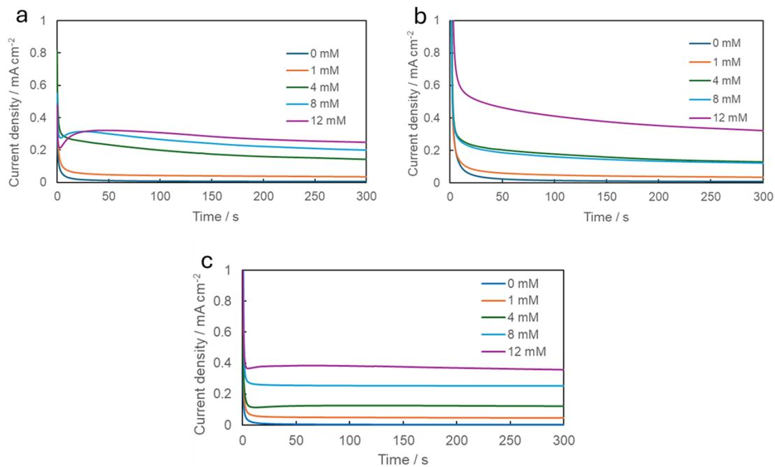
**Fig. S7.** Cascade enzyme electrode (LOx/PDC/ALDH) current response and stability towards the addition of lactate modified on; a) GC/NQ, b) CNT-COOH/NQ, and c) ZIF67-NQS/CNT. Measurements were conducted at 0.3V in 0.1M PBS.
