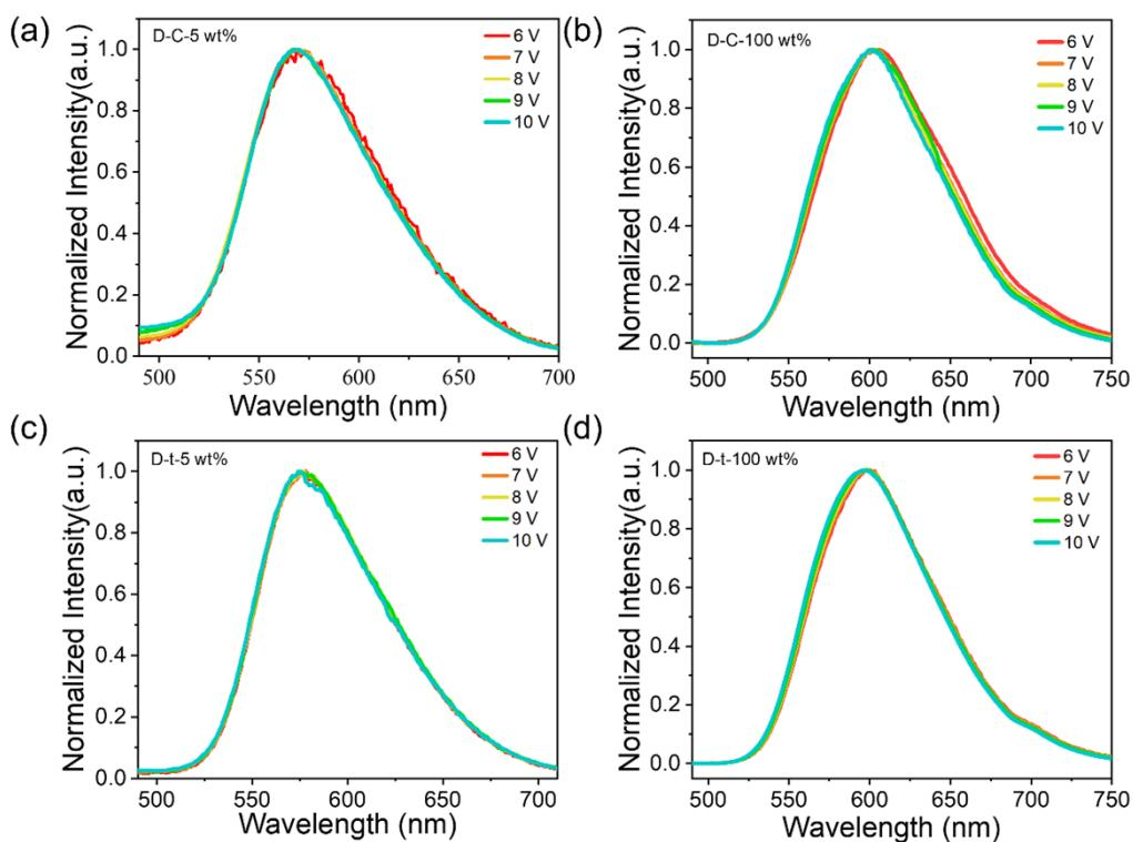
**Fig. S33** EL spectra of (a) D-C-5 wt%, (b) D-C-100 wt%, (c) D-t-5wt%, (d) D-t-100 wt% taken at various voltages from 6 to 10 V.
