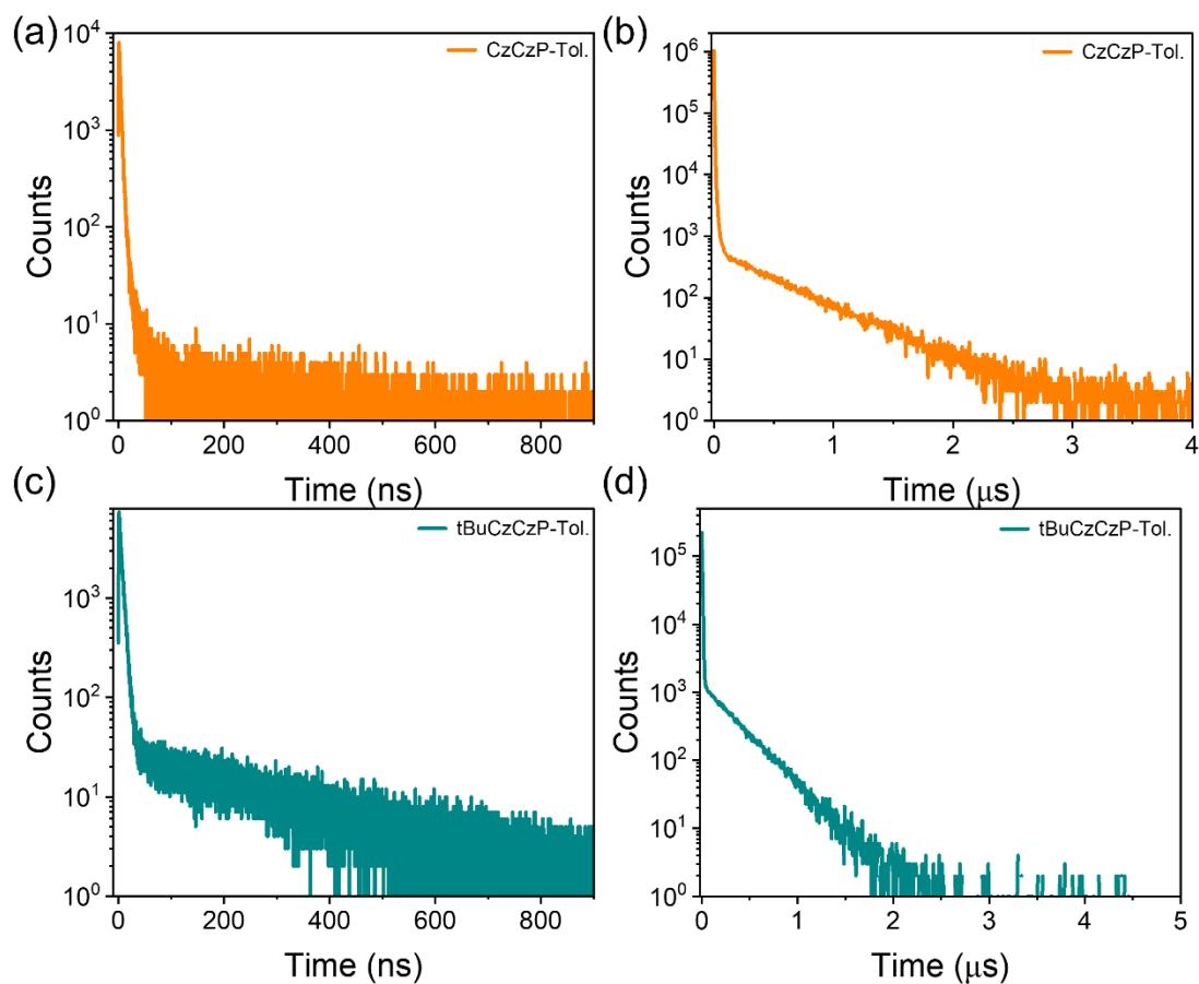
**Fig. S25** Transient photoluminescence decay curves of CzCzP and tBuCzCzP in toluene; a) and c) prompt fluorescence (PF) decay curves at nanosecond scale, c) and d) delayed fluorescence (DF) curves at microsecond scale.
