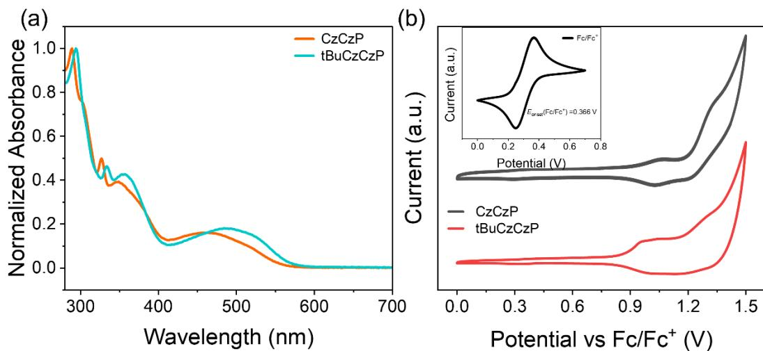
**Fig. S17** (a) The UV–vis absorption spectra of CzCzP and tBuCzCzP in CH<sub>3</sub>CN (r.t) (b) Cyclic voltammetry curves of CzCzP and tBuCzCzP, measured in CH<sub>3</sub>CN containing 0.1 M *tetra-n*-butylammonium hexafluorophosphate. Inset: Cyclic voltammetry diagram ferrocene as the internal standard, and the  $E_{(Fc/Fc^+)}$  is measured as 0.366 eV.
