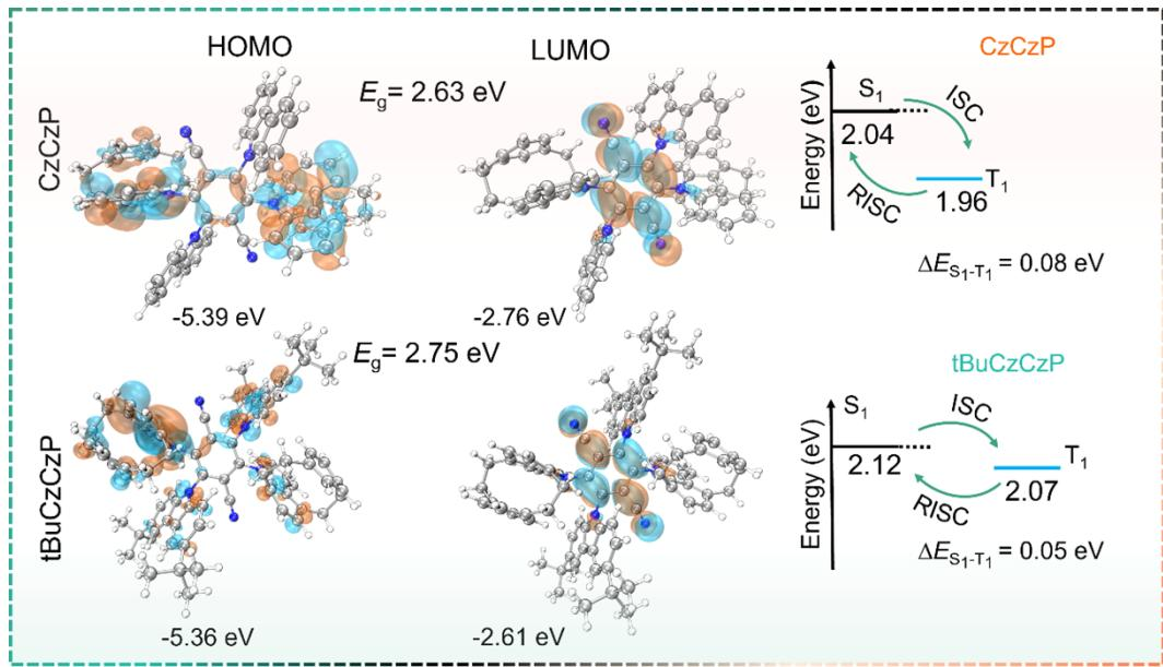
**Fig. S21** Ground-state optimized HOMO/LUMO distributions, energy level alignments ( $\Delta E_{ST}$ ) for CzCzP and tBuCzCzP.
