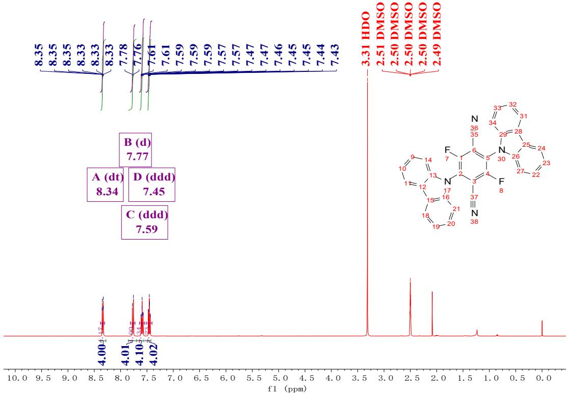
**Fig. S1** The  $^1\text{H}$  NMR spectrum of 2F-Cz in  $\text{DMSO}-d_6$  (400 MHz, 298 K).
