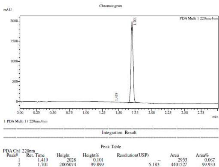
**Fig. S15** HPLC profile of R-CzP.
