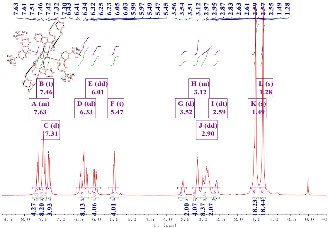
**Fig. S10** The  $^1\text{H}$ NMR spectrum of tBuCzCzP in  $\text{CDCl}_3$  (400 MHz, 298 K).
