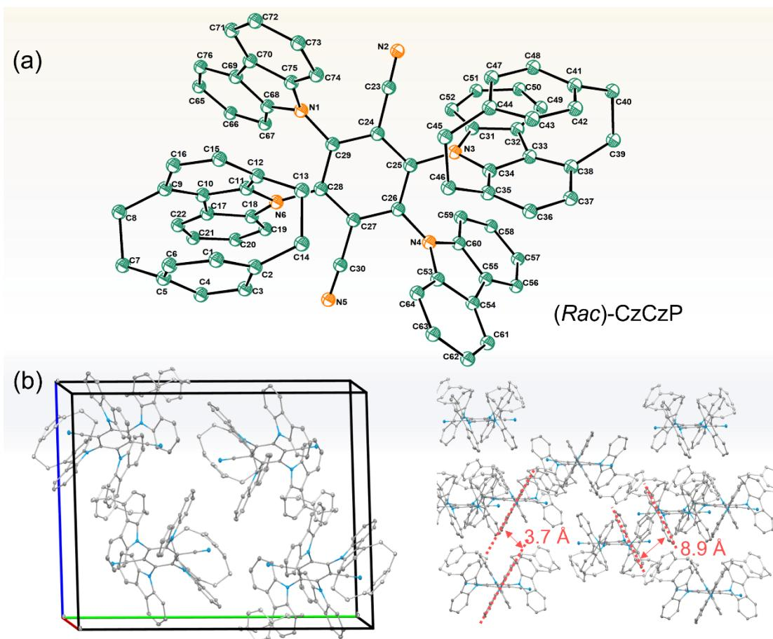
**Fig. S19** (a) Representative ORTEP-style diagram<sup>8</sup> and (b) packing diagram of compound (Rac)-CzCzP. Thermal ellipsoids are set at 20% probability level. All the hydrogen atoms and solvents are omitted for clarity.
