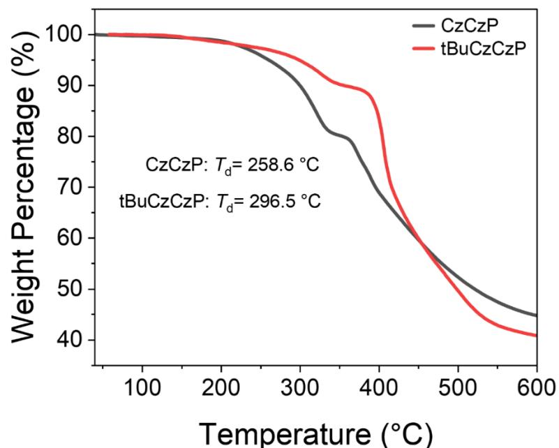
**Fig. S16** TGA curves of the two CP-TADF materials.
