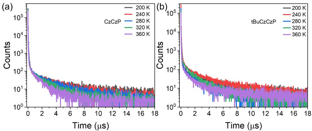
**Fig. S26** Temperature dependent transient PL decay curves of the doped films of a) CzCzP and b) tBuCzCzP
