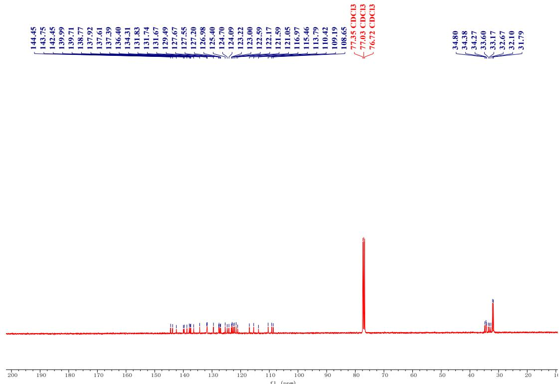
**Fig. S11** The  $^{13}\text{C}$ NMR spectrum of tBuCzCzP in  $\text{CDCl}_3$  (101 MHz, 298 K).
