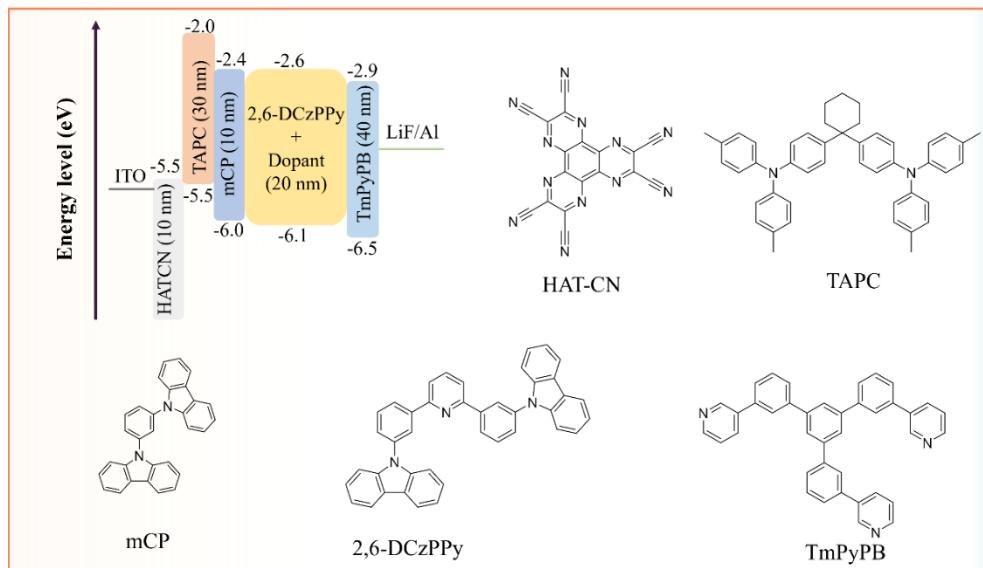
**Fig. S32** Multilayer device architecture with energy level alignment and chemical structures of key materials.
