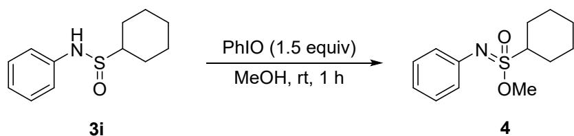
To a solution of **3i** (110 mg, 0.49 mmol) in anhydrous methanol (5 mL) was added iodosylbenzene (163 mg, 0.74 mmol) at room temperature. The reaction mixture was stirred for 1 h. After the starting materials consumed, the solvent was concentrated in vacuo and the residue was purified by a column chromatography (petroleum ether/ethyl acetate = 50:1 to 40:1), delivering the corresponding product **4** (98 mg, 78%) as a colorless oil.<sup>1</sup>
