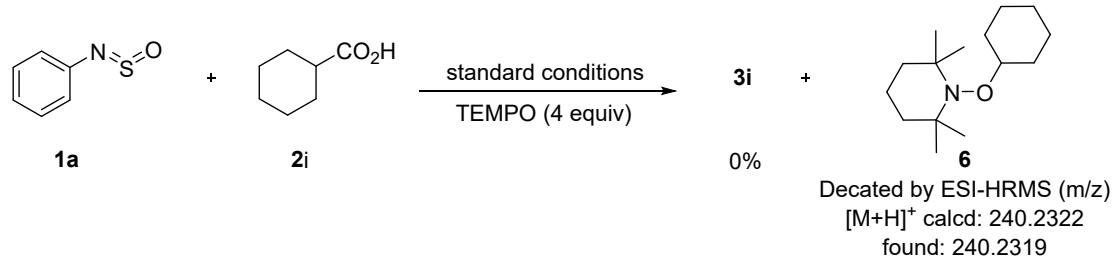
To an 8 mL vial equipped with a magnetic stir bar was added **1a** (28 mg, 0.2 mmol), carboxylic acids **2i** (38.4 mg, 0.3 mmol), FeCl<sub>3</sub> (0.02 mmol), TEMPO (124.8 mg, 0.8 mmol),
