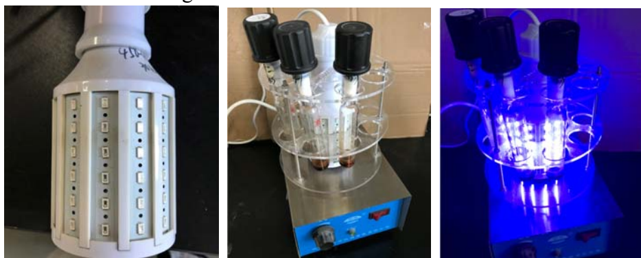
Figure S1. Photoreactor used in this work (30 W blue LEDs, \lambda_{\text{max}} = 454 nm).
