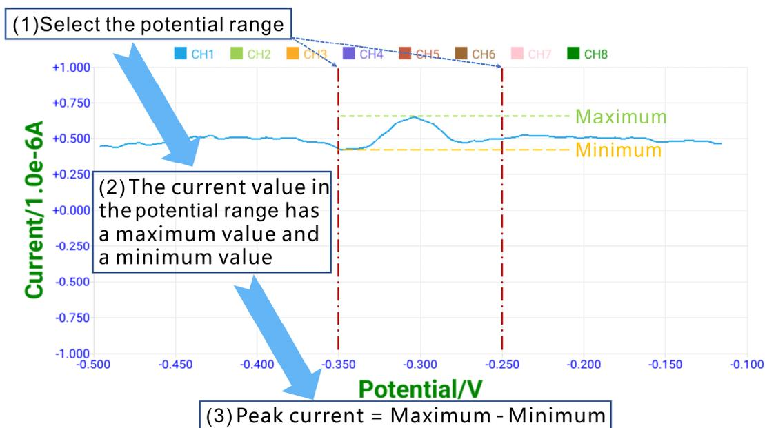
Fig. S5 Schematic diagram of the current peak algorithm built into the SDEA.
