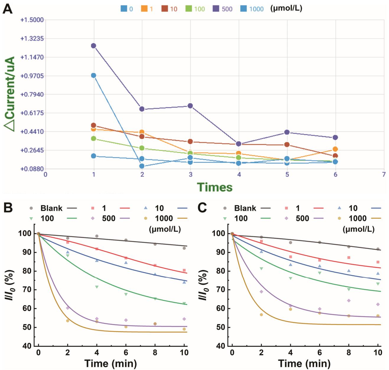
Fig. S6 (A) The screenshot of the SDEA illustrates the real-time data processed by its built-in peak current algorithm, with the horizontal axis representing the number of scans and the vertical axis indicating the peak current value. (B) Results of manual processing for parallel experiment group 2. (C) Results of manual processing for parallel experiment group 3.
