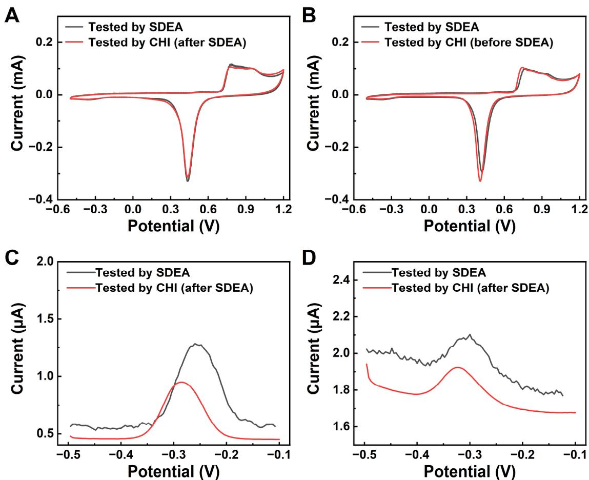
Fig. S4 (A) For the same bare CGE, the SDEA scans first, and the CHI scans later. (B) For the same bare CGE, the CHI scans first, and the SDEA scans subsequently. (C) For the same modified CGE, the SDEA scans first, followed by the CHI. (D) For the same modified CGE, the CHI scans first, and the SDEA scans later.
