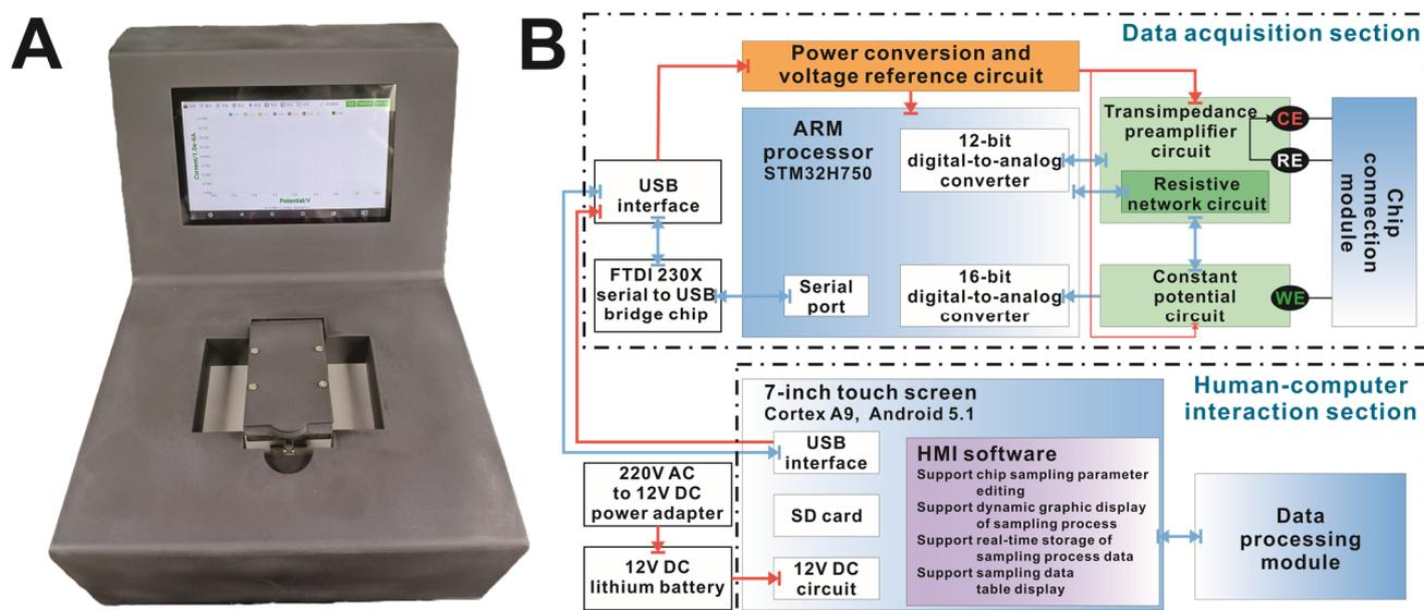
Fig. S3 (A) The appearance of the self-developed electrochemical analyzer (SDEA). (B) A thumbnail representation of the system architecture of SDEA.
