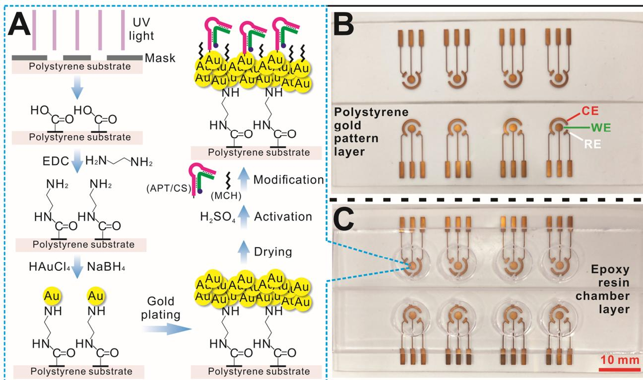
Fig. S2 (A) Schematic diagram of CGE and sensor manufacturing process. (B) Diagram of the eight-channel CGE. (C) An eight-channel CGE chip.
