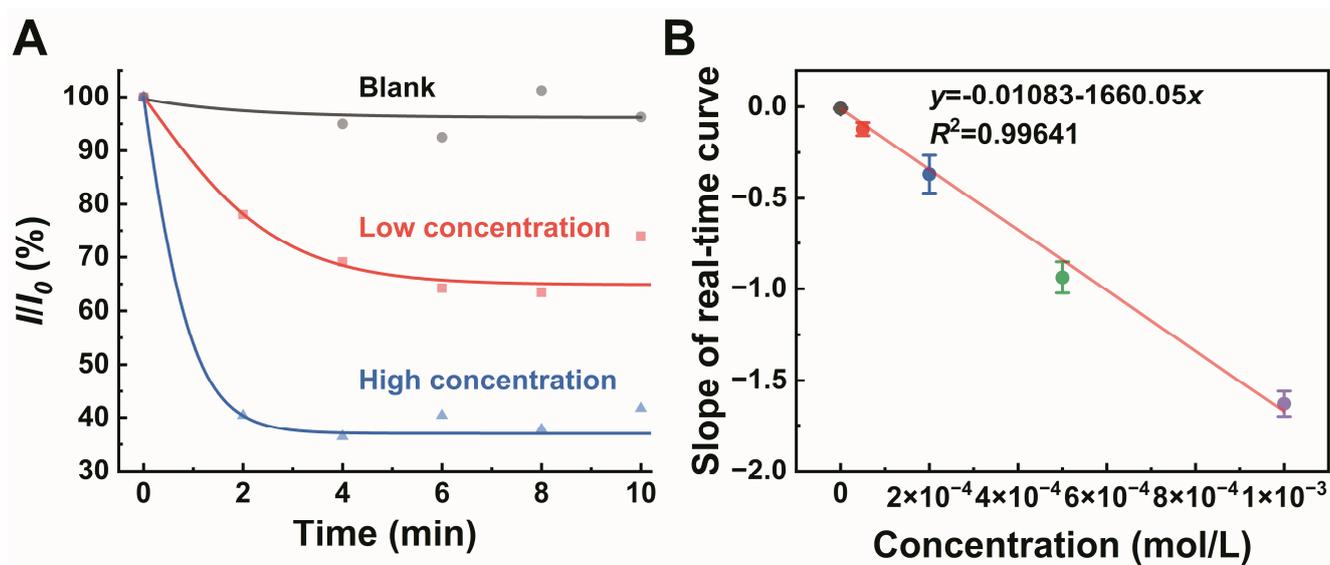
Fig. S7 (A) Real-time results of tetracycline detection. (B) The variation trend of initial point slope in real-time data fitting curves with concentration and their corresponding fitting curve, error bar: SD, n=2-3.
