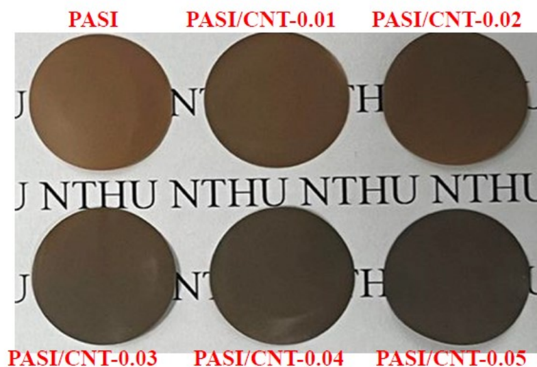
Figure S9. Photographs recorded on the prepared PASI/CNT-X nanocomposites, X denoting to the MWCNT-PASI contents in wt% of the nanocomposites.
