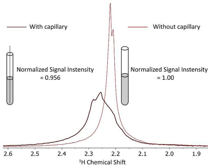
**Figure S3.** A 90-degree single  $^1\text{H}$  NMR scan of 0.91M acetonitrile ( $\text{CH}_3\text{CN}$ ) in chloroform ( $\text{CDCl}_3$ ), performed in a 5 mm NMR tube with and without a capillary tube.
