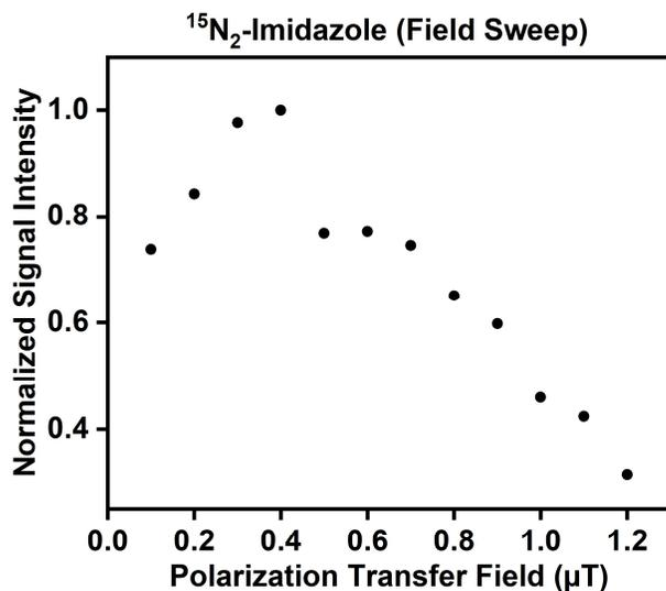
**Figure S6.** Polarization transfer field optimization study demonstrates that 0.4 μT is the optimal field for transferring polarization from  $p$ -H<sub>2</sub> to the <sup>15</sup>N nuclei of <sup>15</sup>N<sub>2</sub>-imidazole.
