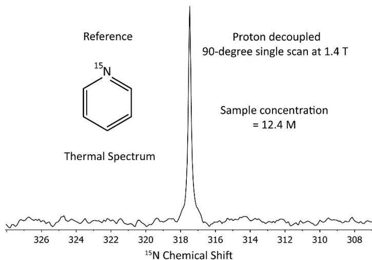
**Figure S2.** Proton-decoupled  $^{15}\text{N}$  NMR spectrum of a thermally polarized neat  $^{15}\text{N}$ -pyridine reference sample at 1.4 T.
