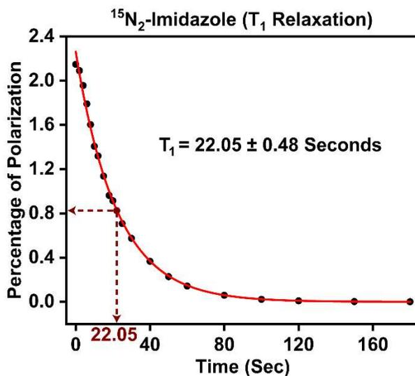
**Figure S8.** Relaxation study of the  $^{15}\text{N}$  nuclei of  $^{15}\text{N}_2$ -imidazole at 1.4 T magnetic field shows a  $T_1$  relaxation time of  $22.05 \pm 0.48$  seconds.
