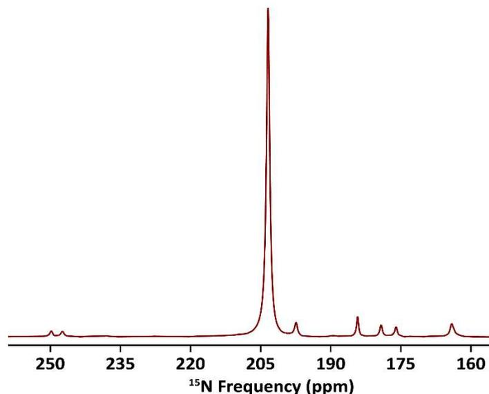
**Figure S1.** SABRE-SHEATH hyperpolarized proton-decoupled  $^{15}\text{N}$  NMR spectrum of  $^{15}\text{N}_2$ -imidazole acquired using a 1.4 T Magritek benchtop NMR spectrometer.
