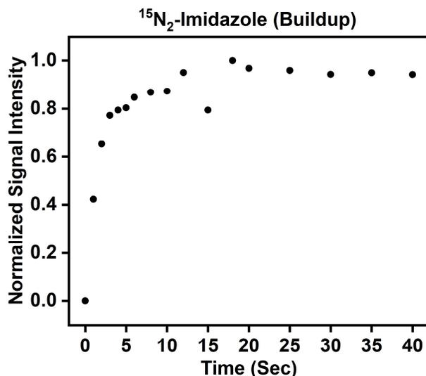
**Figure S5.** SABRE-SHEATH hyperpolarization build-up study of  $^{15}\text{N}_2$ -imidazole revealed polarization saturation after 25 seconds of bubbling with  $\approx 93\%$   $p\text{-H}_2$ .
