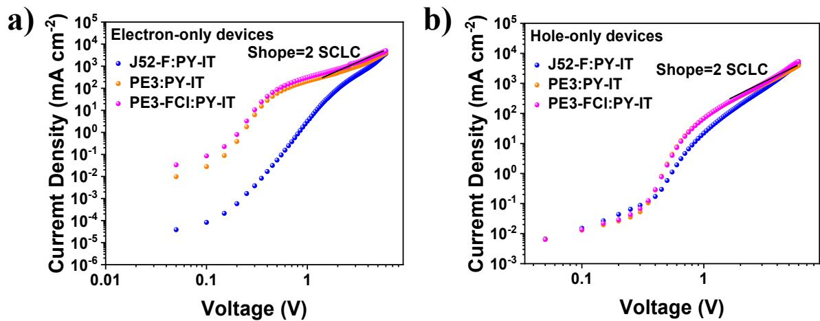
**Fig. S4** Electron and hole mobility of three polymer-based devices.
