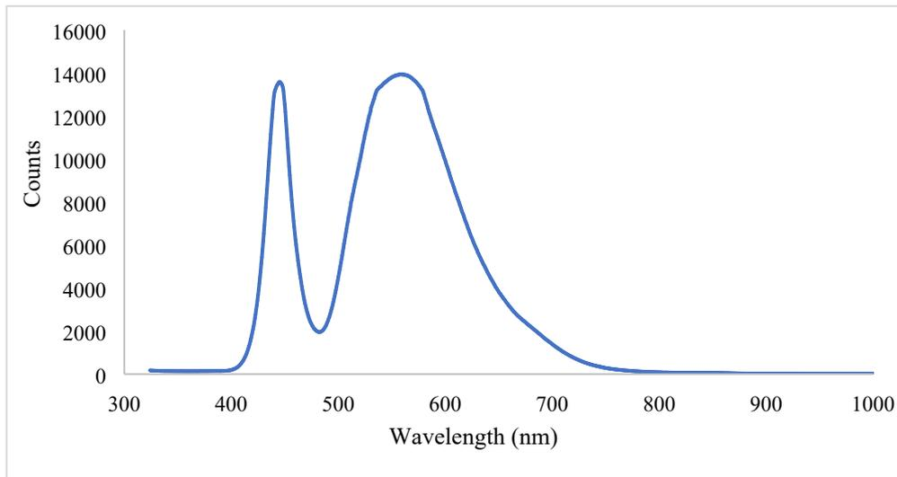
The blue LED (27 W) was purchased from Yihua Company. We measured the spectral profile of the blue LED light by ourselves (recorded on an AVANTES®AvaSpec-
