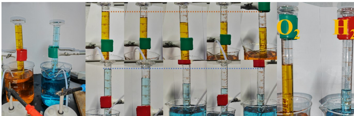
Fig. S9 Schematic of the Faradaic efficiency measurement setup for water splitting, along with photographs showing the collected H_2 and O_2 gases.
