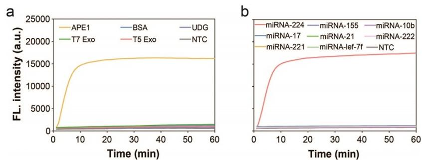
**Fig. S11** (a) Selectivity analysis of the platform to T7 Exo, T5 Exo, UDG (Uracil-DNA glycosylase), BSA (Bovine albumin), APE1. (b) Selectivity analysis of the platform to different miRNAs. APE1: 1 U/ $\mu$ L, miRNA-224: 1 nM. NTC: negative target control.
