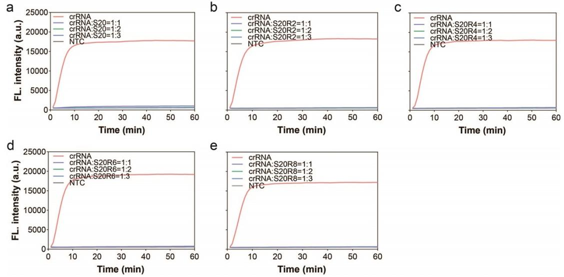
**Fig. S2** Fluorescence kinetic curves of crRNA and different DBs, including S20 (a), S20R2 (b), S20R4 (c), S20R6 (d), S20R8 (e) with concentration ratios of 1:1, 1:2, 1:3. RNA target: 1 nM, APE1: 1 U/ $\mu$ L. NTC: negative target control.
