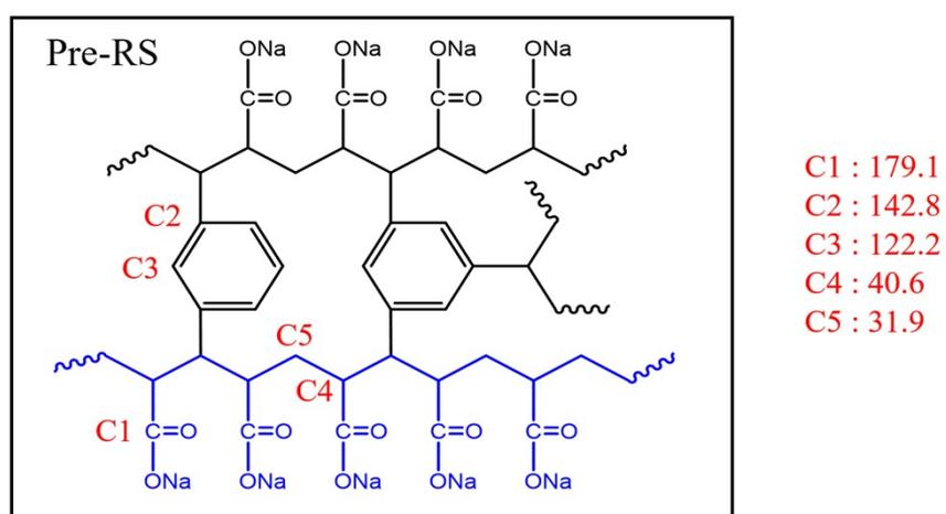
**Figure S6.** The structure of Pre-RS.
