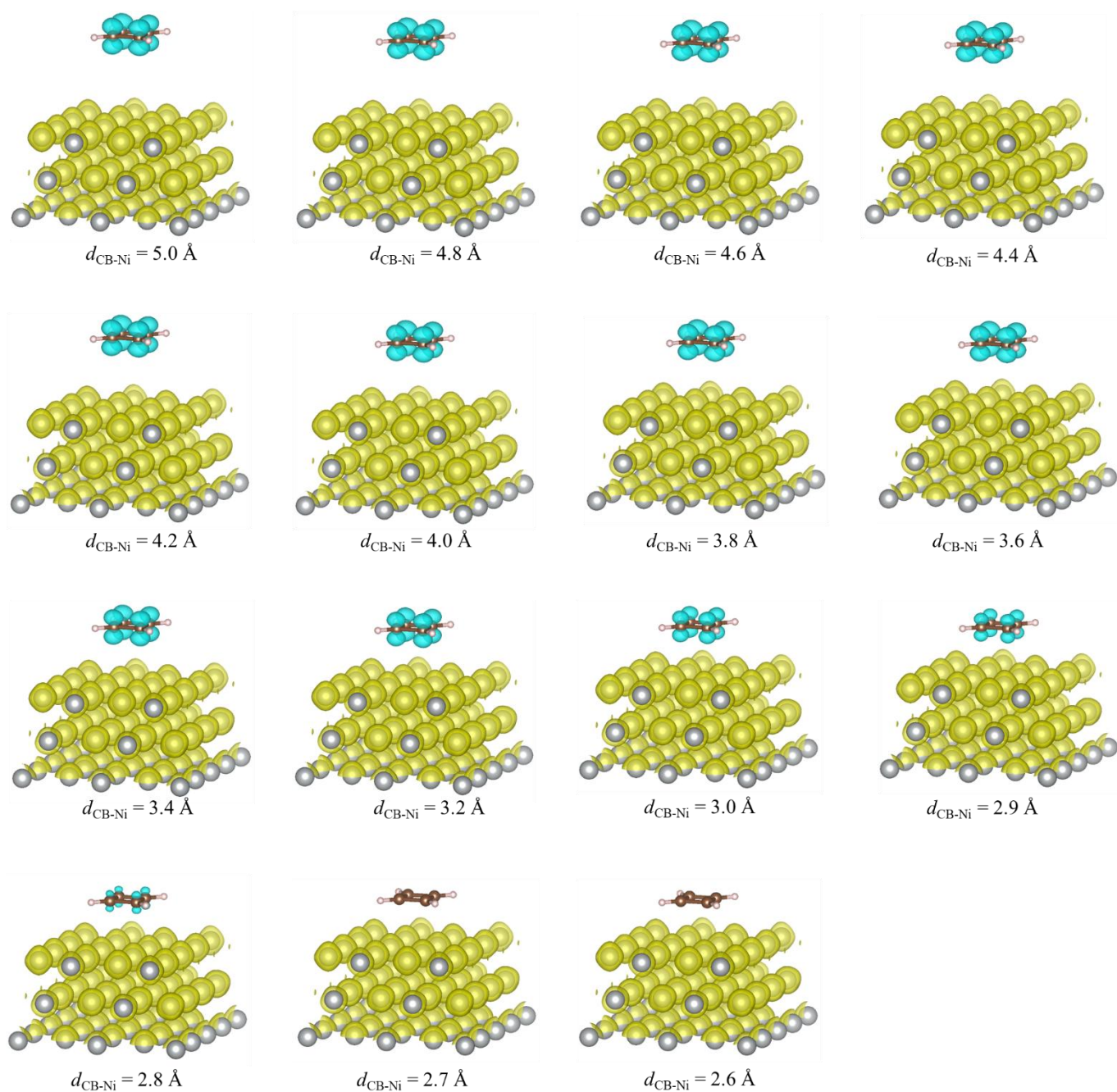
Figure S3. Spin-density distributions of triplet AP states. Yellow and blue represent the distributions for alpha and beta electrons, respectively. The threshold is 0.015 e - /Bohr 3 . In this structure, the electronic spins of the CB are delocalised to Ni(111), and the electronic states and energies of the d_{\text{CB-Ni}} = 2.6 Å structures shown in Figs. S1–S3 are difficult to distinguish at the DFT level. In addition, no significant spin distribution on the CB is observed at d_{\text{CB-Ni}} = 2.7 Å, which is due to the effect of self-interaction error in DFT.
