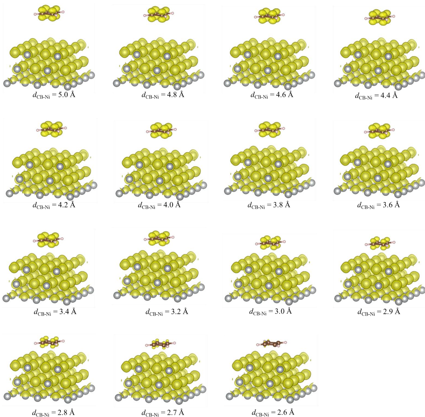
Figure S2. Spin-density distributions of triplet_P states. Yellow and blue represent the distributions for alpha and beta electrons, respectively. The threshold is 0.015 \text{ e}^-/\text{Bohr}^3 . In this structure, the electronic spins of the CB are delocalised to Ni(111), and the electronic states and energies of the d_{\text{CB-Ni}} = 2.6 \text{ \AA} structures shown in Figs. S1–S3 are difficult to distinguish at the DFT level.
