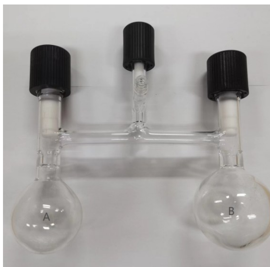
Figure S11 Glass apparatus used for N 2 reduction to NH 3 .
